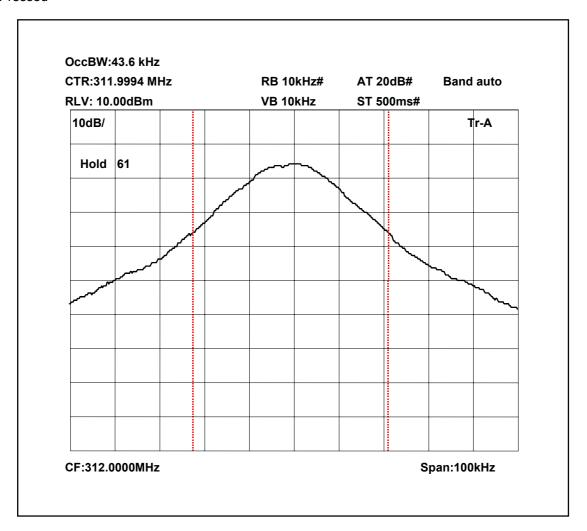
Occupied Bandwidth = 43.6kHz FI = 311.9780MHz Fh = 312.0216
