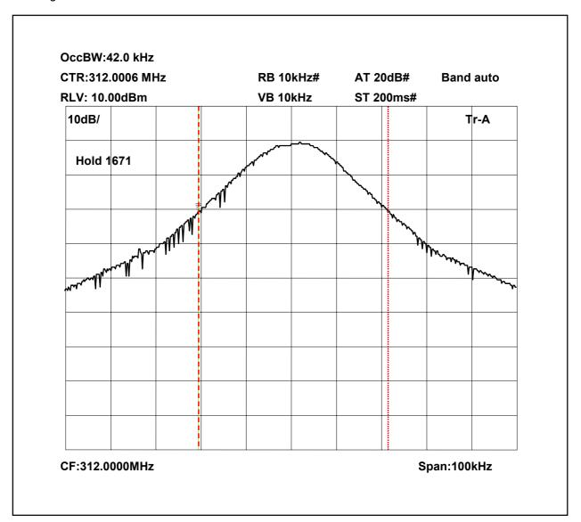
Occupied Bandwidth = 42kHz FI = 311.9796MHz Fh = 312.0216MHz
