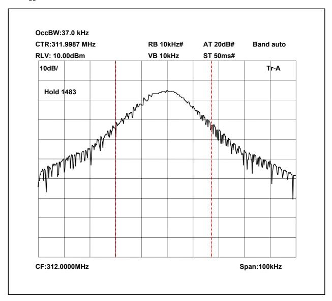
Occupied Bandwidth = 37kHz FI = 311.9802MHz Fh = 312.0172MHz
