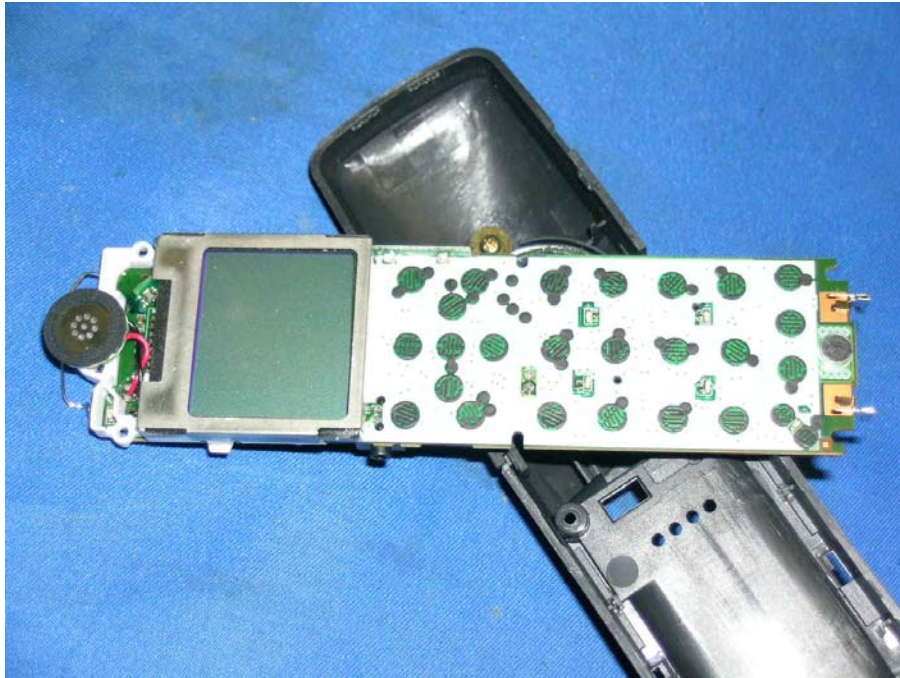
Handset Main PCB display side (View 1)
