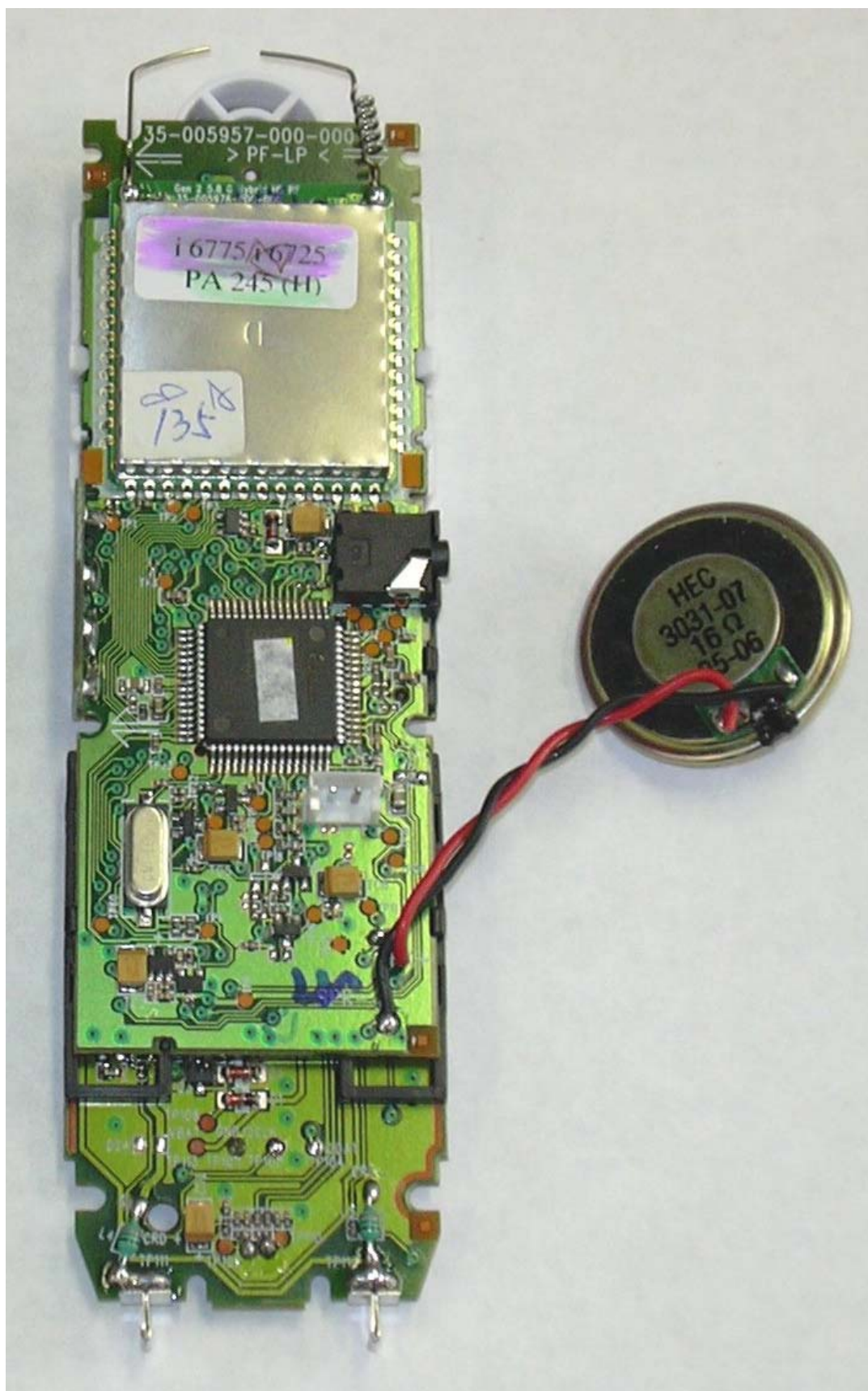
VTech I6765 Handset PCB
