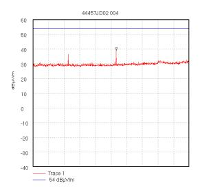
Start 2.0 GHz; Stop 4.0 GHz Ref 60 dBµV/m; Ref Offset 0.0 dB; 10 dB/div RBW 1000.0 kHz; VBW 1.0 MHz; Att 0 dB; Swp 20.0 mS Peak 3.067 GHz, 39.03 dBµV/m Display Line: 54 dBµV/m; ; Limit Test Passed 10/31/2003 3:36:29 PM
