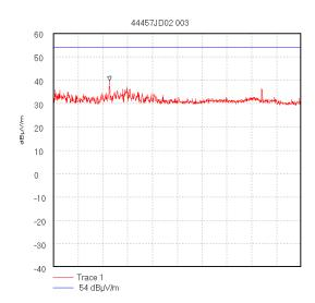
Start 1.0 GHz; Stop 2.0 GHz Ref 60 dBμV/m; Ref Offset 0.0 dB; 10 dB/div RBW 1000.0 kHz; VBW 1.0 MHz; Att 0 dB; Swp 20.0 mS Peak 1.228 GHz, 39.66 dBμV/m Display Line: 54 dBμV/m; ; Limit Test Passed 10/31/2003 3:18:23 PM
