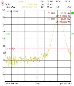
Comment A: Radiated Band Edge Bottom Channel WMTS Telepack
