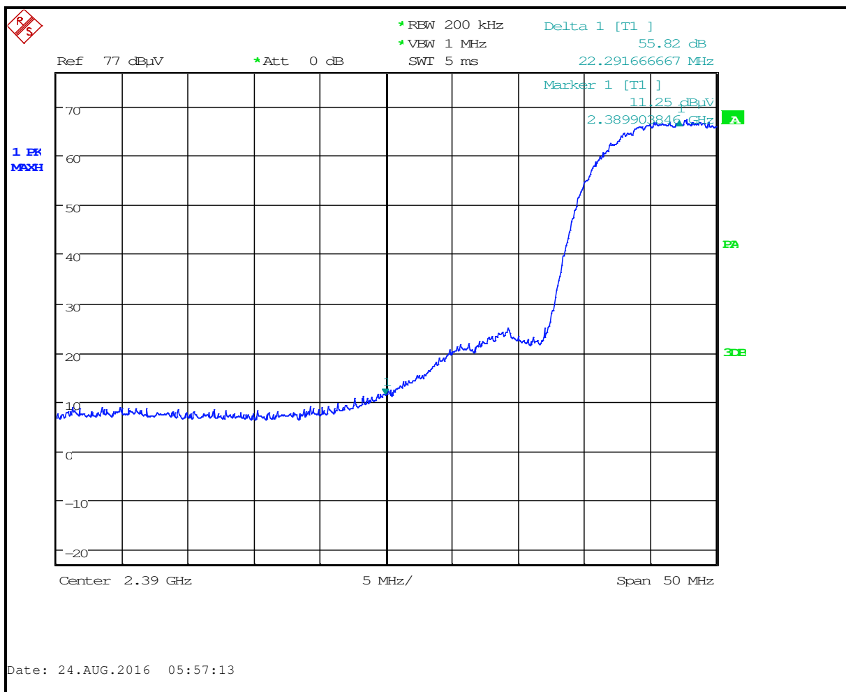
Plot 4-1: Lower Band Edge – 802.11b (Antenna #1)
