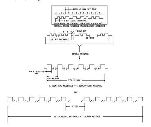
Rolling code encryption (14.3%) Messages, with the HCS 300 Encoder:
