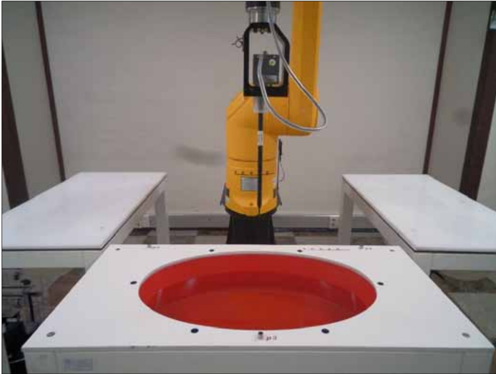
(a) SAR measurement system
