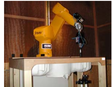
Figure 6.1 DASY3 Test System
