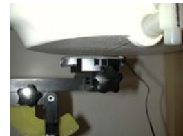
Figure 14.10 Body SAR Test Setup -- w/o Holster --
