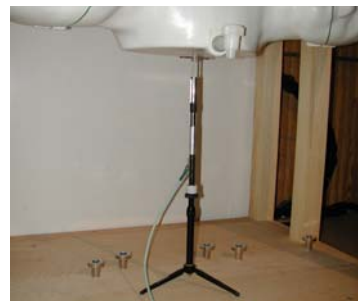
Figure 12.1 Dipole Validation Test Setup
