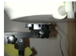
Figure 14.9 Body SAR Test Setup -- w/o Holster --
