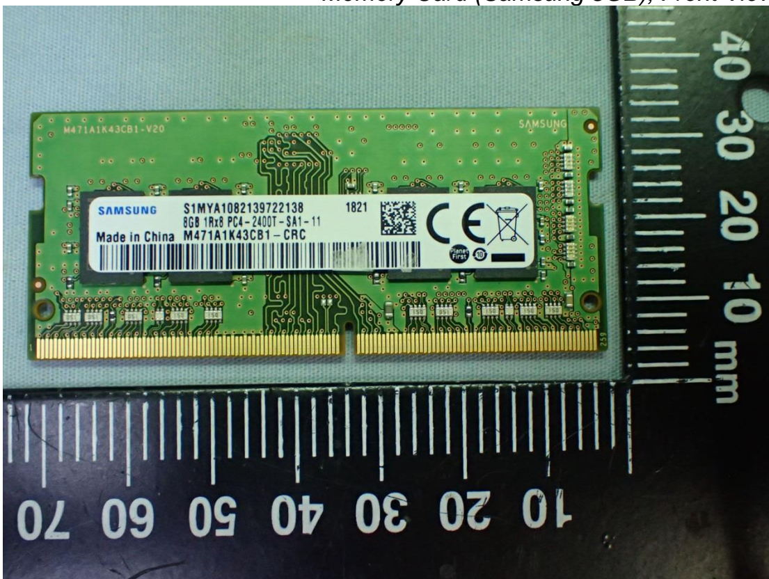
Figure 56 Memory Card (Samsung 8GB), Front View
