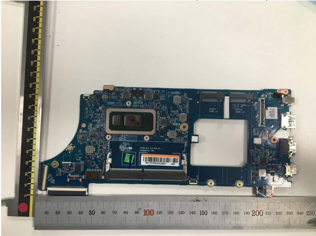
Figure 34 Main Board (with Thunderbolt), Front View
