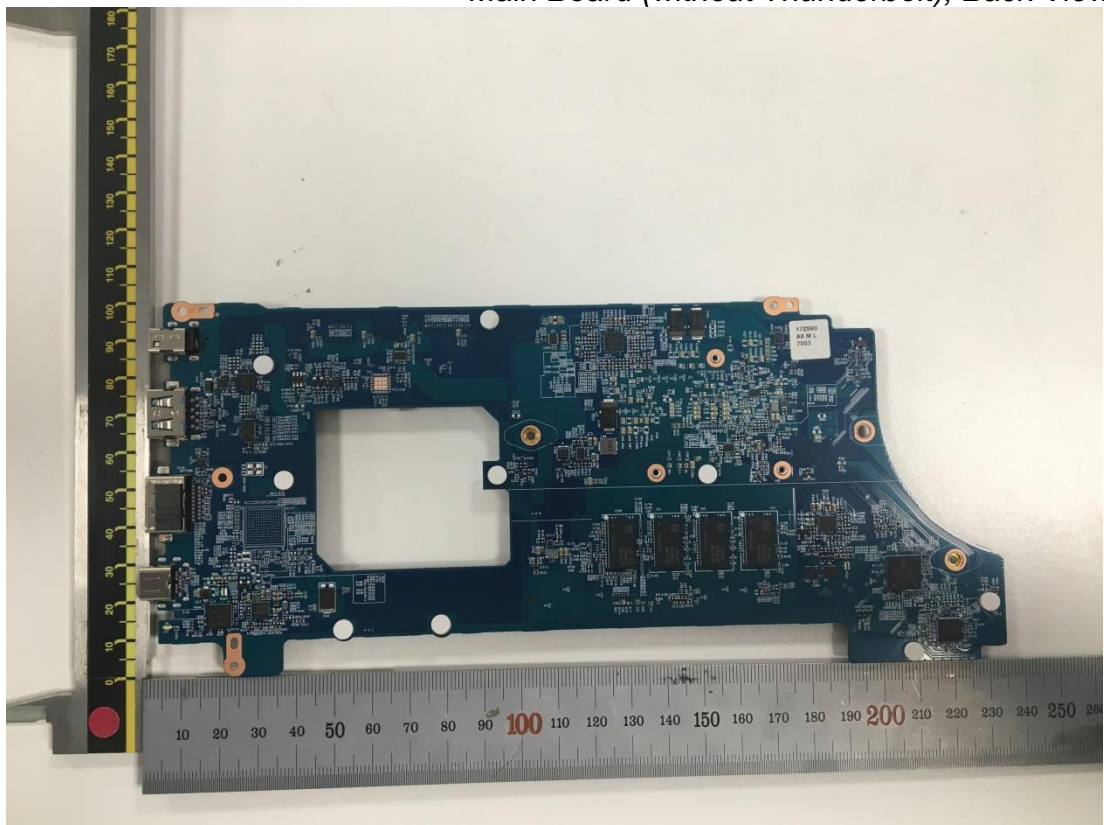
Figure 37 Main Board (without Thunderbolt), Back View
