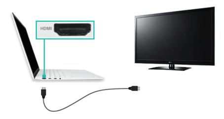
2 On the PC, press [Fn] + [F7] to display monitor (projector) toggling screen. Select the desired screen output.
