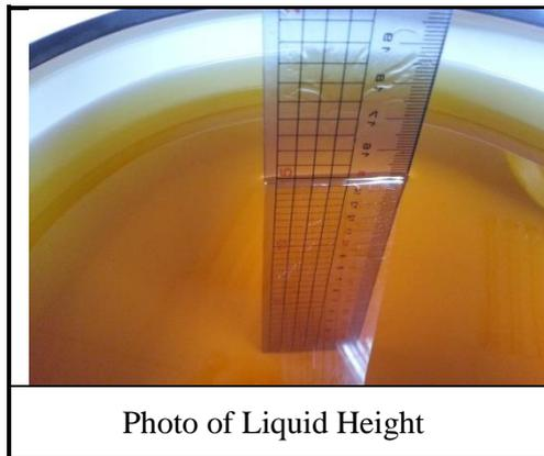
The dielectric properties of the head tissue simulating liquids are defined in IEEE 1528 and FCC OET 65 Supplement C Appendix C. For the body tissue simulating liquids, the dielectric properties are defined in FCC OET 65 Supplement C Appendix C. The dielectric properties of the tissue simulating liquids were verified prior to the SAR evaluation using an Agilent 85070D Dielectric Probe Kit and an Agilent Network Analyzer.
