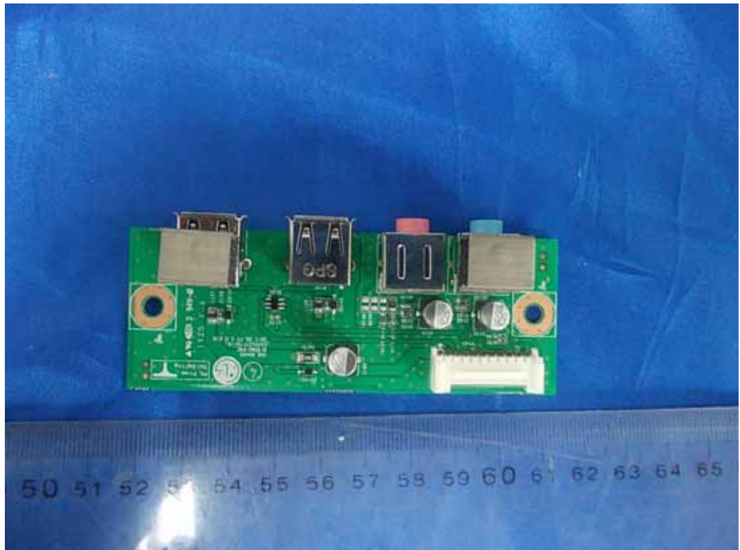
FIGURE 13 LCD MONITOR (M/N: N2311AZ) USB BOARD (COMPONENT SIDE)
