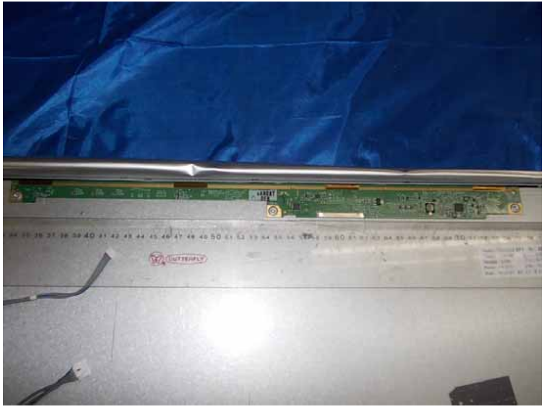
FIGURE 11 LCD MONITOR (M/N: N2311AZ) LCD PANEL BOARD (COMPONENT SIDE)
