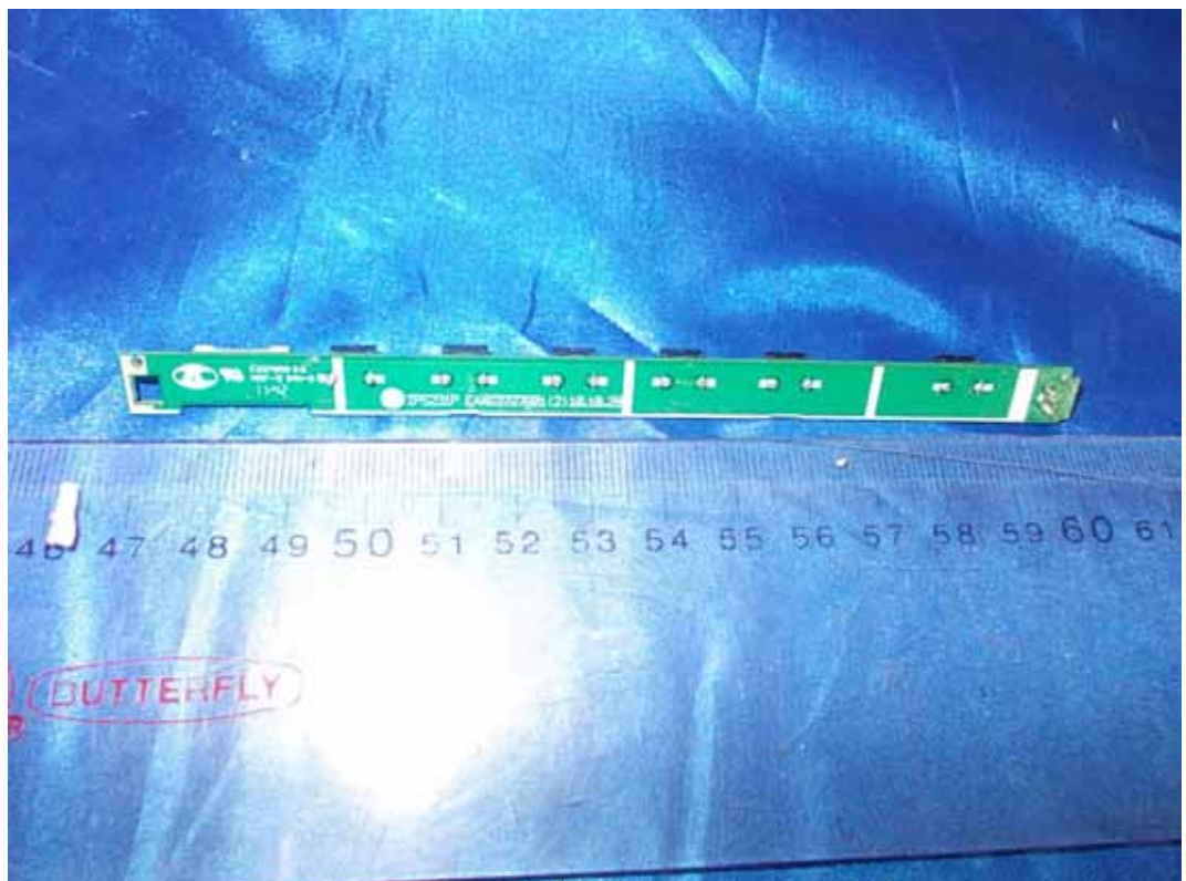
FIGURE 10 LCD MONITOR (M/N: N2311AZ) KEY BOARD (SOLDERED SIDE)
