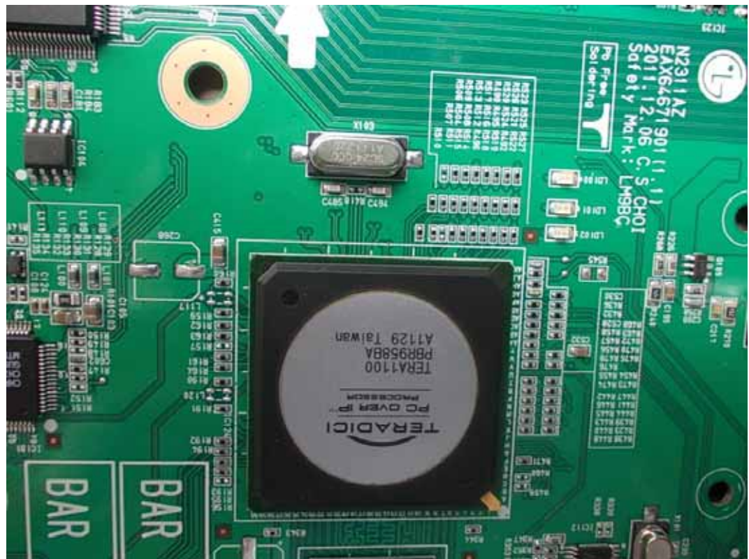
FIGURE 5 LCD MONITOR (M/N: N2311AZ) CHIP#1 & CRYSTAL#1 ON MAIN BOARD
