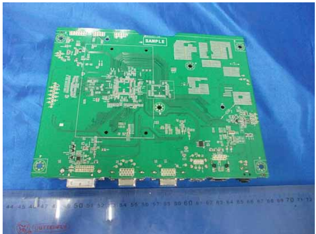
FIGURE 4 LCD MONITOR (M/N: N2311AZ) MAIN BOARD (SOLDERED SIDE)
