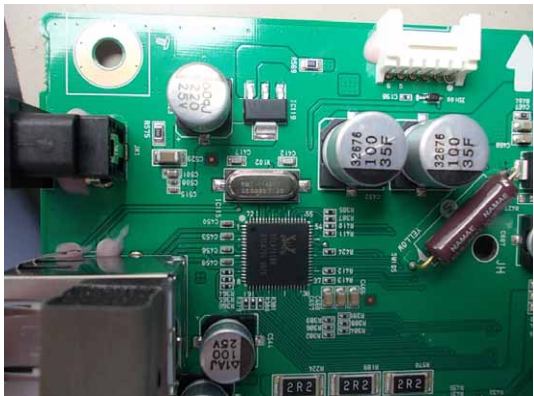
FIGURE 6 LCD MONITOR (M/N: N2311AZ) CHIP#2 & CRYSTAL#2 ON MAIN BOARD
