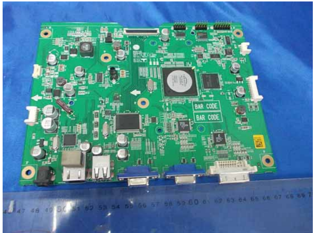
FIGURE 3 LCD MONITOR (M/N: N2311AZ) MAIN BOARD (COMPONENT SIDE)
