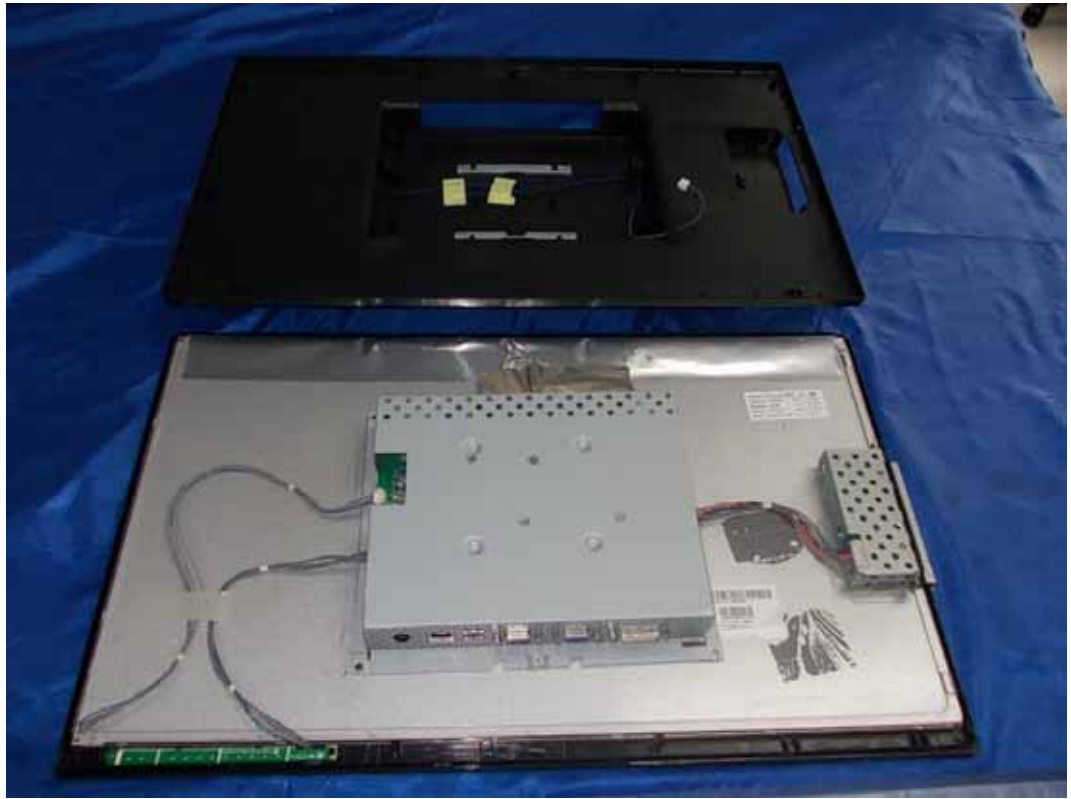
FIGURE 1 LCD MONITOR (M/N: N2311AZ) COVER REMOVED
