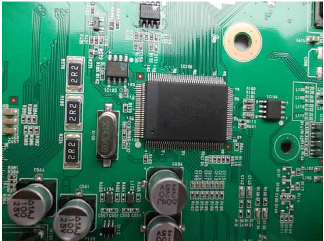
FIGURE 7 LCD MONITOR (M/N: N2311AZ) CRYSTAL#3 ON MAIN BOARD
