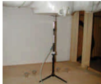
Figure 12.1 Dipole Validation Test Setup
