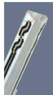
Figure 3.2 Probe Thick-Film Technique
