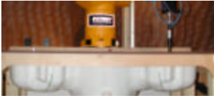
Figure 5.1 SAM Twin Phantom
