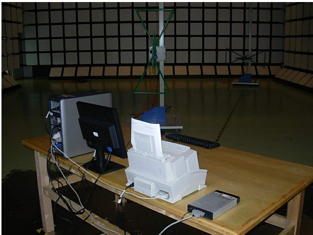
SETUP WITH MAXIMUM DETECTED EMISSION AT VERTICAL POLARIZATION (VGA 800*600@75Hz)
