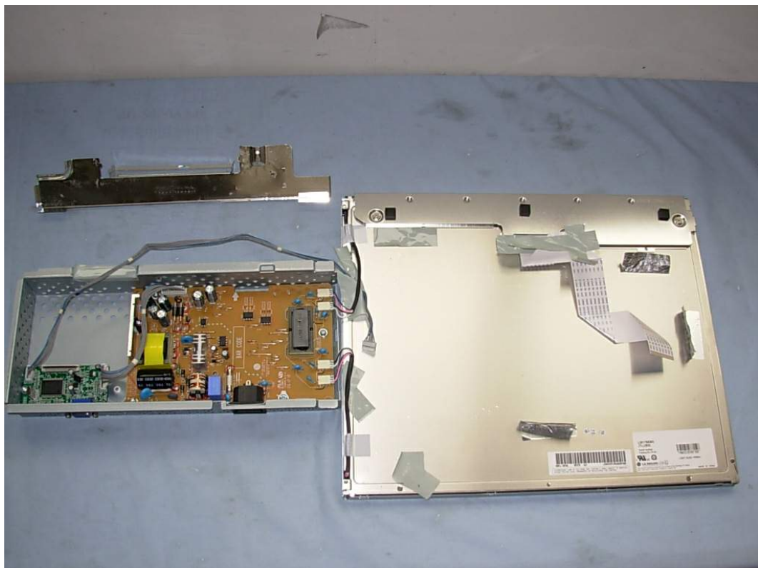
FIGURE 2 LCD MONITOR (M/N: L1719SS) SHIELDED COVER
