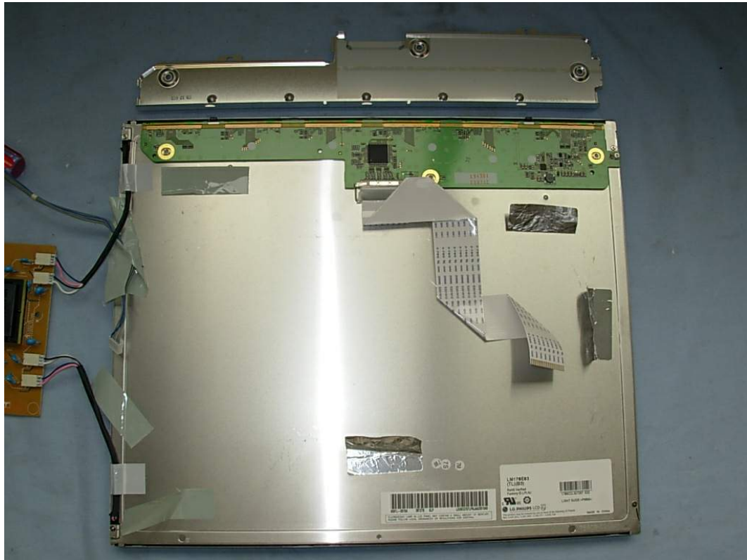
FIGURE 11 LCD MONITOR (M/N: L1719SS) LCD PANEL SHIELDED SHELL REMOVED
