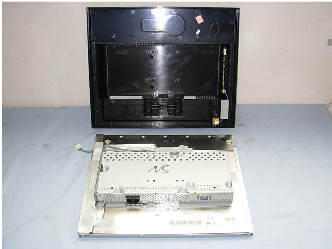
FIGURE 1 LCD MONITOR (M/N: L1719SS) COVER REMOVED
