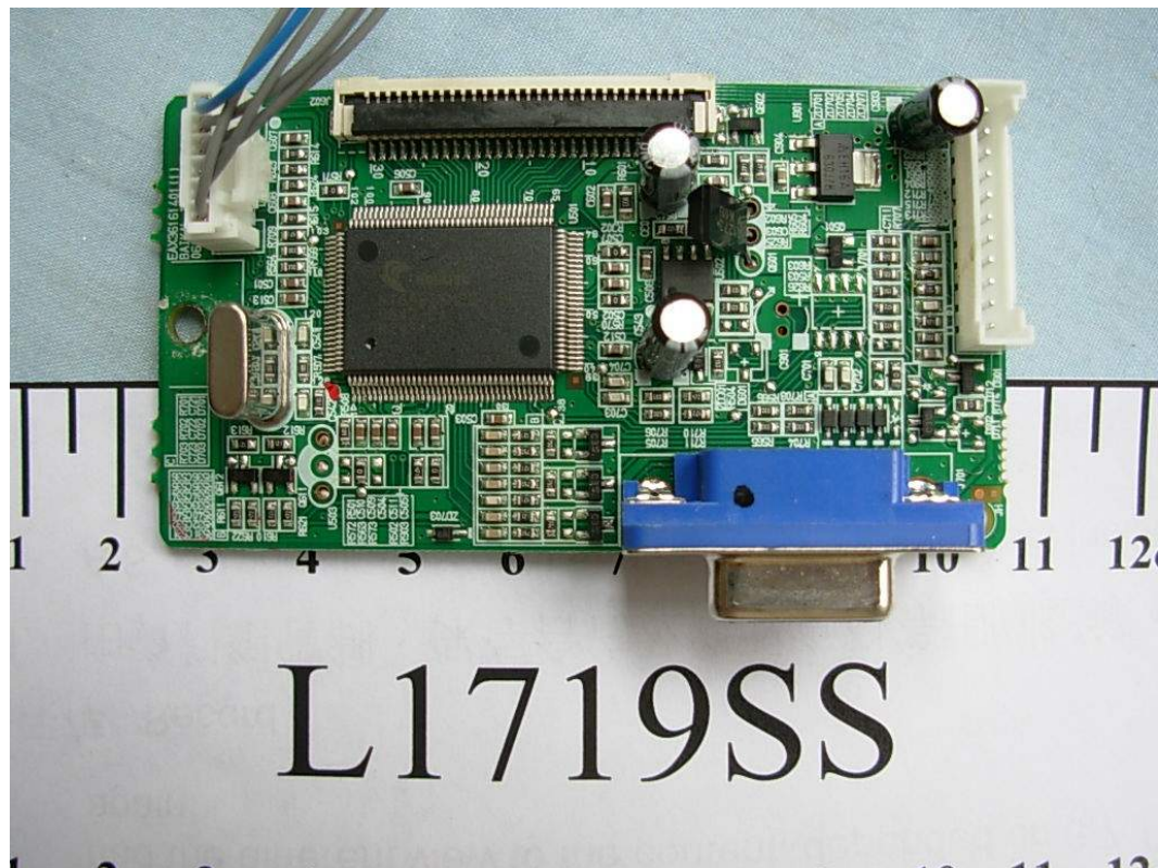
FIGURE 3 LCD MONITOR (M/N: L1719SS) MAIN BOARD (COMPONENT SIDE)
