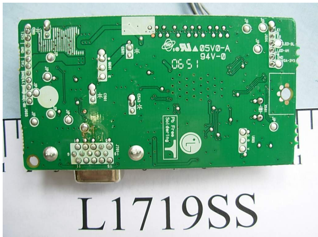
FIGURE 4 LCD MONITOR (M/N: L1719SS) MAIN BOARD (SOLDERED SIDE)
