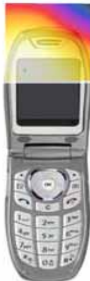
Figure 28 Sample H-field Scan Overlay
