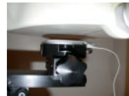
Figure 14.5 Body SAR Test Setup -- w/o Belt-clip --
