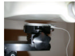
Figure 14.5 Body SAR Test Setup -- w/o Belt-clip --
