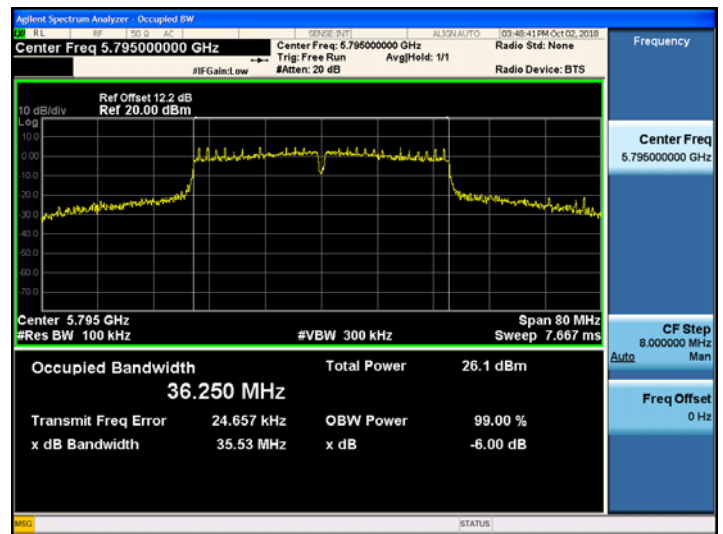
802.11ac_VHT40 UNII 3 BAND 6dB Bandwidth(CH.159)
