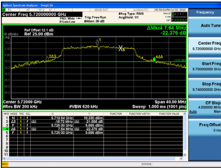
802.11ac_VHT20 CH.144 Bandwidth
