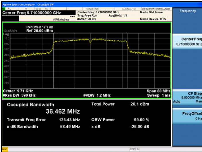
802.11ac_VHT40 UNII 2C BAND 26dB Bandwidth(CH 142)
