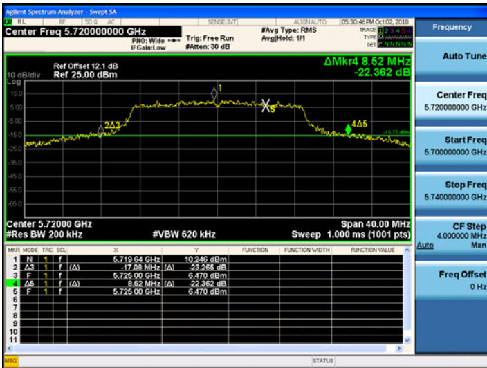
802.11ac_VHT20 CH.144 Bandwidth
