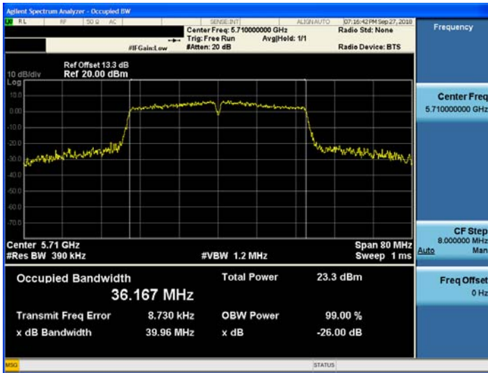
802.11n_HT40 UNII 2C BAND 26dB Bandwidth(CH 142)
