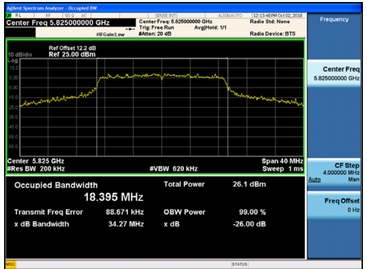
802.11n_HT20 UNII 3 BAND 26dB Bandwidth(CH 165)
