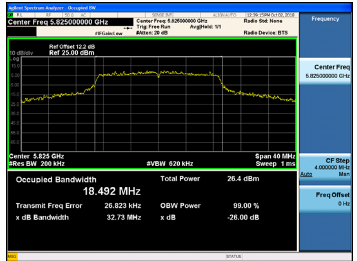
802.11ac_VHT20 UNII 3 BAND 26dB Bandwidth(CH 165)
