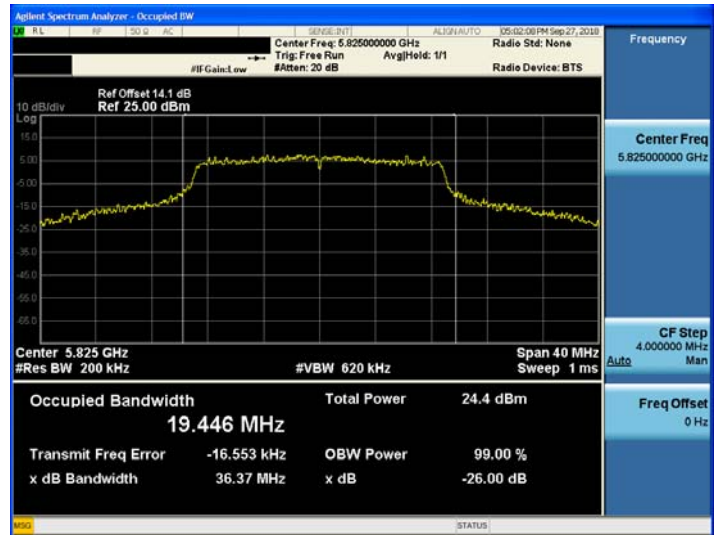
802.11n_HT20 UNII 3 BAND 26dB Bandwidth(CH 165)
