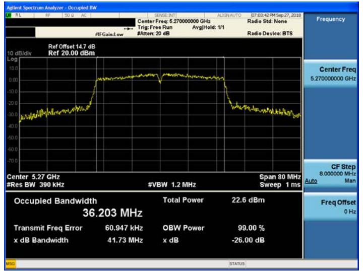
802.11n_HT40 UNII 3 BAND 26dB Bandwidth (CH 159)
