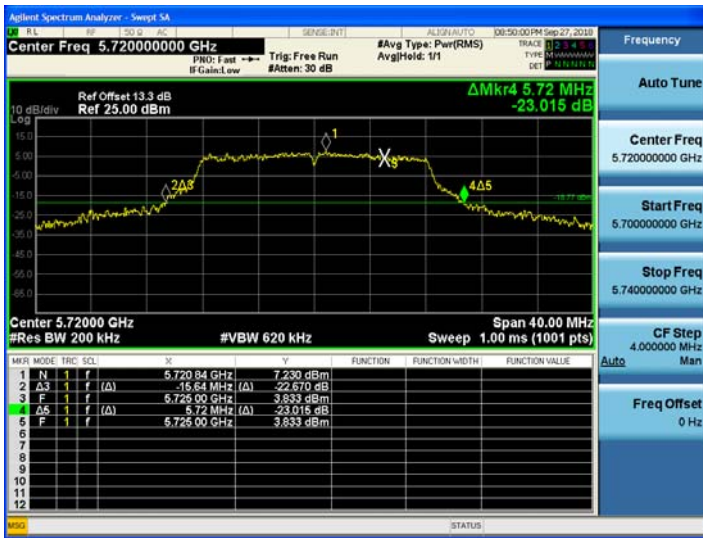
802.11ac_VHT20 CH.144 Bandwidth
