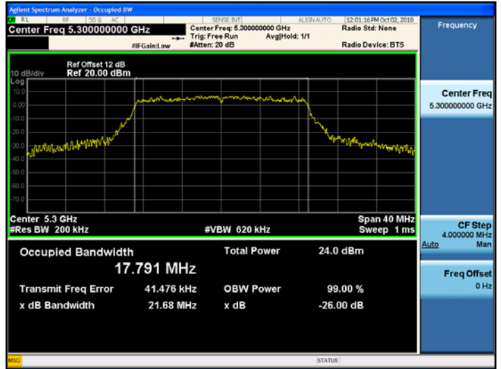
802.11n_HT20 UNII 3 BAND 26dB Bandwidth(CH 165)
