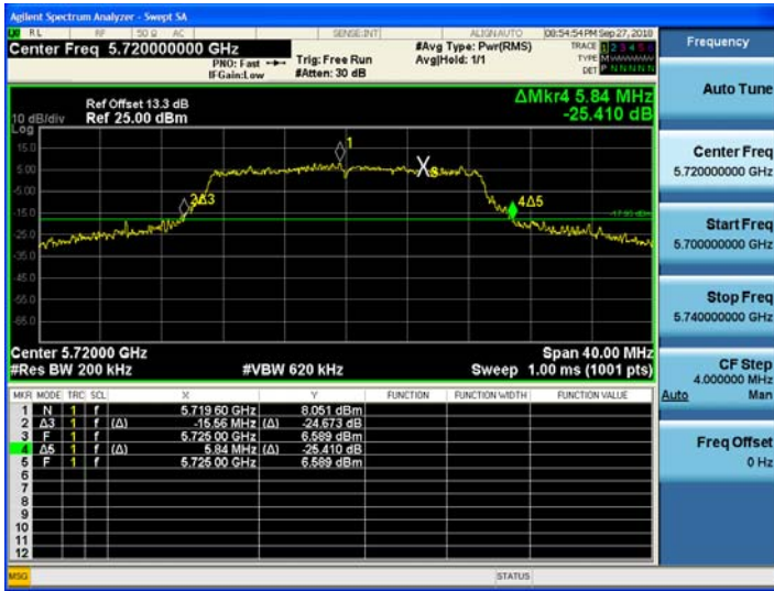
802.11ac_VHT20 CH.144 Bandwidth
