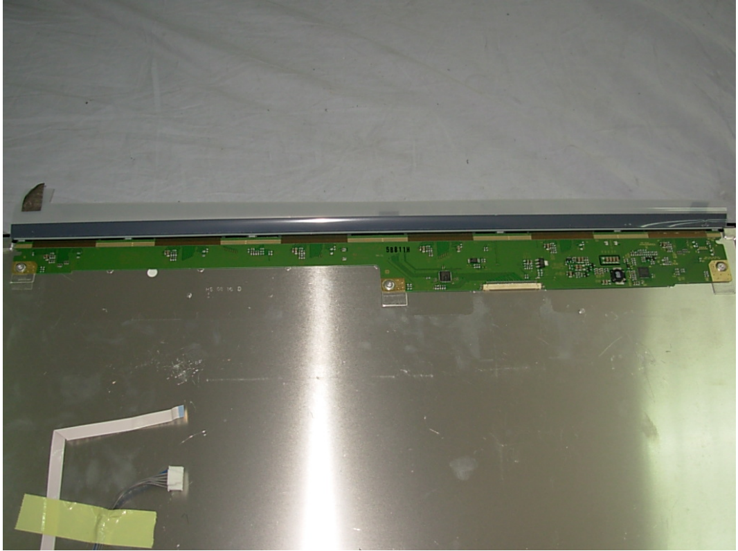
FIGURE 3 LCD MONITOR (M/N: E2241SX) PANEL BOARD (COMPONENT SIDE)
