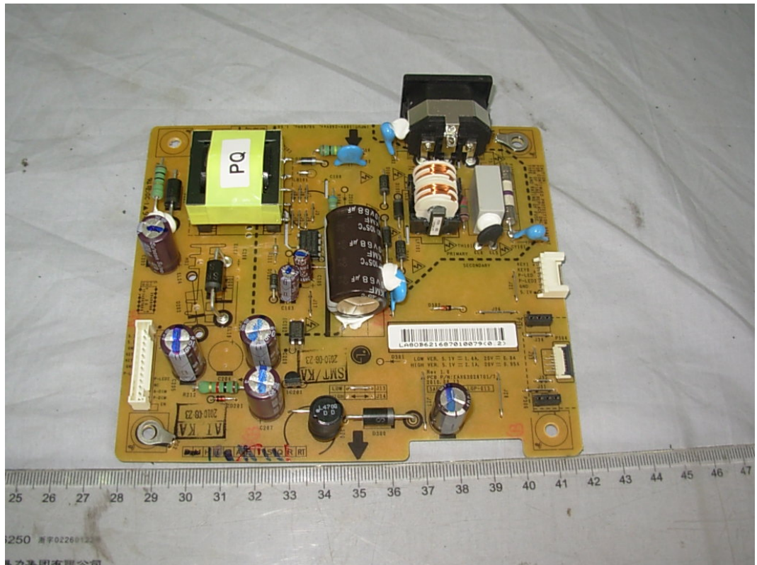
FIGURE 5 LCD MONITOR (M/N: E2241SX) POWER BOARD (COMPONENT SIDE)
