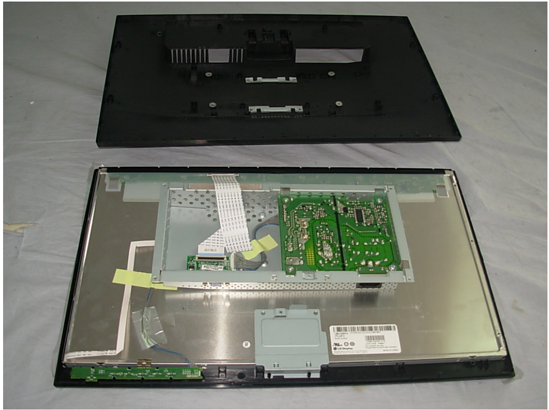
FIGURE 1 LCD MONITOR (M/N: E2241SX) COVER REMOVED
