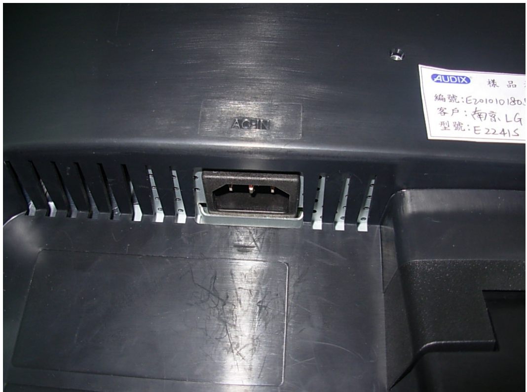
FIGURE 4 LCD MONITOR (M/N: E2241SX) AC POWER PORT
