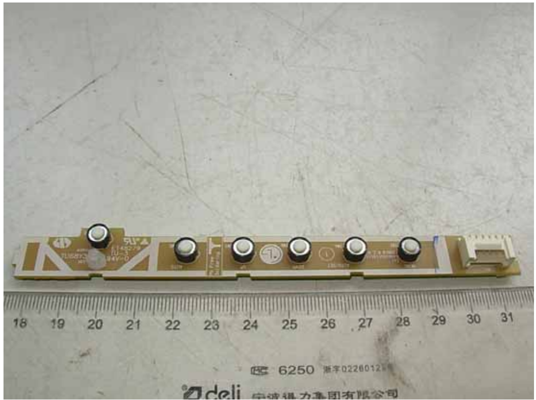
FIGURE 8 LCD MONITOR (M/N: E1948SX) KEY BOARD (COMPONENT SIDE)
