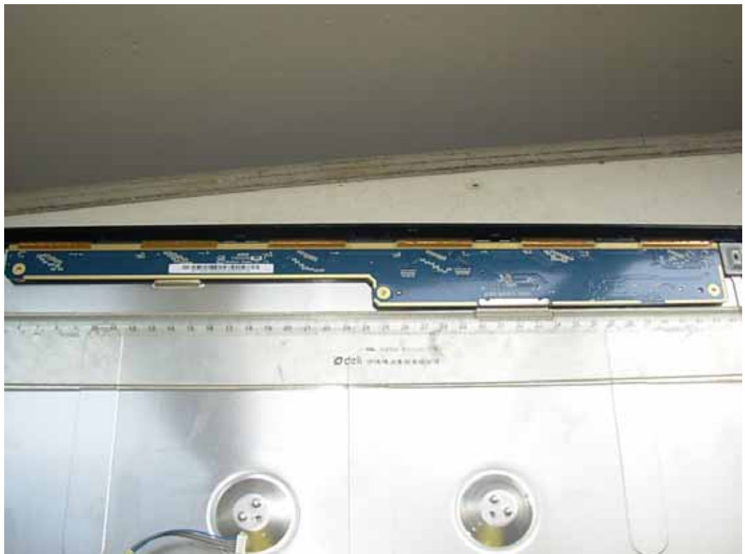
FIGURE 7 LCD MONITOR (M/N: E1948SX) DISPLAY BOARD (SOLDERED SIDE)
