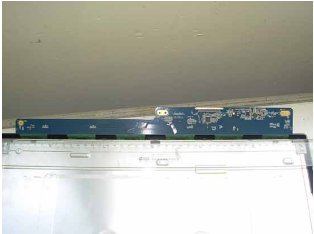
FIGURE 6 LCD MONITOR (M/N: E1948SX) DISPLAY BOARD (COMPONENT SIDE)
