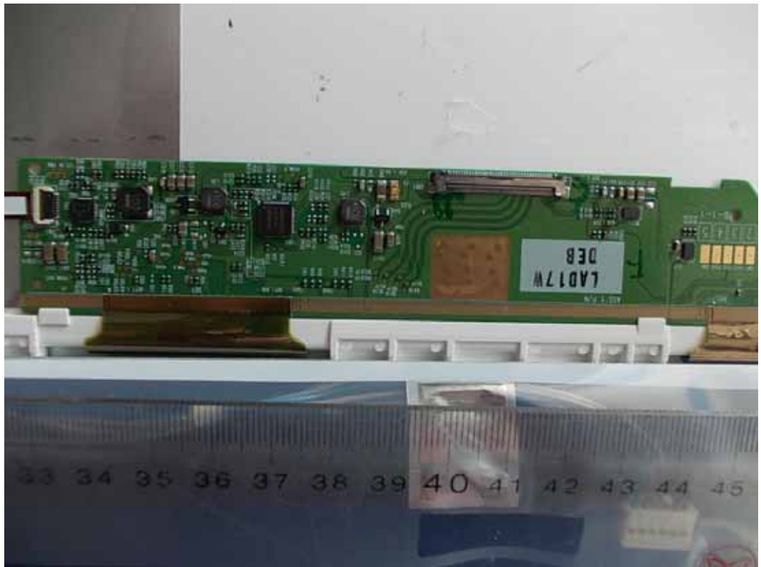
FIGURE 14 LCD MONITOR (M/N: E1641CX) LCD PANEL CONTROL BOARD #2(COMPONENT SIDE #1)
