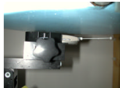
Figure 19. Body SAR Test Setup
