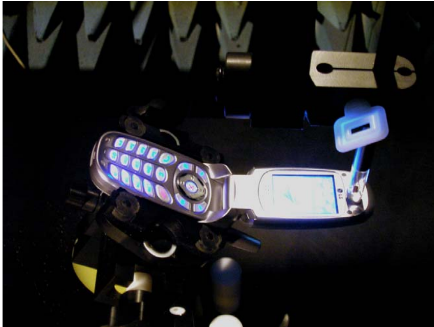
Figure 12-1 Test Setup for Wireless Device
