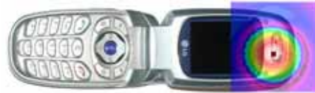
Figure A T-coil Location
