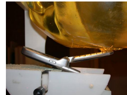
Figure A.8 Left Head SAR Test Setup -- Ear / 15° Tilt Position --
