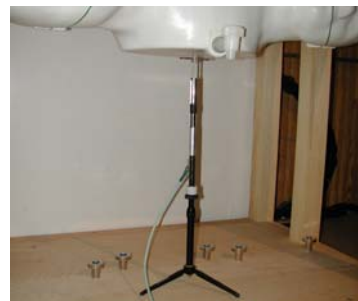
Figure 12.1 Dipole Validation Test Setup
