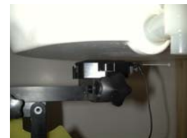
Figure 14.6 Body SAR Test Setup -- w/o Holster --
