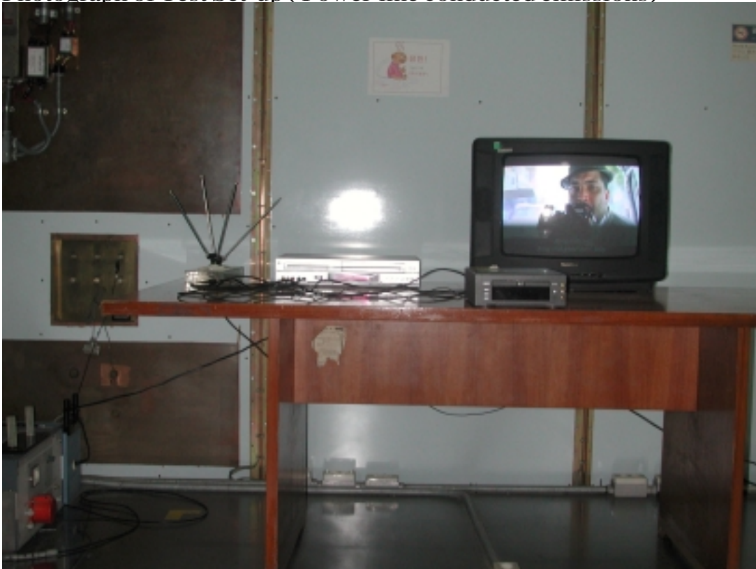
Photograph of Test Set-up ( Power line conducted emissions)
