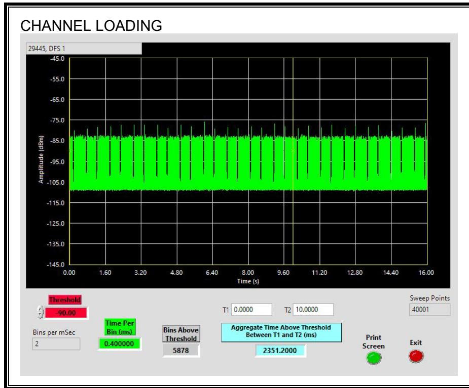
The level of traffic loading on the channel by the Peer Slave is 23.51%
