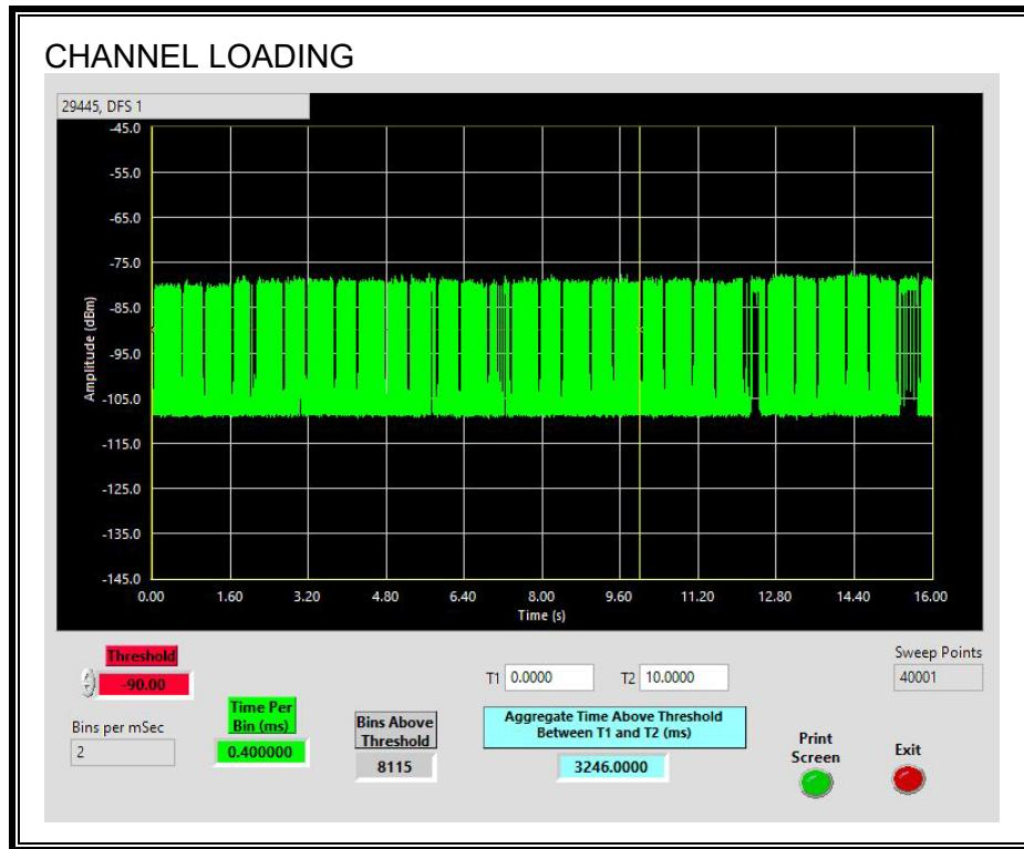
The level of traffic loading on the channel by the EUT is 32.46%
