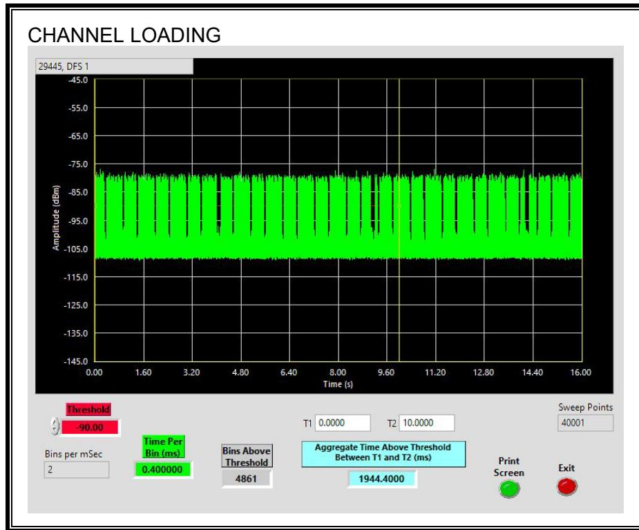
The level of traffic loading on the channel by the EUT is 19.44%
