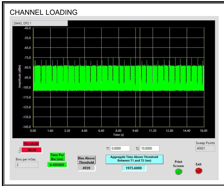
The level of traffic loading on the channel by the Peer Slave is 19.75%
