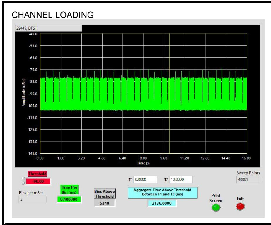
The level of traffic loading on the channel by the Peer Slave is 21.36%
