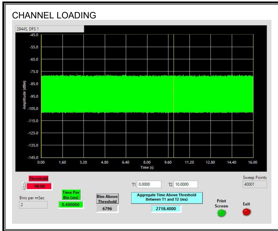
The level of traffic loading on the channel by the EUT is 27.18%
