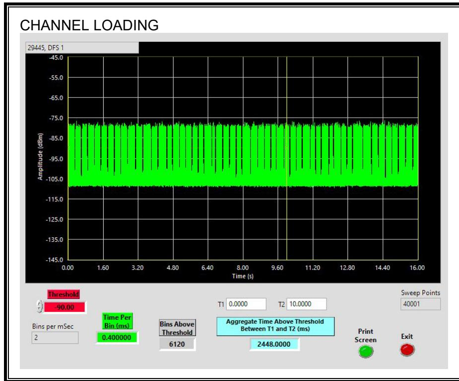
The level of traffic loading on the channel by the EUT is 24.48%
