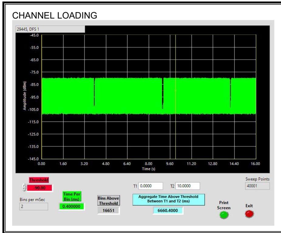
The level of traffic loading on the channel by the EUT is 66.6%
