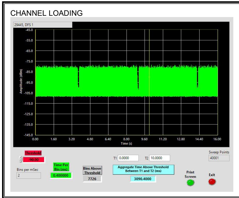
The level of traffic loading on the channel by the EUT is 30.9%
