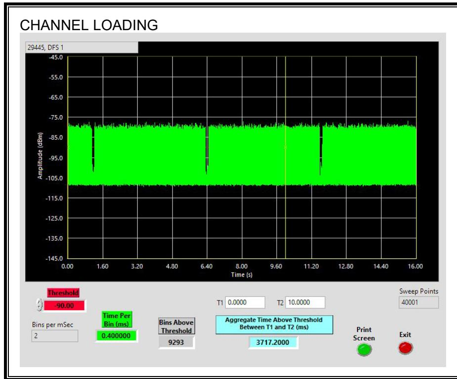
The level of traffic loading on the channel by the EUT is 37.17%
