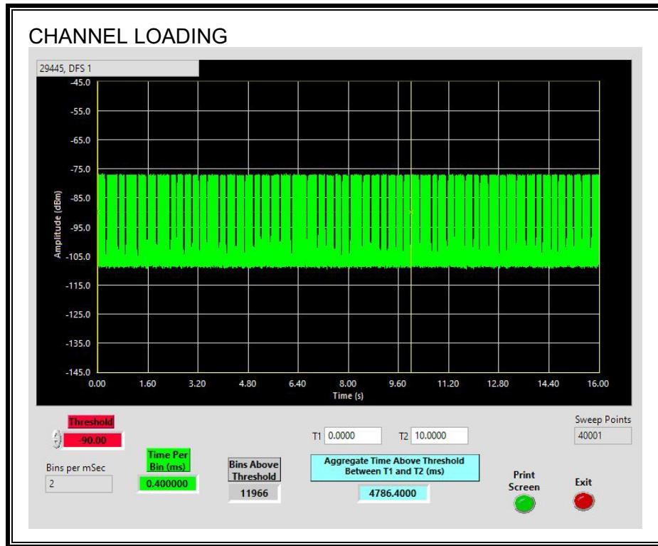
The level of traffic loading on the channel by the EUT is 47.86%
