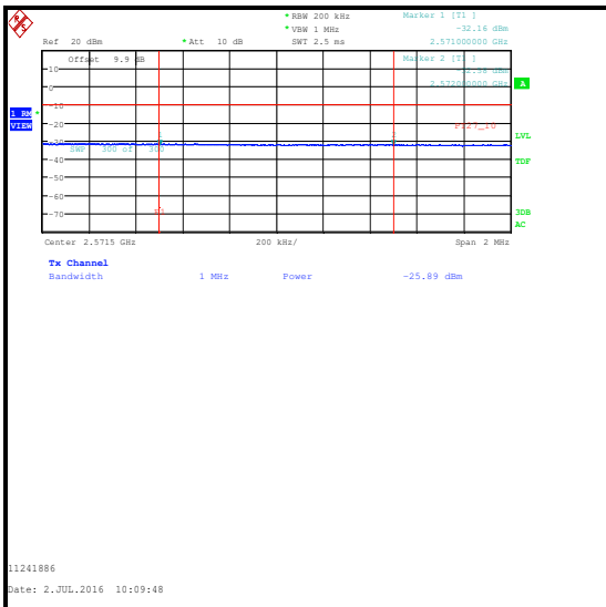
16QAM / 50 RB 0 Offset / 2571 to 2572 MHz / Integrated level
