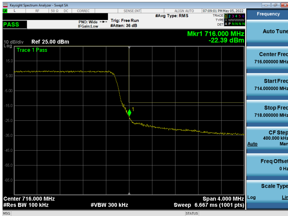
Plot 7-109. Upper Band Edge Plot (LTE Band 12 - 5MHz QPSK – Full RB)
