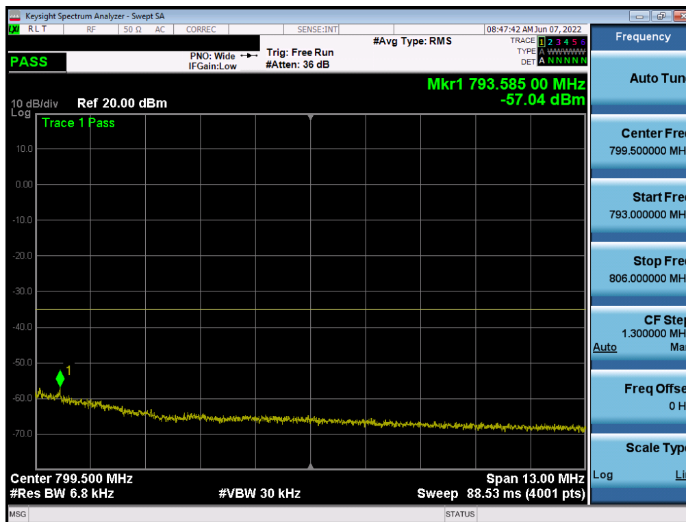
Plot 7-119. Upper Emission Mask Plot (LTE Band 13 - 5MHz QPSK – Full RB)
