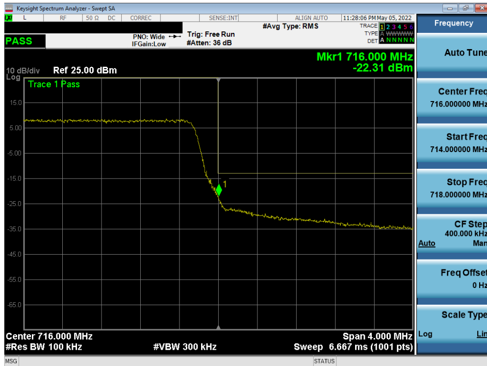
Plot 7-113. Upper Band Edge Plot (LTE Band 17 - 5MHz QPSK – Full RB)
