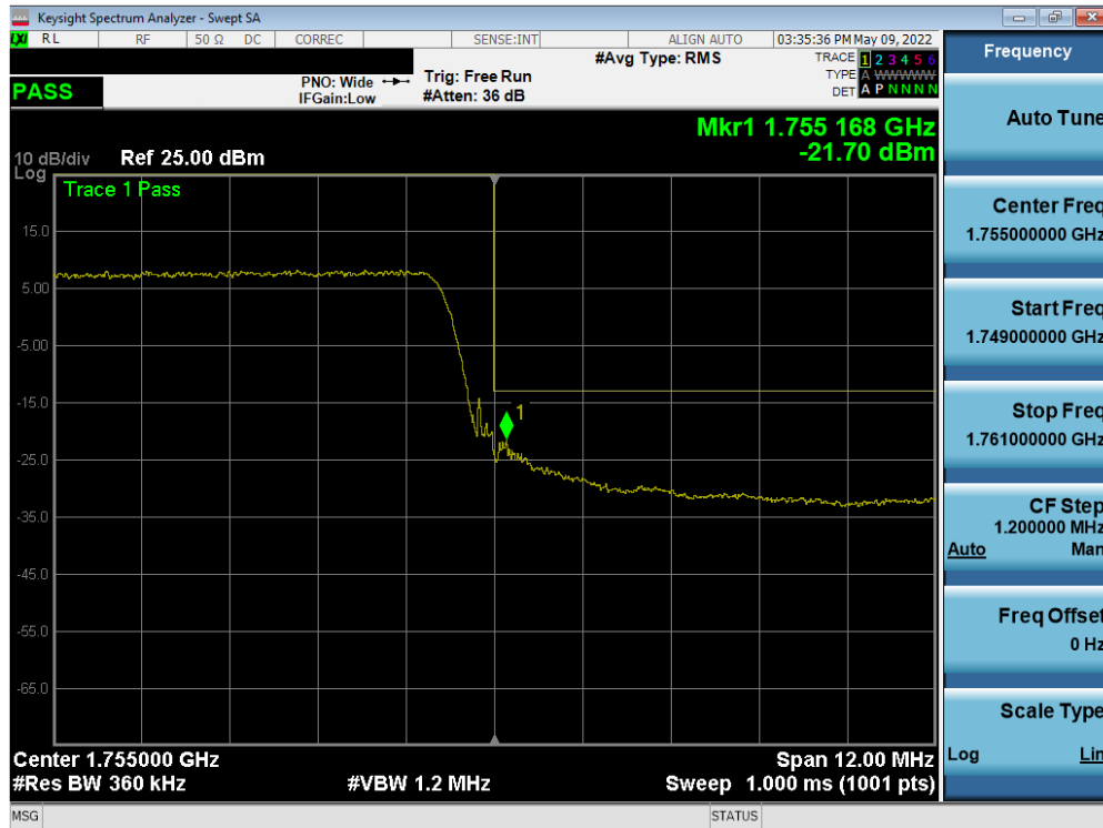
Plot 7-98. Upper Band Edge Plot (LTE Band 4 - 15MHz QPSK – Full RB)
