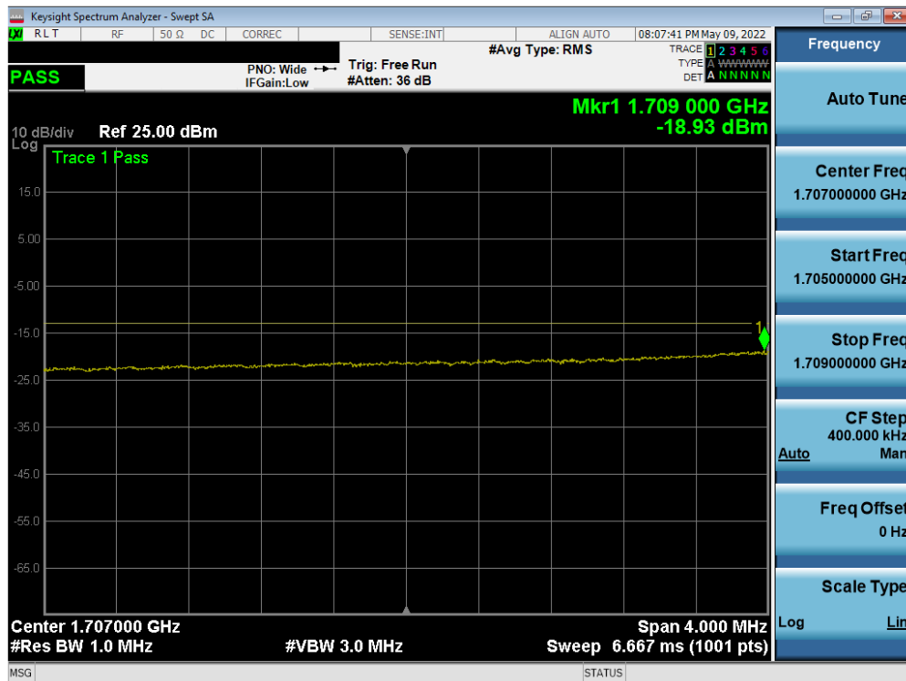
Plot 7-77. Lower Extended Band Edge Plot (LTE Band 66 - 20MHz QPSK – Full RB)
