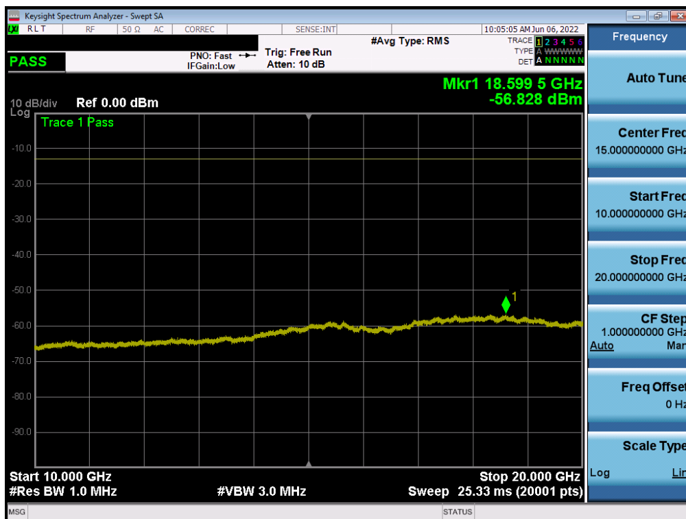
Plot 7-52. Conducted Spurious Plot (WCDMA Ch. 1413- Mid Channel)
