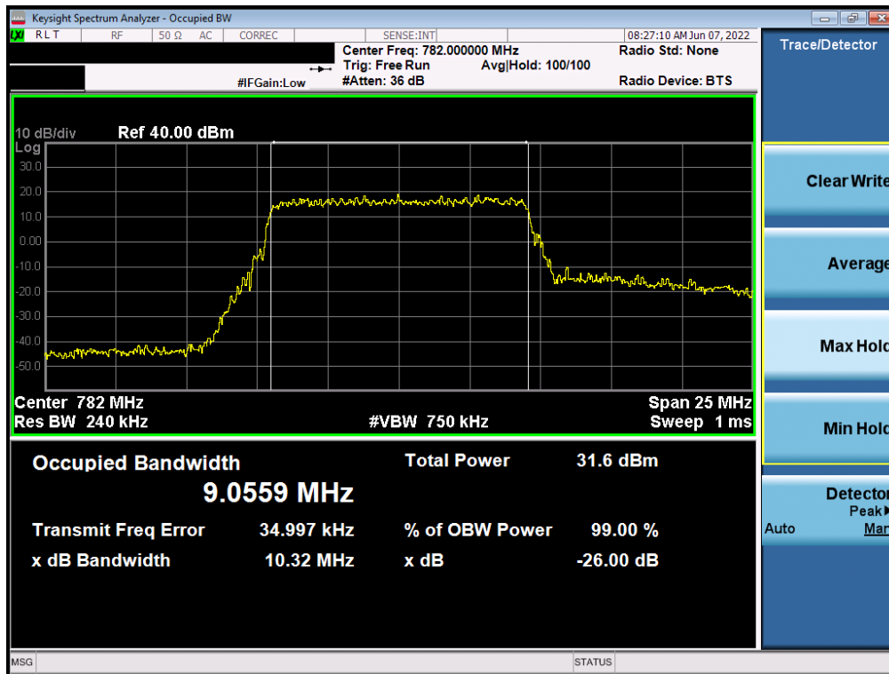
Plot 7-23. Occupied Bandwidth Plot (LTE Band 13 - 10MHz QPSK - Full RB)
