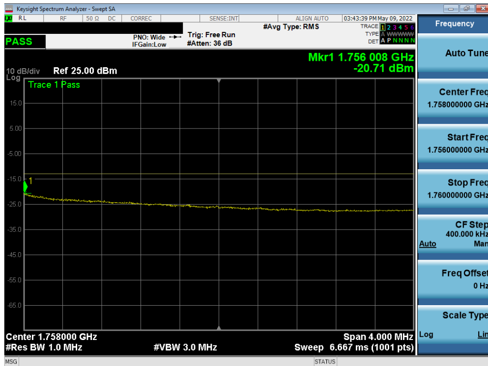
Plot 7-95. Upper Extended Band Edge Plot (LTE Band 4 - 10MHz QPSK – Full RB)
