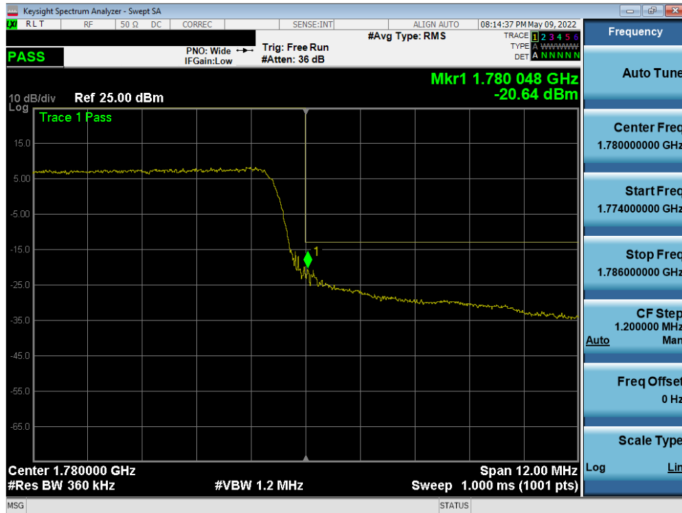
Plot 7-74. Upper Band Edge Plot (LTE Band 66 - 15MHz QPSK – Full RB)
