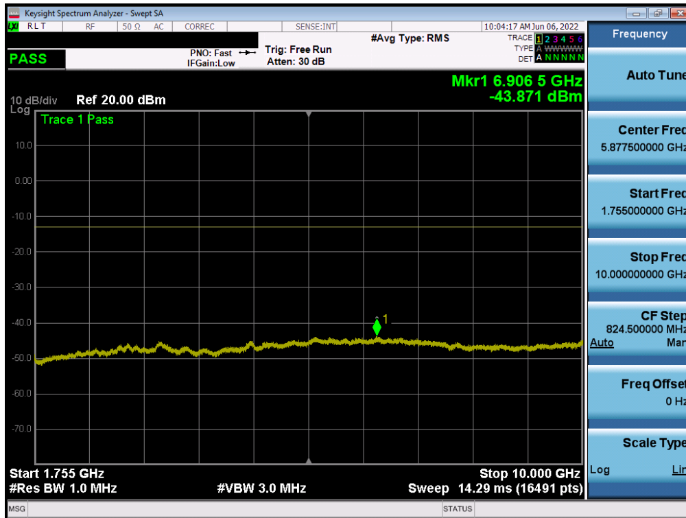
Plot 7-51. Conducted Spurious Plot (WCDMA Ch. 1413- Mid Channel)
