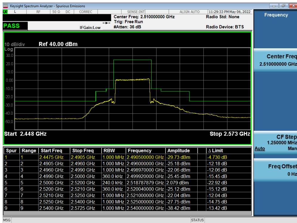
Plot 7-44. Lower ACP Plot (LTE Band 7 - 20MHz QPSK – Full RB)
