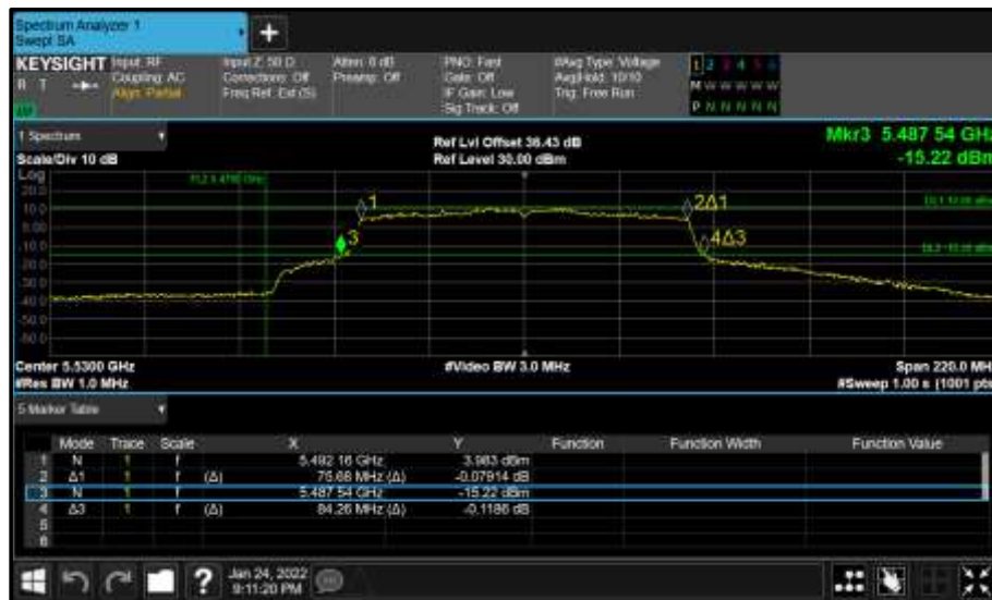
Figure 432 - Core 0 (A) 5530 MHz (CH106) 26 dB and 99% Bandwidth
