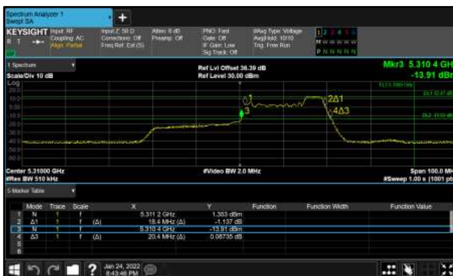
Figure 363 - Core 1 (B) 5310 MHz (CH62) 26 dB and 99% Bandwidth
