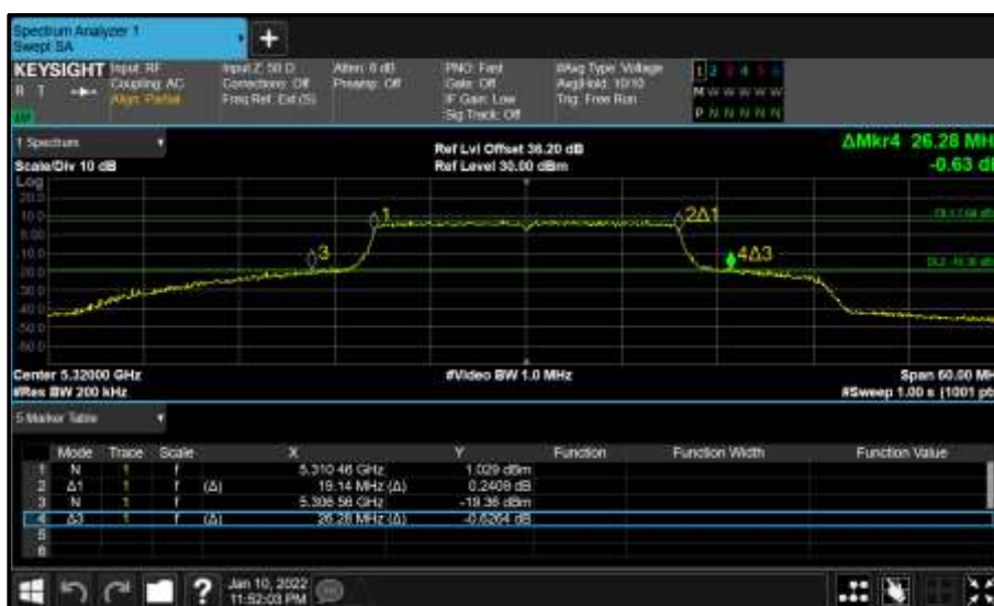
Figure 321 - Core 0 (A) 5320 MHz (CH64) 26 dB and 99% Bandwidth
