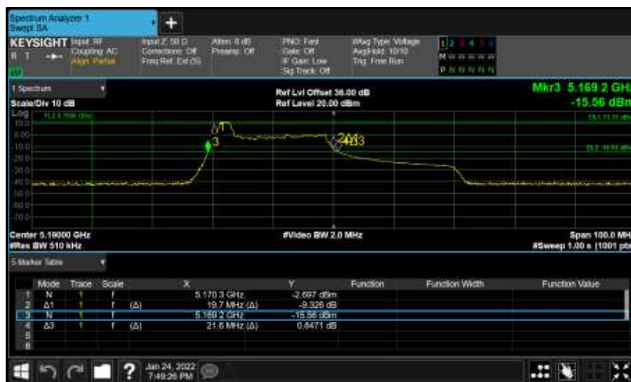
Figure 247 - Core 0 (A) 5190 MHz (CH38) 26 dB and 99% Bandwidth
