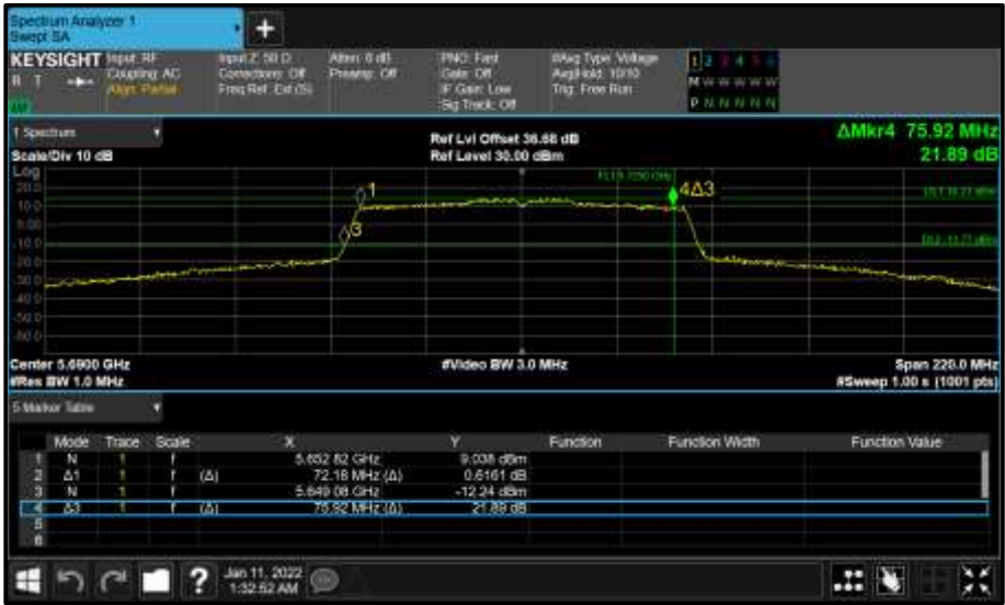
Figure 425 - Core 0 (A) 5690 MHz (CH138) 26 dB and 99% Bandwidth
