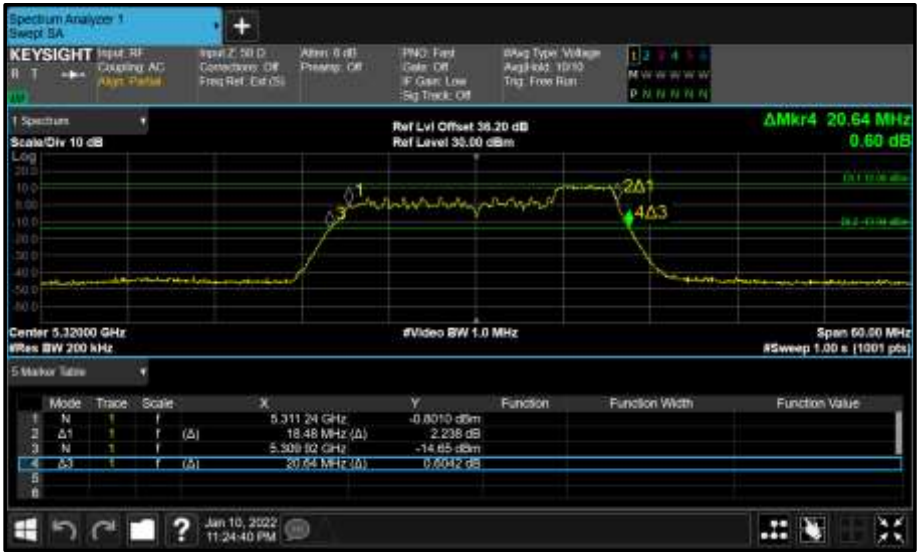
Figure 331 - Core 0 (A) 5320 MHz (CH64) 26 dB and 99% Bandwidth
