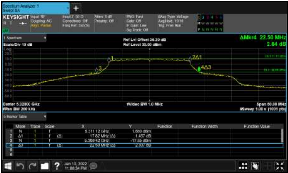
Figure 286 - Core 0 (A) 5320 MHz (CH64) 26 dB and 99% Bandwidth
