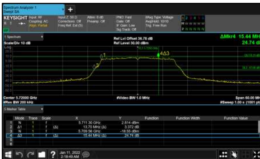
Figure 393 - Core 0 (A) 5720 MHz (CH144) 26 dB and 99% Bandwidth
