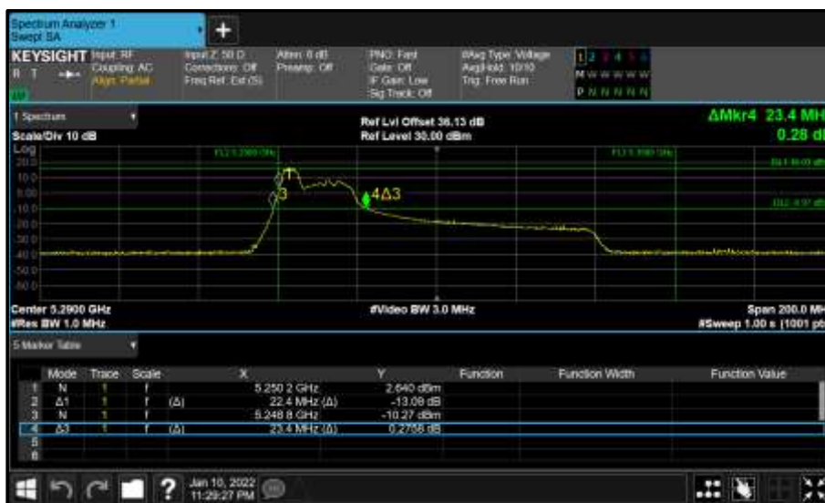
Figure 369 - Core 0 (A) 5290 MHz (CH58) 26 dB and 99% Bandwidth
