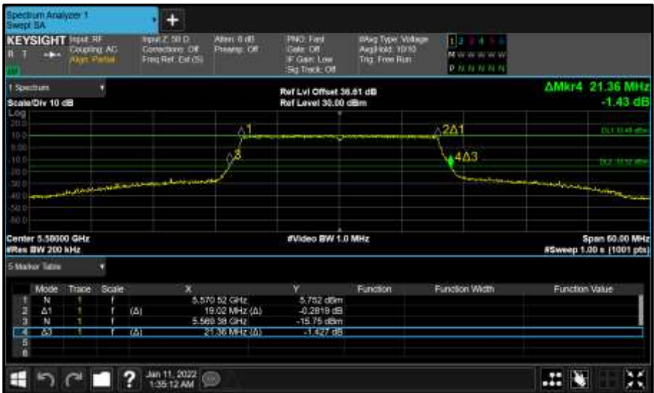
Figure 439 - Core 0 (A) 5580 MHz (CH116) 26 dB and 99% Bandwidth
