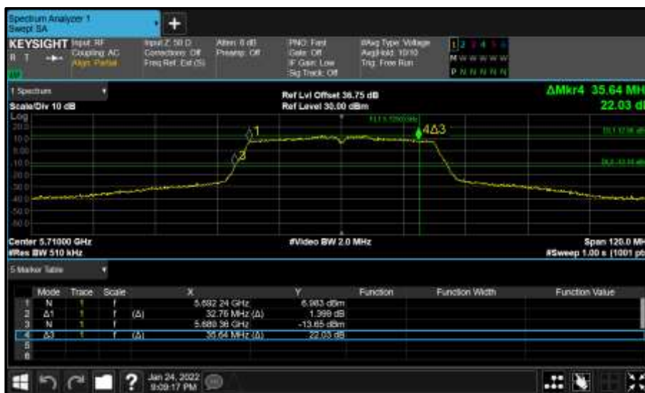
Figure 421 - Core 0 (A) 5710 MHz (CH142) 26 dB and 99% Bandwidth
