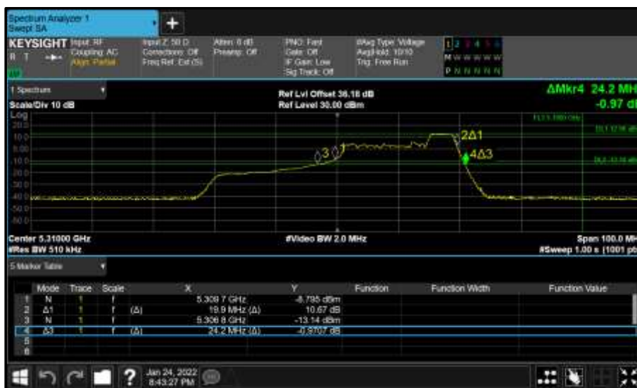
Figure 362 - Core 0 (A) 5310 MHz (CH62) 26 dB and 99% Bandwidth
