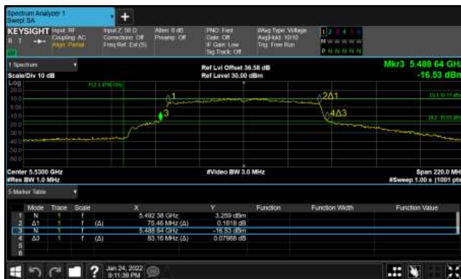
Figure 433 - Core 1 (B) 5530 MHz (CH106) 26 dB and 99% Bandwidth
