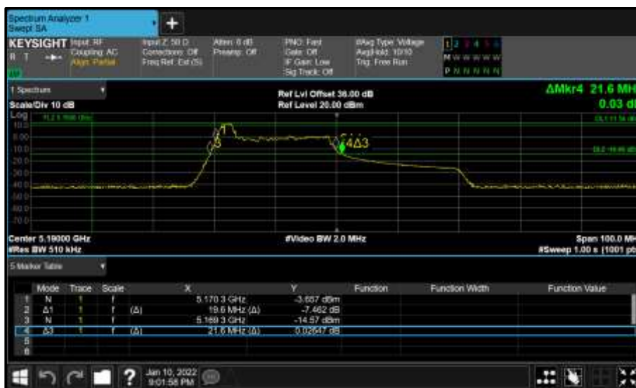
Figure 233 - Core 0 (A) 5190 MHz (CH38) 26 dB and 99% Bandwidth
