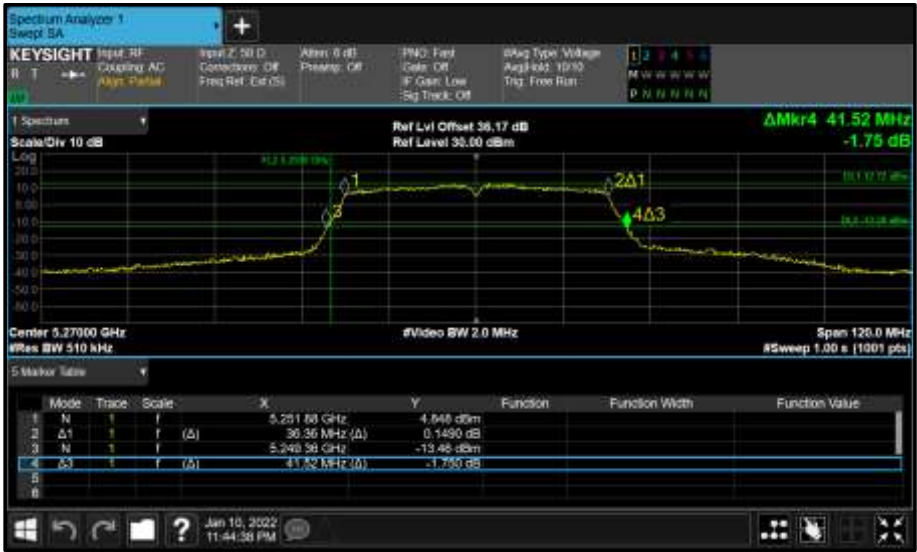
Figure 301 - Core 0 (A) 5270 MHz (CH54) 26 dB and 99% Bandwidth
