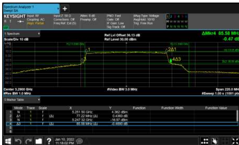
Figure 364 - Core 0 (A) 5290 MHz (CH58) 26 dB and 99% Bandwidth
