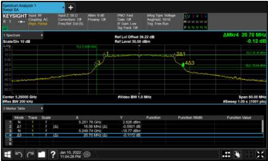
Figure 281 - Core 0 (A) 5260 MHz (CH52) 26 dB and 99% Bandwidth
