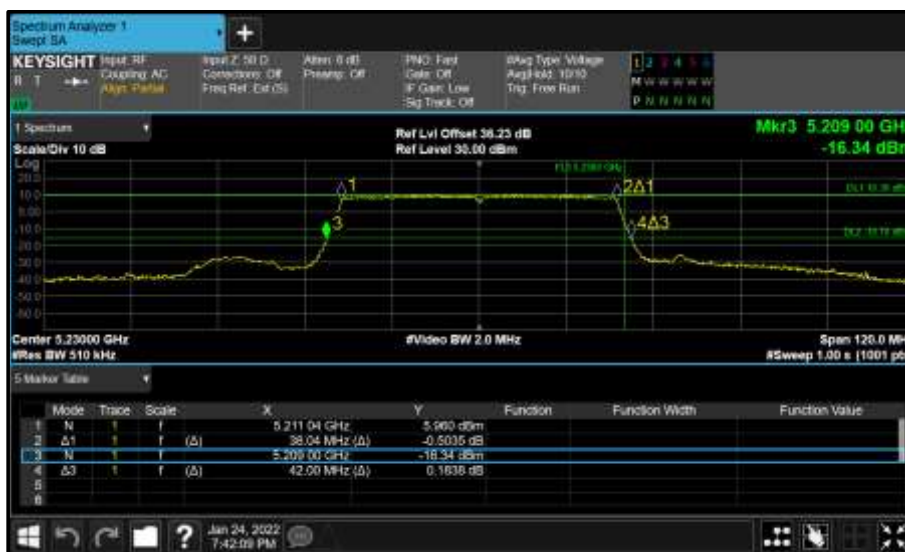
Figure 229 - Core 0 (A) 5230 MHz (CH46) 26 dB and 99% Bandwidth
