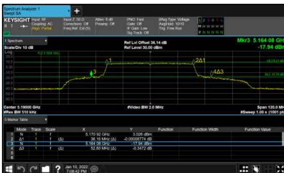
Figure 216 - Core 1 (B) 5190 MHz (CH38) 26 dB and 99% Bandwidth
