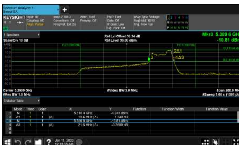
Figure 374 - Core 1 (B) 5290 MHz (CH58) 26 dB and 99% Bandwidth
