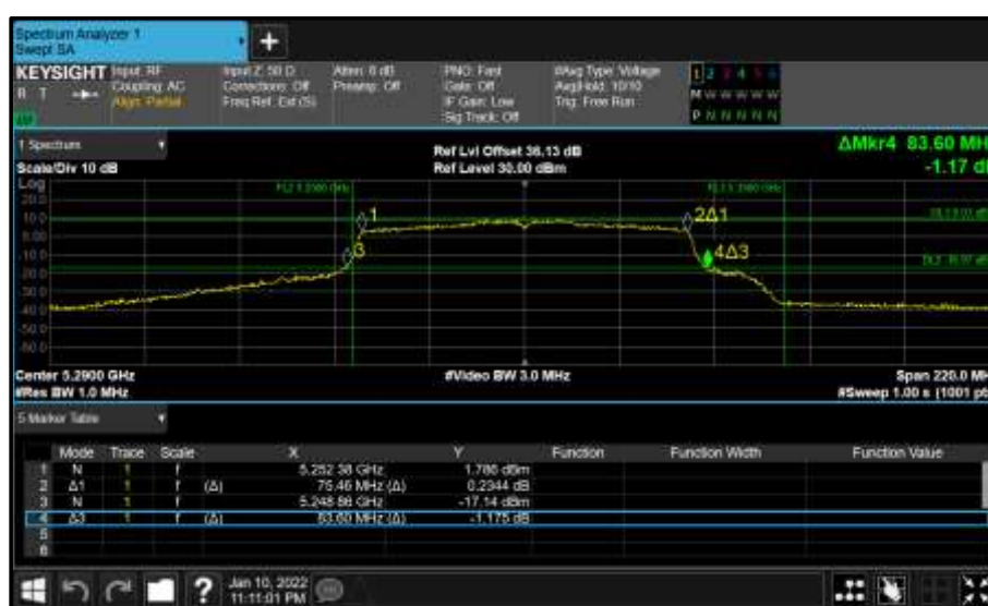
Figure 309 - Core 0 (A) 5290 MHz (CH58) 26 dB and 99% Bandwidth
