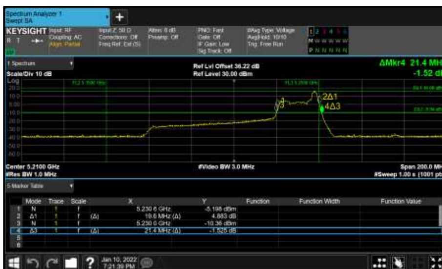
Figure 268 - Core 1 (B) 5210 MHz (CH42) 26 dB and 99% Bandwidth
