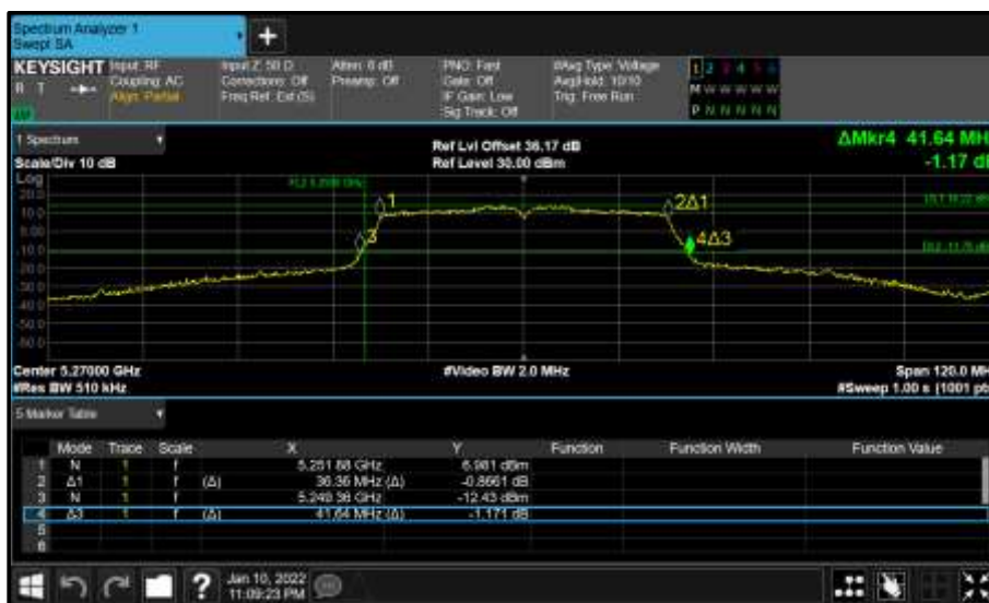
Figure 299 - Core 0 (A) 5270 MHz (CH54) 26 dB and 99% Bandwidth
