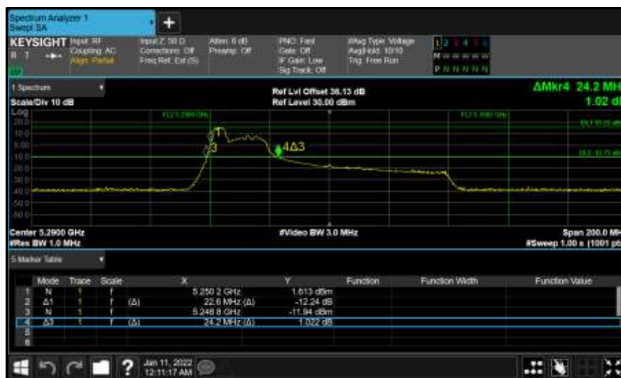
Figure 371 - Core 0 (A) 5290 MHz (CH58) 26 dB and 99% Bandwidth
