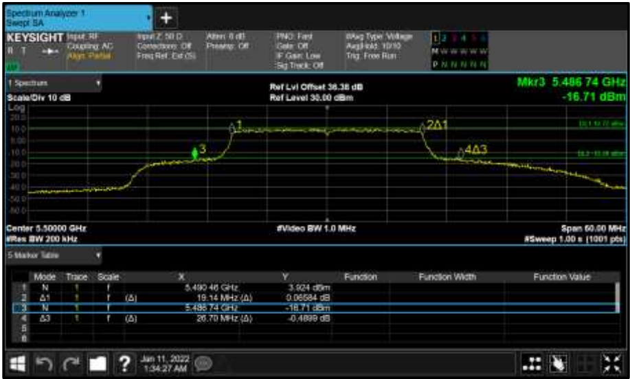
Figure 438 - Core 0 (A) 5500 MHz (CH100) 26 dB and 99% Bandwidth
