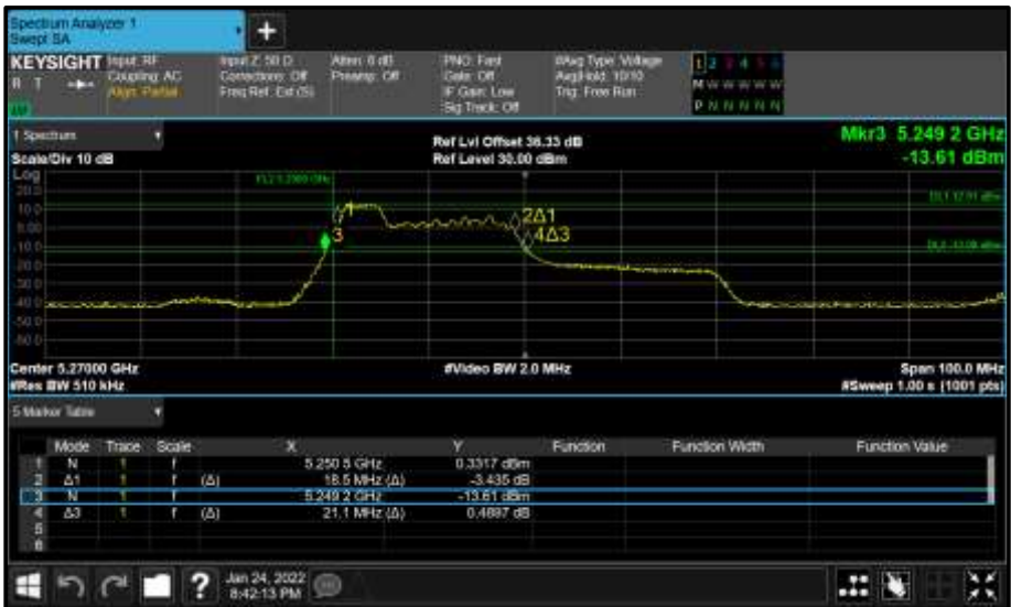
Figure 361 - Core 1 (B) 5270 MHz (CH54) 26 dB and 99% Bandwidth
