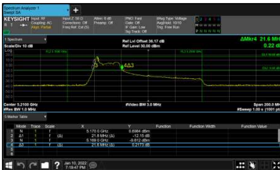
Figure 265 - Core 0 (A) 5210 MHz (CH42) 26 dB and 99% Bandwidth
