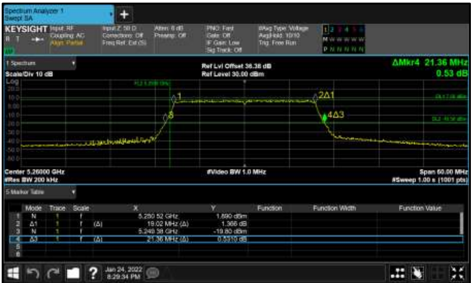
Figure 324 - Core 1 (B) 5260 MHz (CH52) 26 dB and 99% Bandwidth
