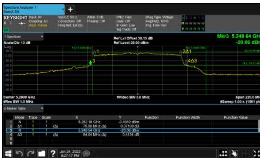
Figure 312 - Core 0 (A) 5290 MHz (CH58) 26 dB and 99% Bandwidth
