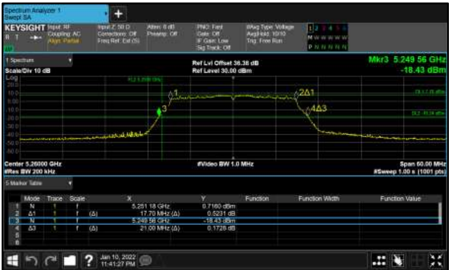
Figure 288 - Core 1 (B) 5260 MHz (CH52) 26 dB and 99% Bandwidth
