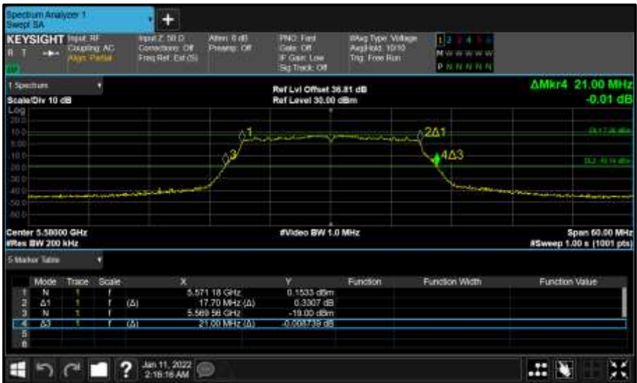
Figure 390 - Core 1 (B) 5580 MHz (CH116) 26 dB and 99% Bandwidth
