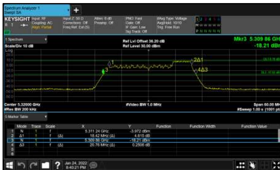
Figure 342 - Core 0 (A) 5320 MHz (CH64) 26 dB and 99% Bandwidth
