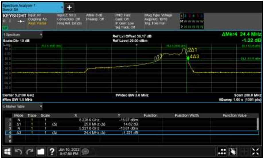
Figure 271 - Core 0 (A) 5210 MHz (CH42) 26 dB and 99% Bandwidth
