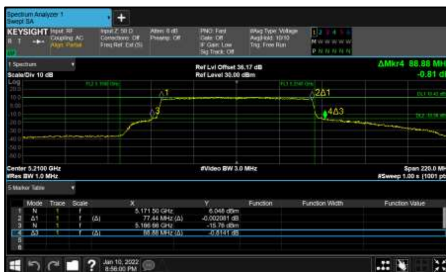
Figure 252 - Core 0 (A) 5210 MHz (CH42) 26 dB and 99% Bandwidth
