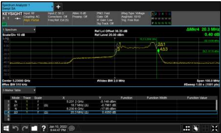
Figure 242 - Core 1 (B) 5230 MHz (CH46) 26 dB and 99% Bandwidth
