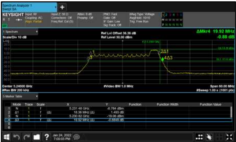
Figure 204 - Core 1 (B) 5240 MHz (CH48) 26 dB and 99% Bandwidth
