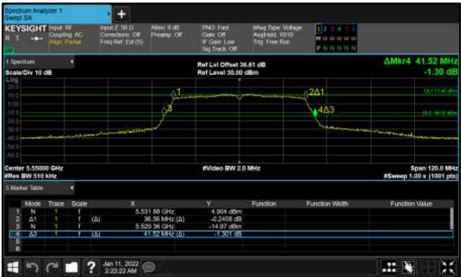
Figure 410 - Core 1 (B) 5550 MHz (CH110) 26 dB and 99% Bandwidth
