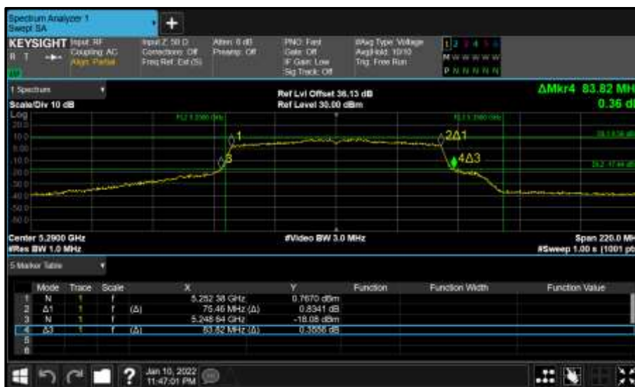
Figure 310 - Core 0 (A) 5290 MHz (CH58) 26 dB and 99% Bandwidth
