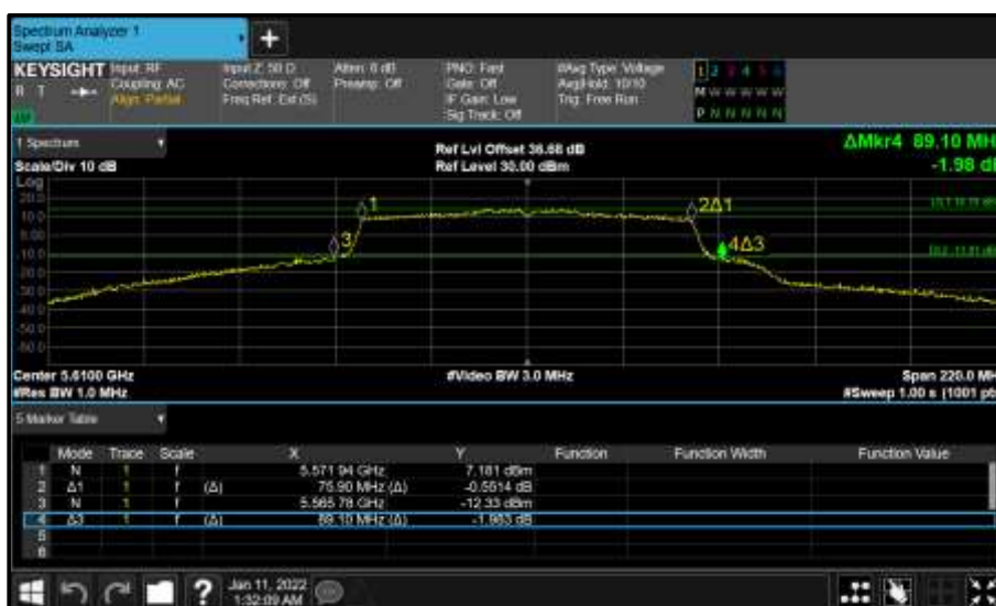
Figure 424 - Core 0 (A) 5610 MHz (CH122) 26 dB and 99% Bandwidth
