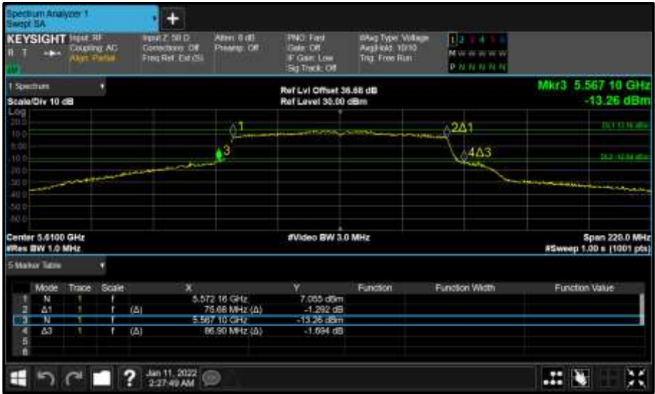
Figure 428 - Core 0 (A) 5610 MHz (CH122) 26 dB and 99% Bandwidth
