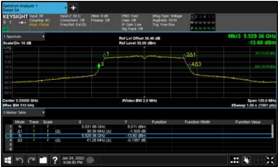
Figure 417 - Core 0 (A) 5550 MHz (CH110) 26 dB and 99% Bandwidth
