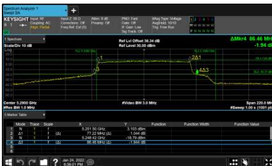
Figure 368 - Core 1 (B) 5290 MHz (CH58) 26 dB and 99% Bandwidth
