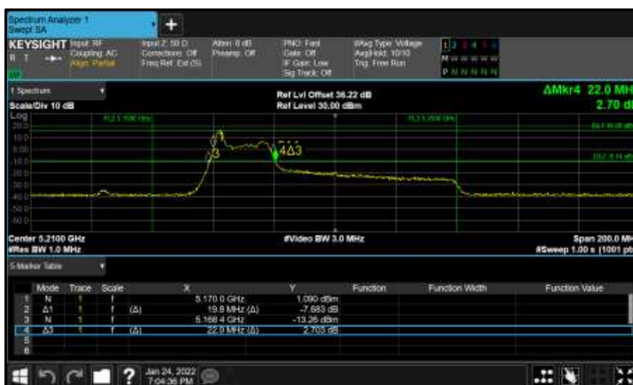
Figure 274 - Core 1 (B) 5210 MHz (CH42) 26 dB and 99% Bandwidth
