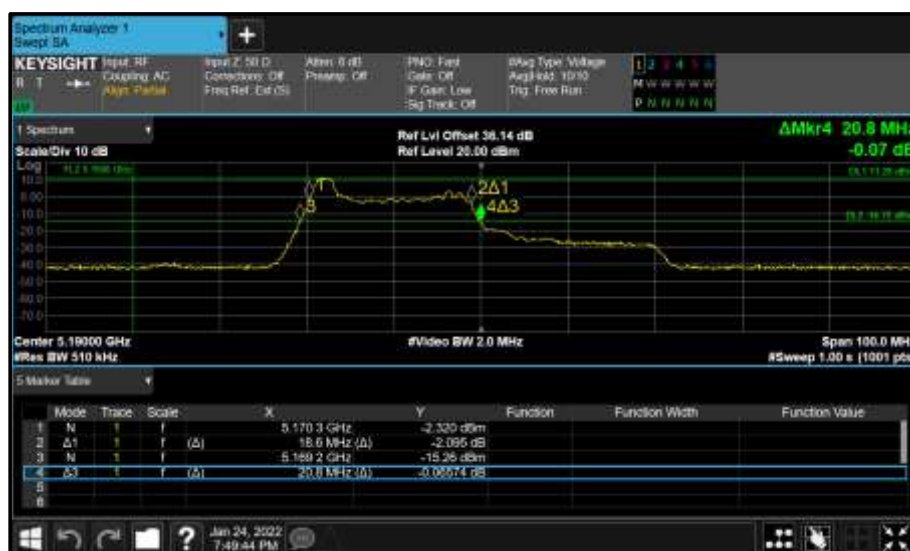
Figure 248 - Core 1 (B) 5190 MHz (CH38) 26 dB and 99% Bandwidth
