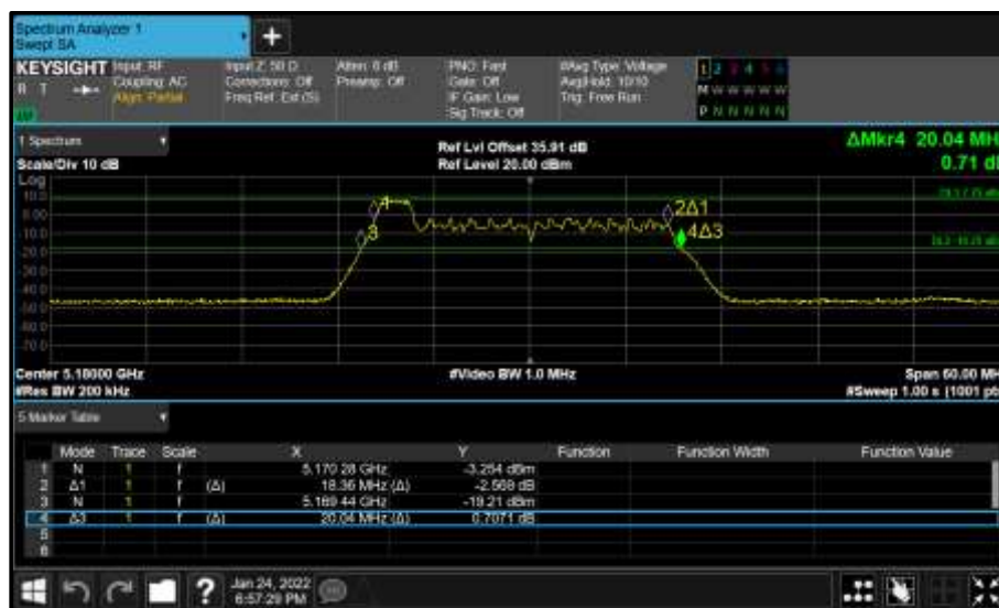
Figure 199 - Core 0 (A) 5180 MHz (CH36) 26 dB and 99% Bandwidth
