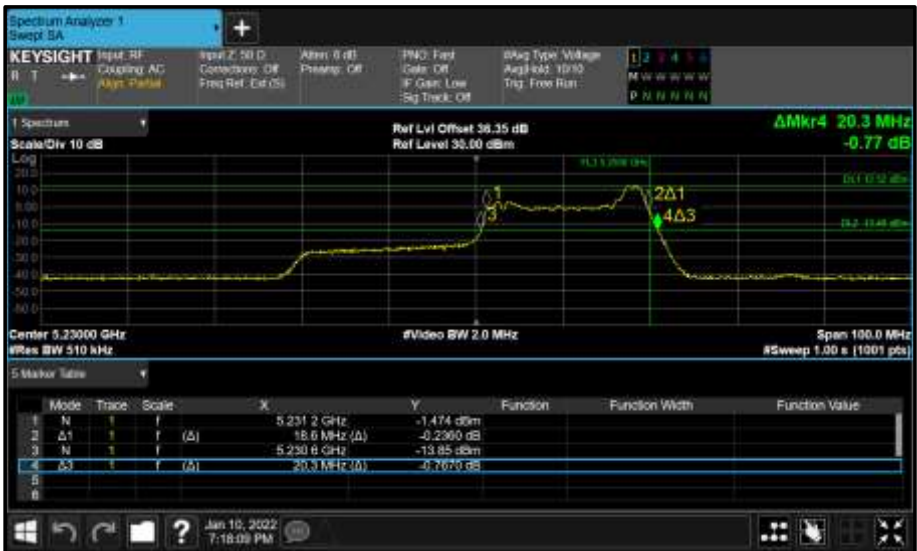
Figure 238 - Core 1 (B) 5230 MHz (CH46) 26 dB and 99% Bandwidth
