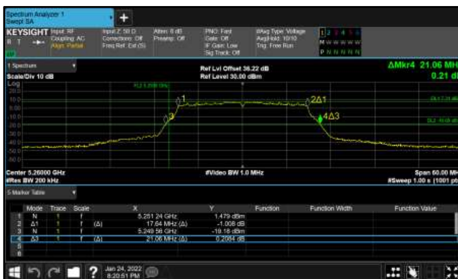
Figure 293 - Core 0 (A) 5260 MHz (CH52) 26 dB and 99% Bandwidth
