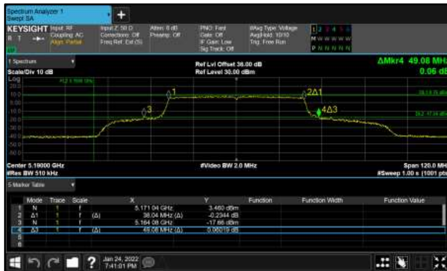
Figure 227 - Core 0 (A) 5190 MHz (CH38) 26 dB and 99% Bandwidth
