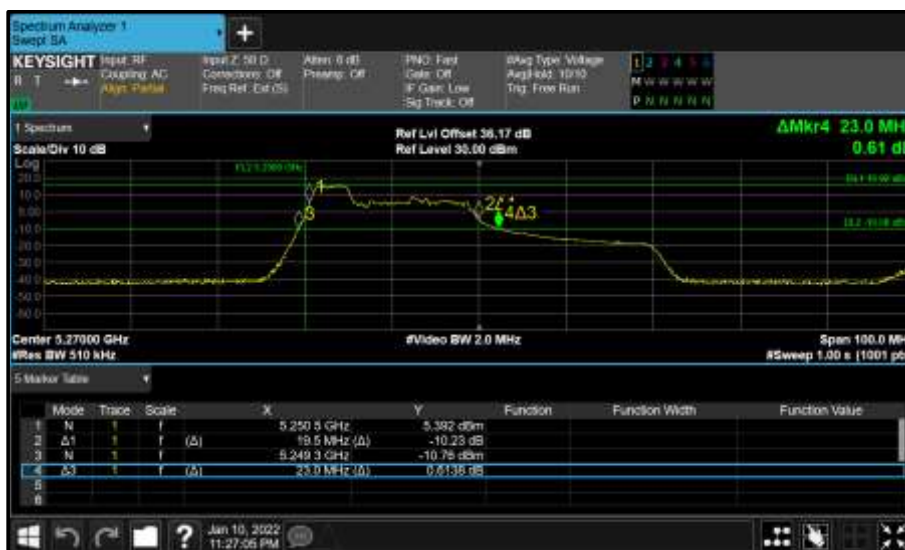
Figure 354 - Core 0 (A) 5270 MHz (CH54) 26 dB and 99% Bandwidth
