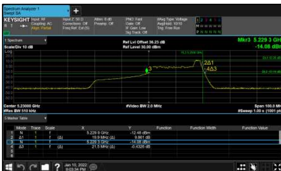
Figure 234 - Core 0 (A) 5230 MHz (CH46) 26 dB and 99% Bandwidth
