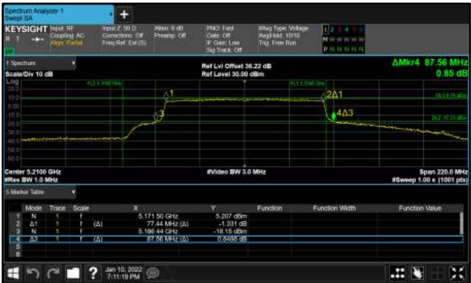
Figure 254 - Core 1 (B) 5210 MHz (CH42) 26 dB and 99% Bandwidth
