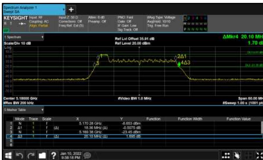
Figure 193 - Core 0 (A) 5180 MHz (CH36) 26 dB and 99% Bandwidth
