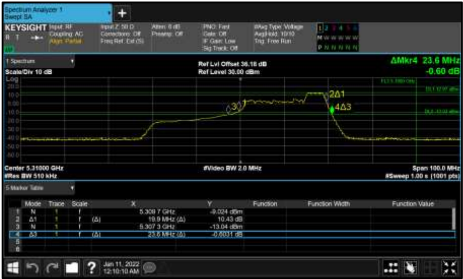
Figure 358 - Core 0 (A) 5310 MHz (CH62) 26 dB and 99% Bandwidth
