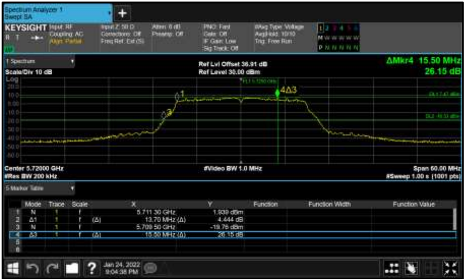
Figure 402 - Core 1 (B) 5720 MHz (CH144) 26 dB and 99% Bandwidth
