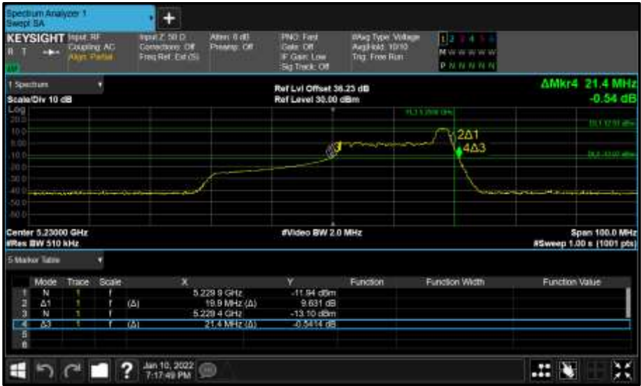
Figure 237 - Core 0 (A) 5230 MHz (CH46) 26 dB and 99% Bandwidth
