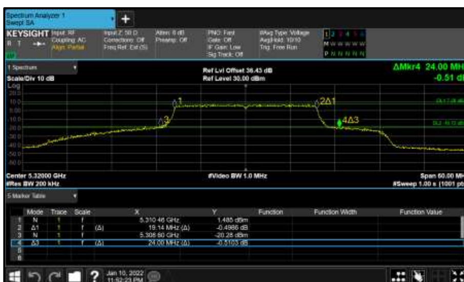
Figure 322 - Core 1 (B) 5320 MHz (CH64) 26 dB and 99% Bandwidth
