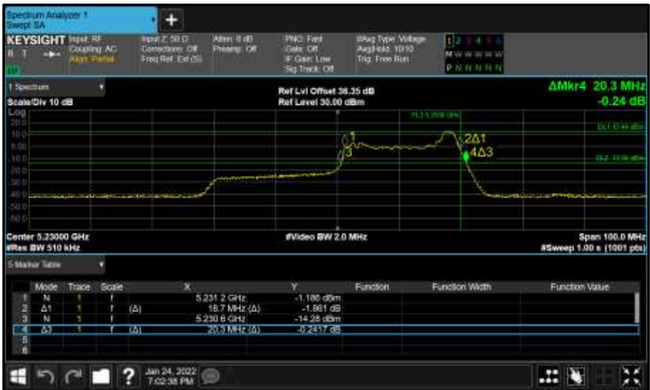
Figure 246 - Core 1 (B) 5230 MHz (CH46) 26 dB and 99% Bandwidth
