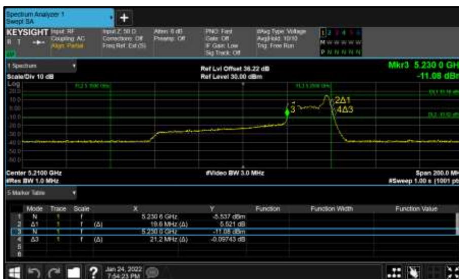
Figure 280 - Core 1 (B) 5210 MHz (CH42) 26 dB and 99% Bandwidth
