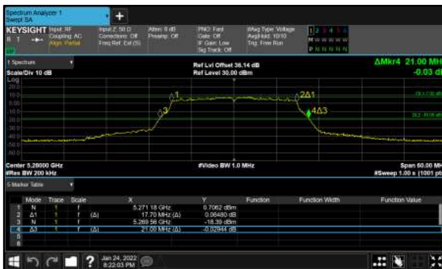
Figure 295 - Core 0 (A) 5280 MHz (CH56) 26 dB and 99% Bandwidth
