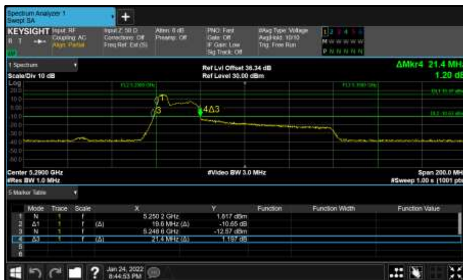
Figure 376 - Core 1 (B) 5290 MHz (CH58) 26 dB and 99% Bandwidth
