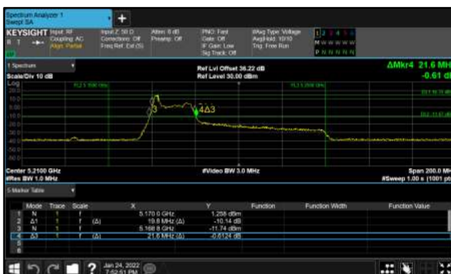
Figure 278 - Core 1 (B) 5210 MHz (CH42) 26 dB and 99% Bandwidth
