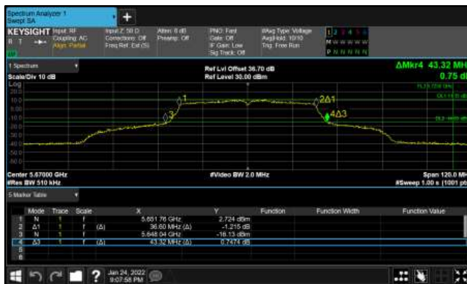
Figure 419 - Core 0 (A) 5670 MHz (CH134) 26 dB and 99% Bandwidth
