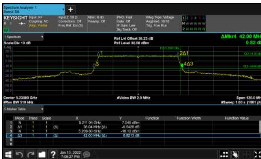
Figure 217 - Core 0 (A) 5230 MHz (CH46) 26 dB and 99% Bandwidth
