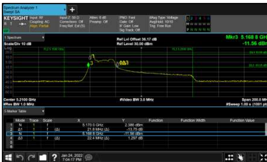
Figure 273 - Core 0 (A) 5210 MHz (CH42) 26 dB and 99% Bandwidth
