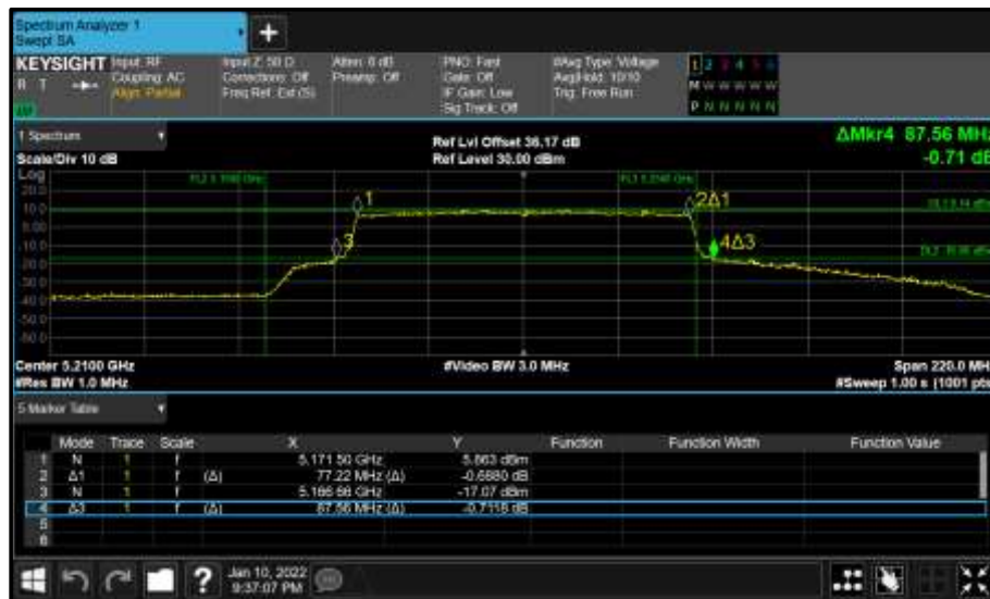
Figure 255 - Core 0 (A) 5210 MHz (CH42) 26 dB and 99% Bandwidth
