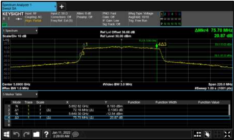
Figure 430 - Core 0 (A) 5690 MHz (CH138) 26 dB and 99% Bandwidth
