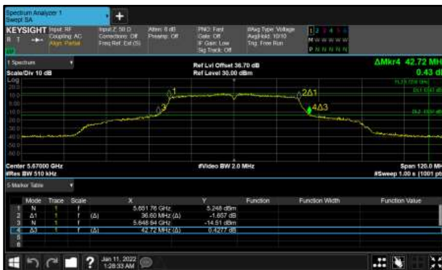
Figure 405 - Core 0 (A) 5670 MHz (CH134) 26 dB and 99% Bandwidth
