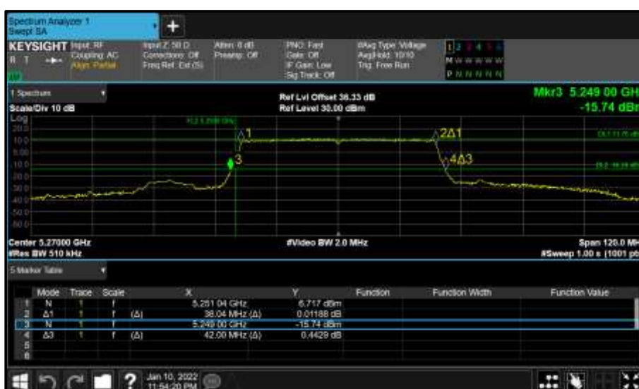
Figure 347 - Core 1 (B) 5270 MHz (CH54) 26 dB and 99% Bandwidth
