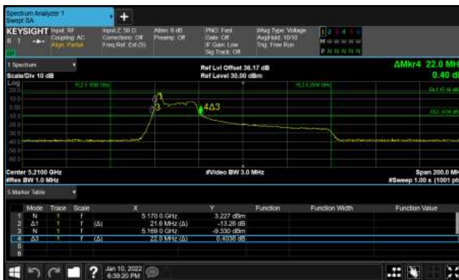
Figure 261 - Core 0 (A) 5210 MHz (CH42) 26 dB and 99% Bandwidth
