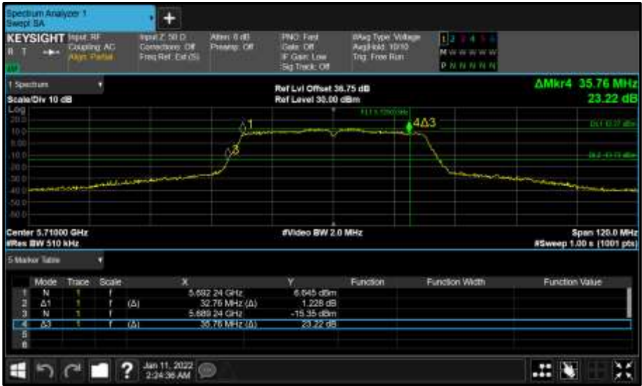
Figure 413 - Core 0 (A) 5710 MHz (CH142) 26 dB and 99% Bandwidth
