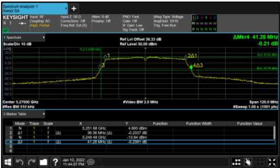
Figure 302 - Core 1 (B) 5270 MHz (CH54) 26 dB and 99% Bandwidth
