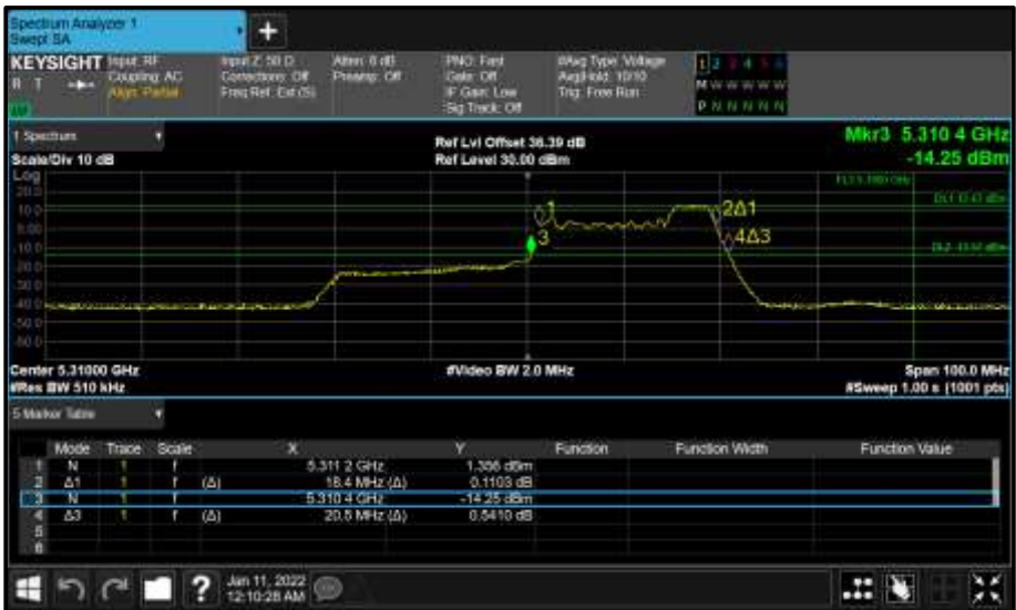
Figure 359 - Core 1 (B) 5310 MHz (CH62) 26 dB and 99% Bandwidth
