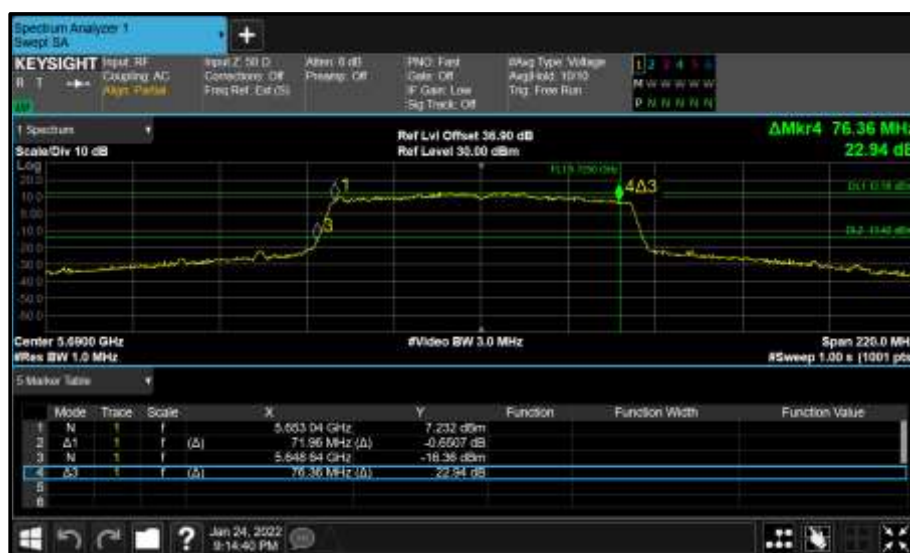
Figure 437 - Core 1 (B) 5690 MHz (CH138) 26 dB and 99% Bandwidth
