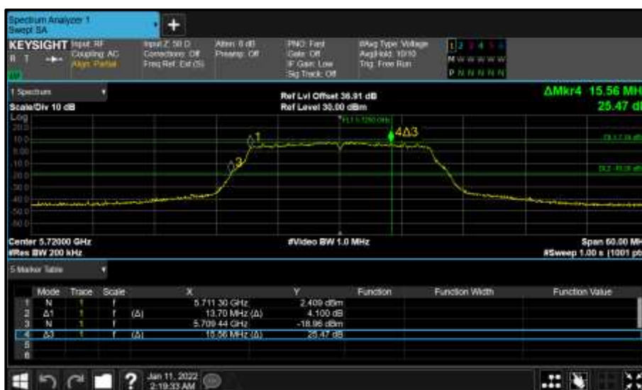
Figure 394 - Core 1 (B) 5720 MHz (CH144) 26 dB and 99% Bandwidth
