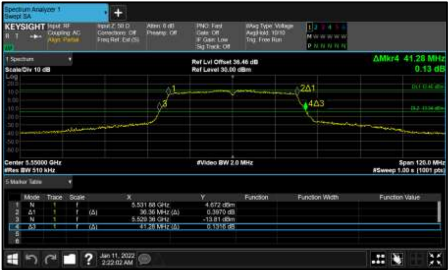
Figure 409 - Core 0 (A) 5550 MHz (CH110) 26 dB and 99% Bandwidth
