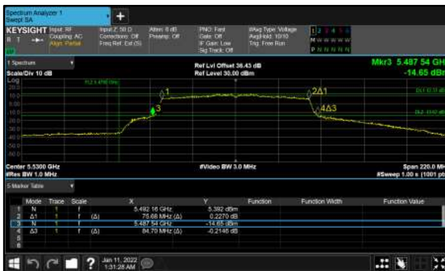
Figure 423 - Core 0 (A) 5530 MHz (CH106) 26 dB and 99% Bandwidth
