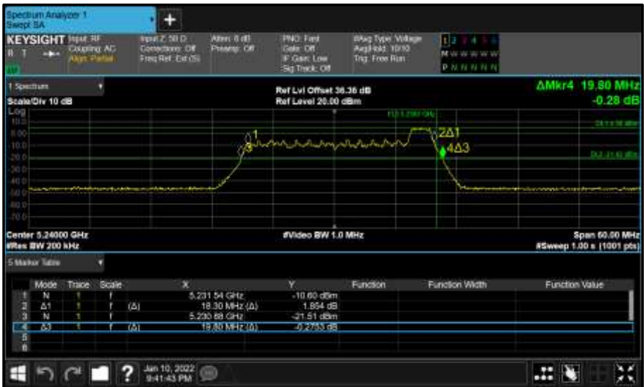
Figure 198 - Core 1 (B) 5240 MHz (CH48) 26 dB and 99% Bandwidth
