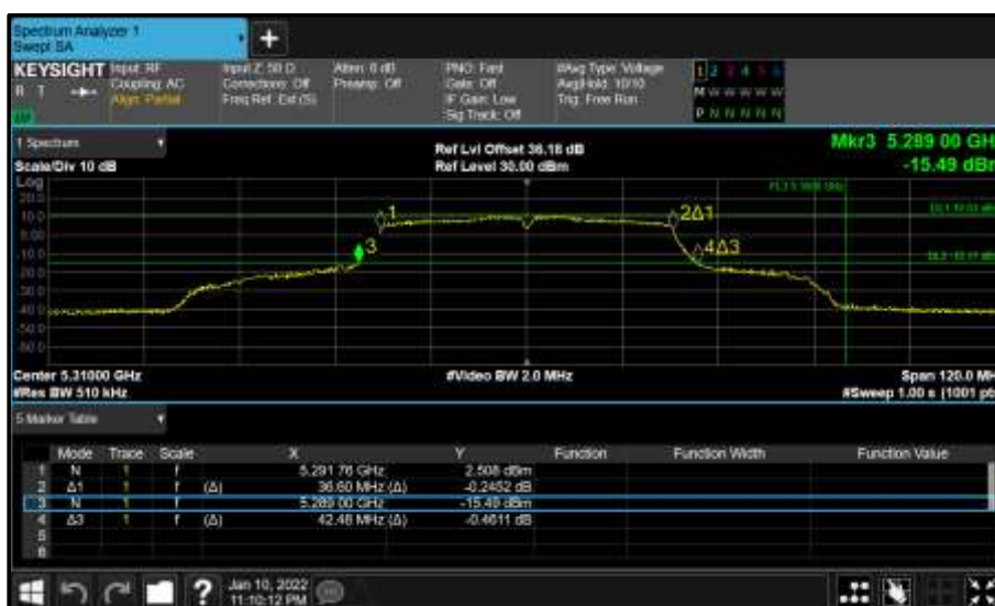
Figure 300 - Core 0 (A) 5310 MHz (CH62) 26 dB and 99% Bandwidth
