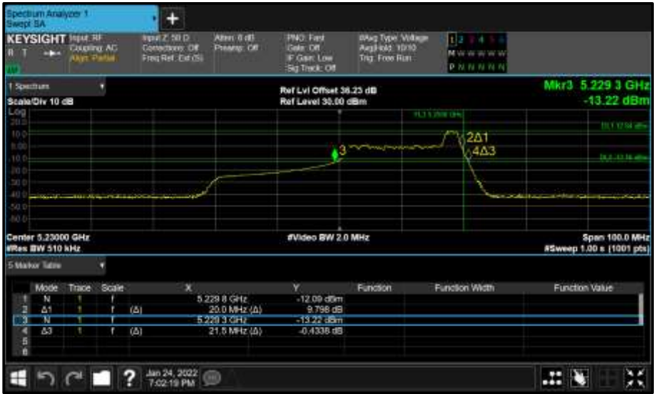
Figure 245 - Core 0 (A) 5230 MHz (CH46) 26 dB and 99% Bandwidth
