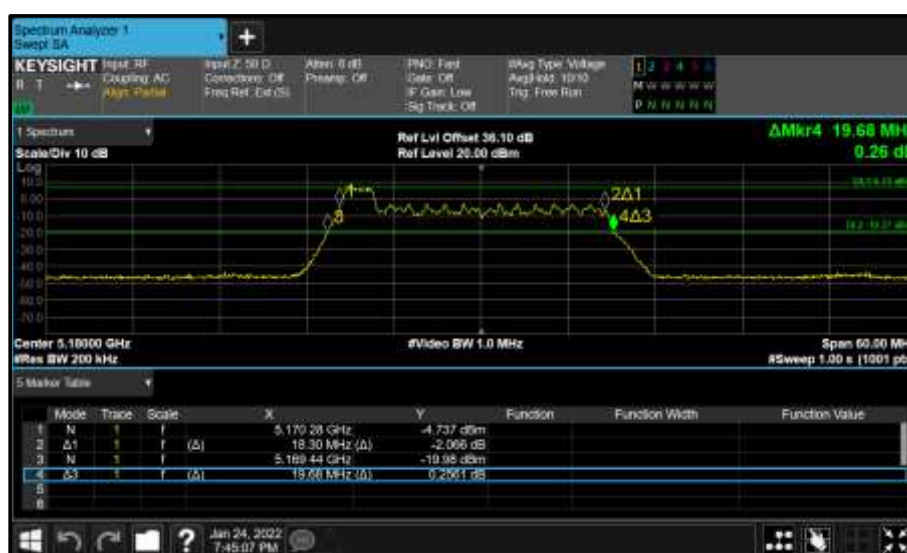
Figure 206 - Core 1 (B) 5180 MHz (CH36) 26 dB and 99% Bandwidth
