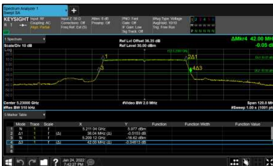
Figure 230 - Core 1 (B) 5230 MHz (CH46) 26 dB and 99% Bandwidth
