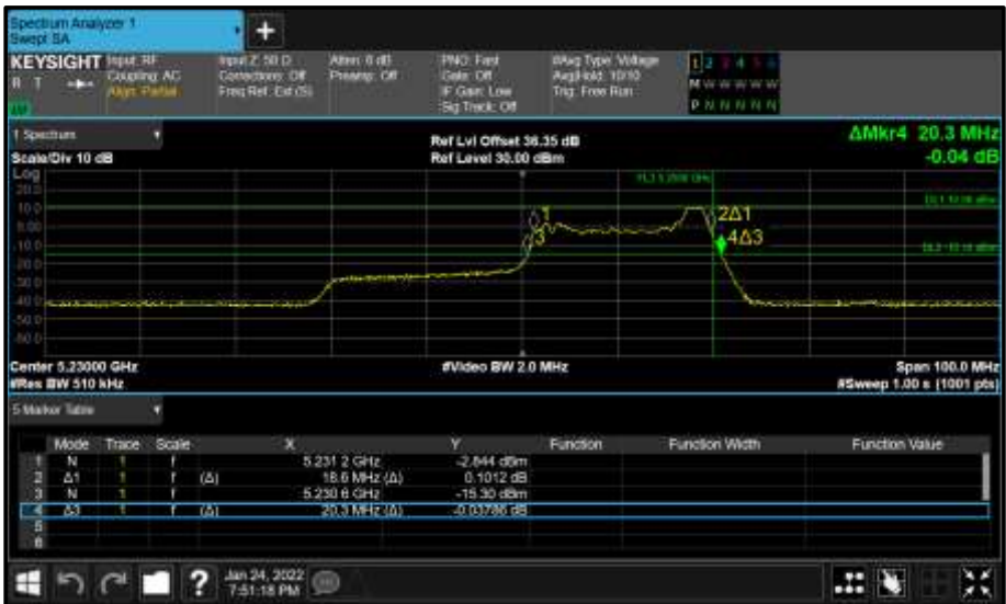
Figure 250 - Core 1 (B) 5230 MHz (CH46) 26 dB and 99% Bandwidth
