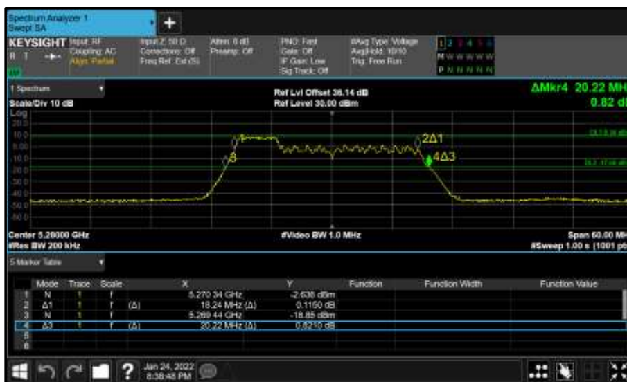
Figure 340 - Core 0 (A) 5280 MHz (CH56) 26 dB and 99% Bandwidth
