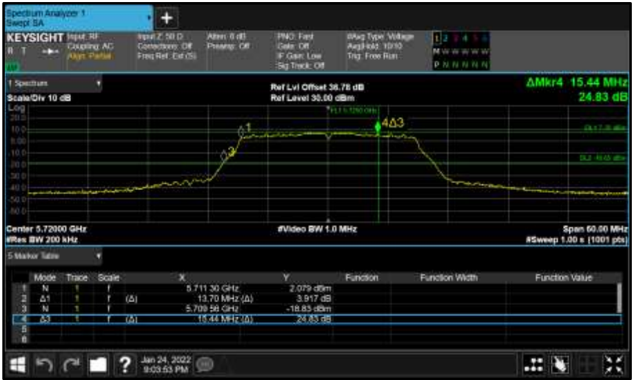
Figure 401 - Core 0 (A) 5720 MHz (CH144) 26 dB and 99% Bandwidth
