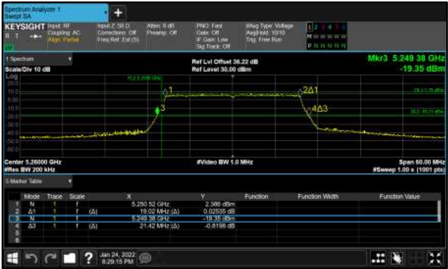
Figure 323 - Core 0 (A) 5260 MHz (CH52) 26 dB and 99% Bandwidth
