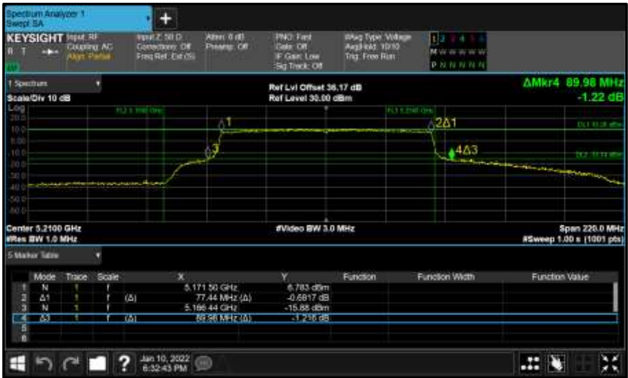
Figure 251 - Core 0 (A) 5210 MHz (CH42) 26 dB and 99% Bandwidth
