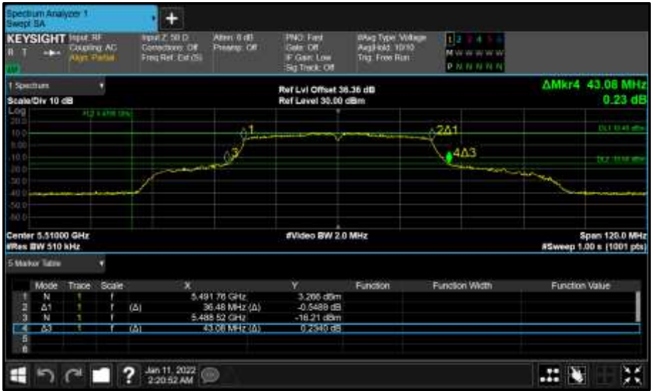
Figure 407 - Core 0 (A) 5510 MHz (CH102) 26 dB and 99% Bandwidth
