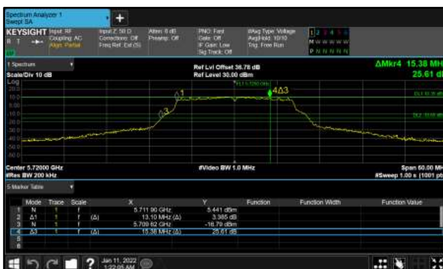
Figure 382 - Core 0 (A) 5720 MHz (CH144) 26 dB and 99% Bandwidth
