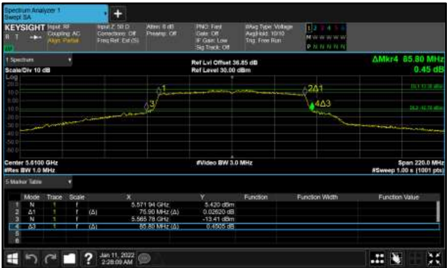
Figure 429 - Core 1 (B) 5610 MHz (CH122) 26 dB and 99% Bandwidth
