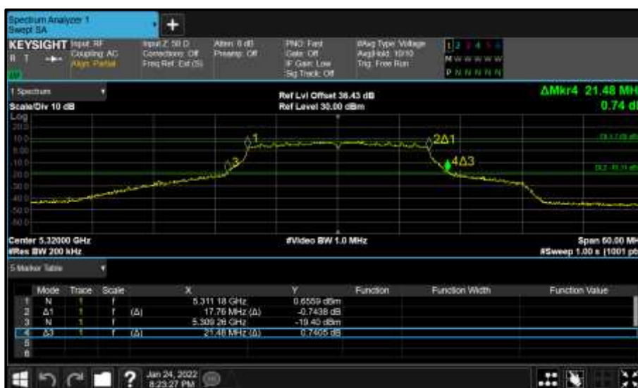
Figure 298 - Core 1 (B) 5320 MHz (CH64) 26 dB and 99% Bandwidth
