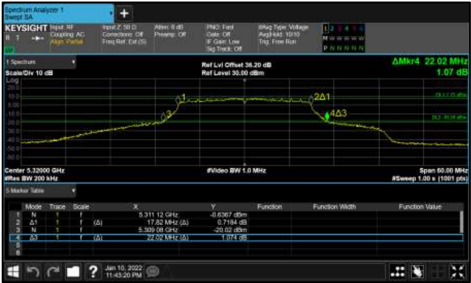
Figure 291 - Core 0 (A) 5320 MHz (CH64) 26 dB and 99% Bandwidth
