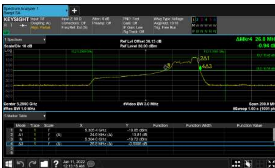
Figure 373 - Core 0 (A) 5290 MHz (CH58) 26 dB and 99% Bandwidth
