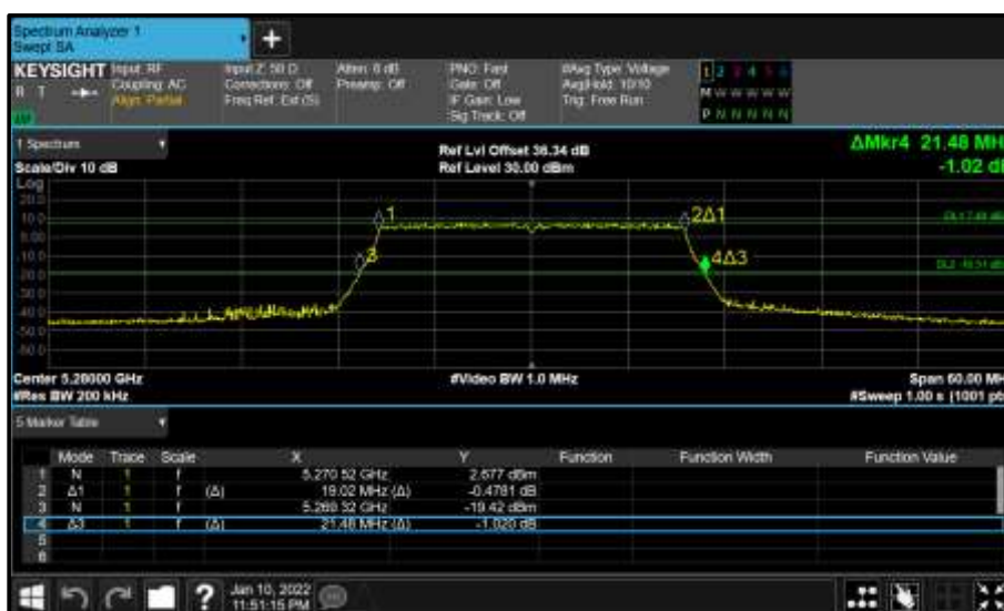
Figure 320 - Core 1 (B) 5280 MHz (CH56) 26 dB and 99% Bandwidth
