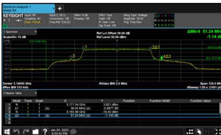
Figure 223 - Core 0 (A) 5190 MHz (CH38) 26 dB and 99% Bandwidth
