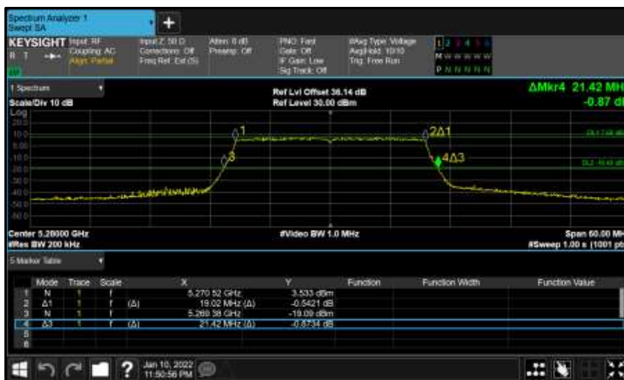
Figure 319 - Core 0 (A) 5280 MHz (CH56) 26 dB and 99% Bandwidth
