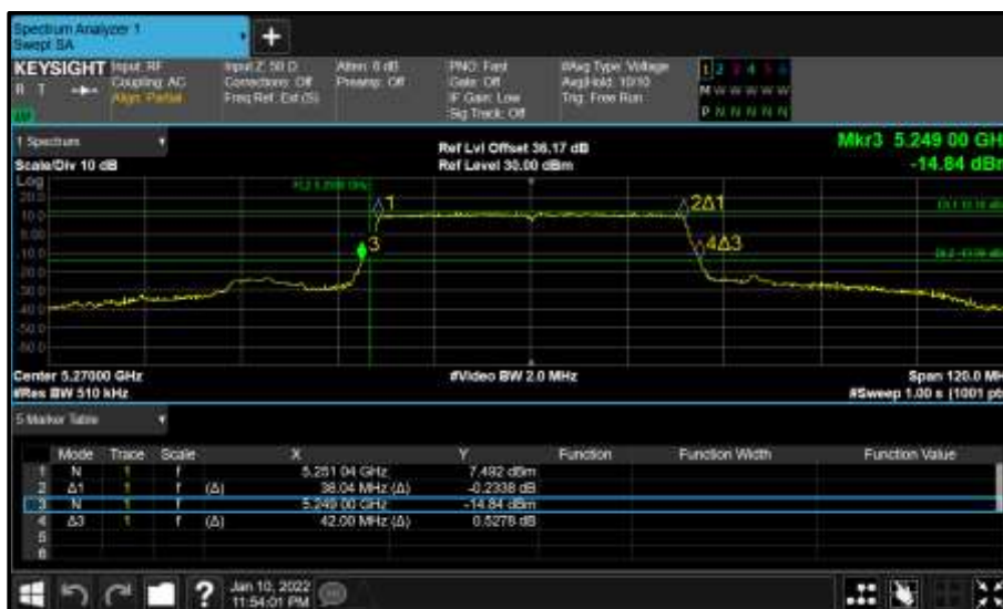
Figure 346 - Core 0 (A) 5270 MHz (CH54) 26 dB and 99% Bandwidth
