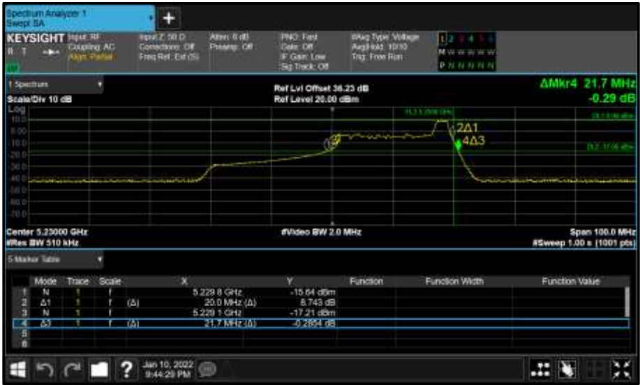
Figure 241 - Core 0 (A) 5230 MHz (CH46) 26 dB and 99% Bandwidth
