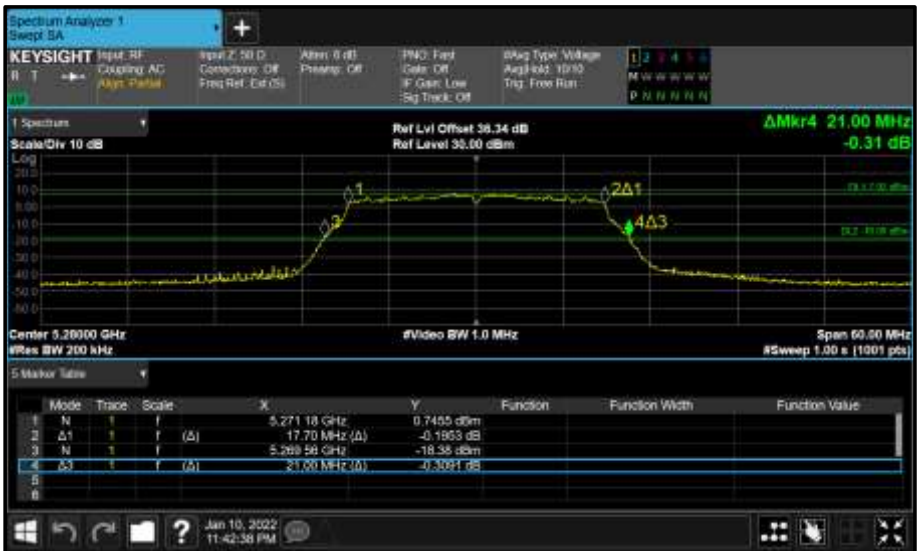
Figure 290 - Core 1 (B) 5280 MHz (CH56) 26 dB and 99% Bandwidth
