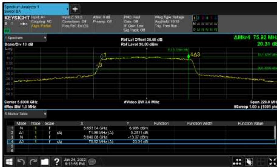
Figure 436 - Core 0 (A) 5690 MHz (CH138) 26 dB and 99% Bandwidth
