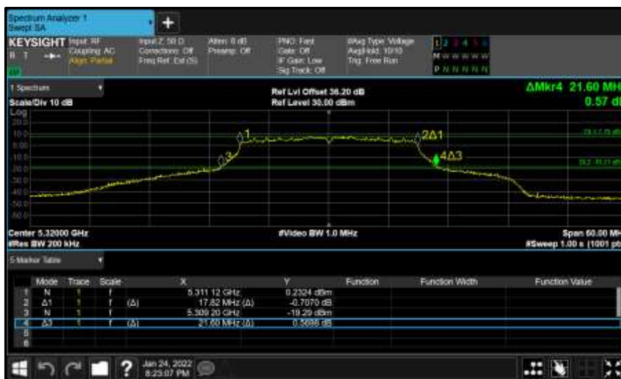
Figure 297 - Core 0 (A) 5320 MHz (CH64) 26 dB and 99% Bandwidth
