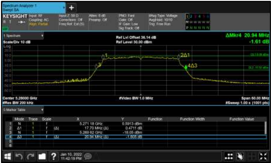
Figure 289 - Core 0 (A) 5280 MHz (CH56) 26 dB and 99% Bandwidth
