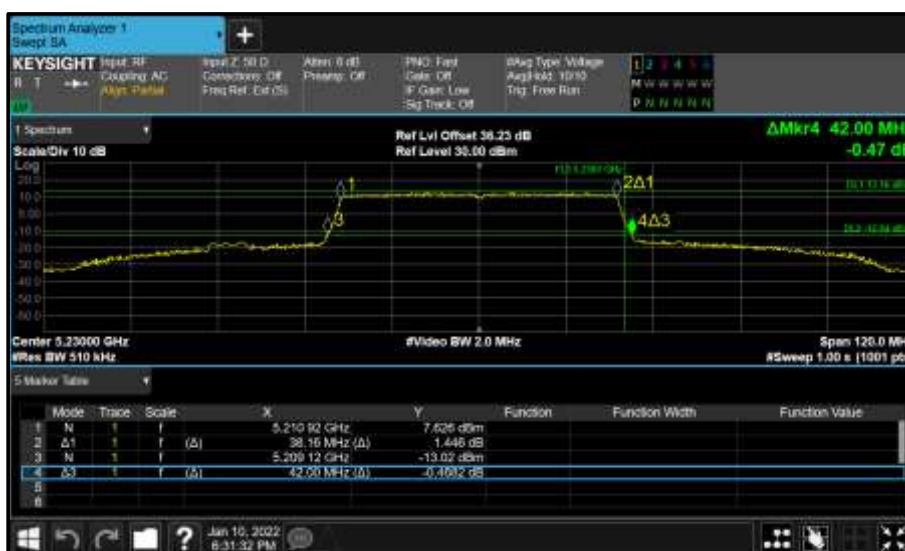
Figure 212 - Core 0 (A) 5230 MHz (CH46) 26 dB and 99% Bandwidth
