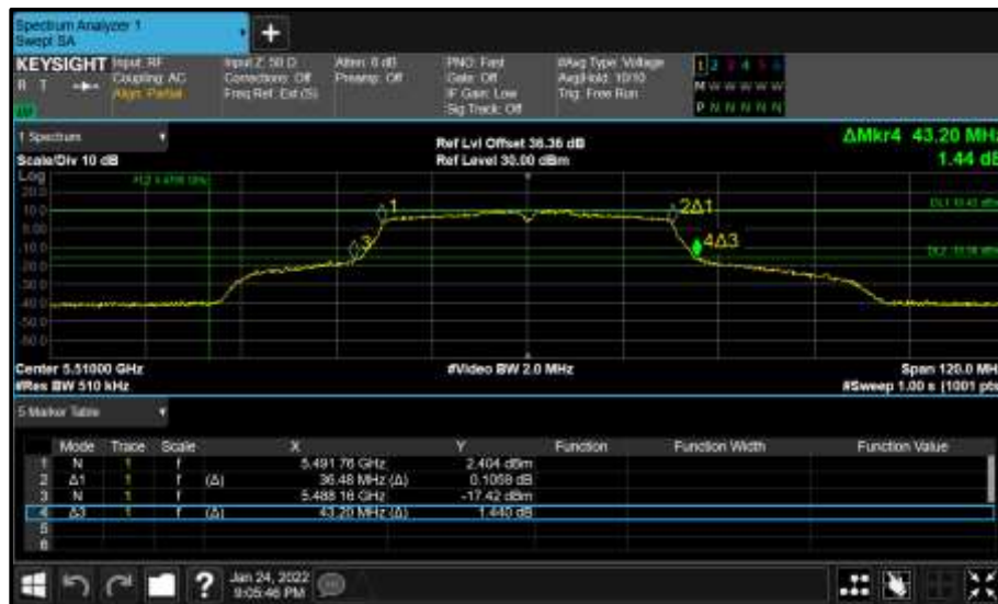
Figure 415 - Core 0 (A) 5510 MHz (CH102) 26 dB and 99% Bandwidth
