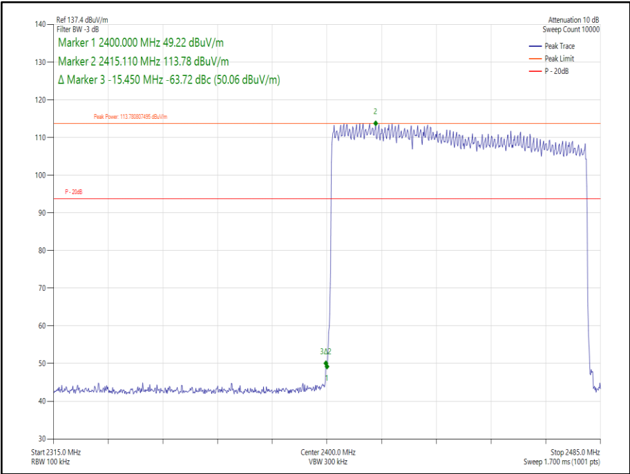
Figure 157 Core 0- Hopping - 8-DPSK/3DH5 - Band Edge Frequency 2400.0 MHz
