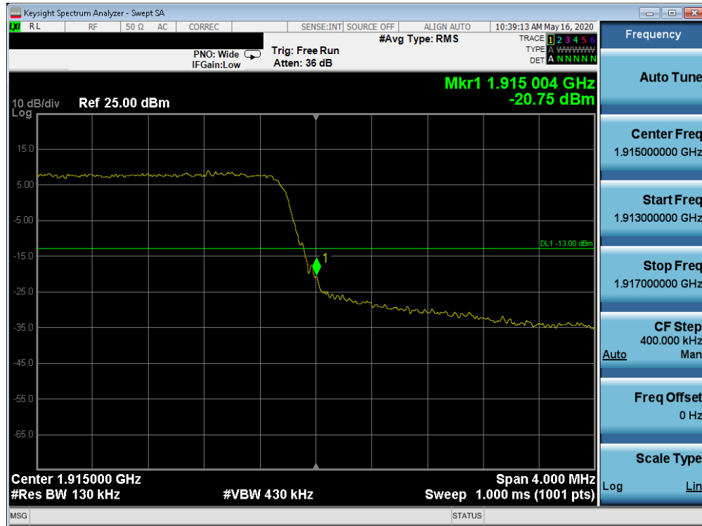
Plot 7-218. Upper Band Edge Plot (Band 25 - 5.0MHz QPSK - Full RB Configuration)
