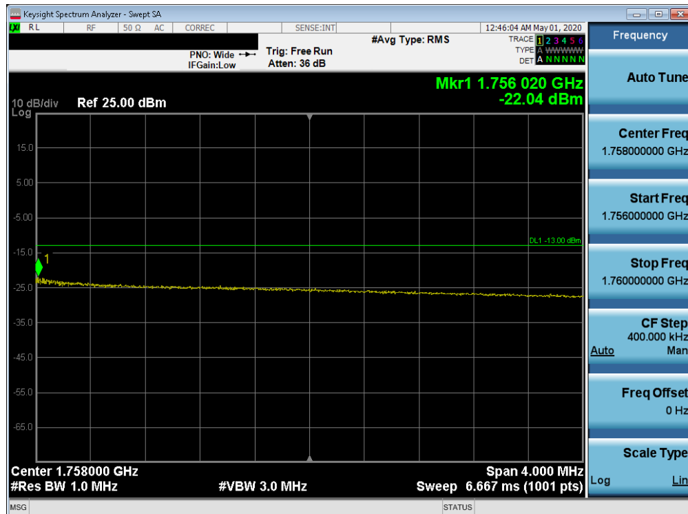
Plot 7-207. Upper Extended Band Edge Plot (Band 4 - 20.0MHz QPSK - Full RB Configuration)
