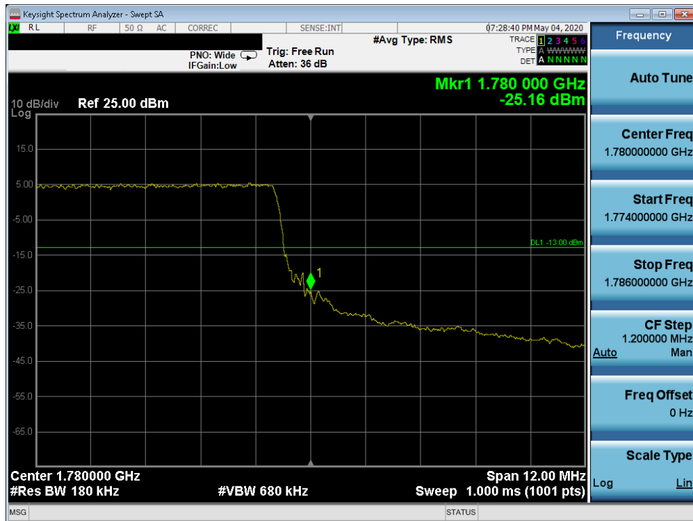
Plot 7-178. Upper Band Edge Plot (Band 66 - 15.0MHz QPSK - Full RB Configuration)
