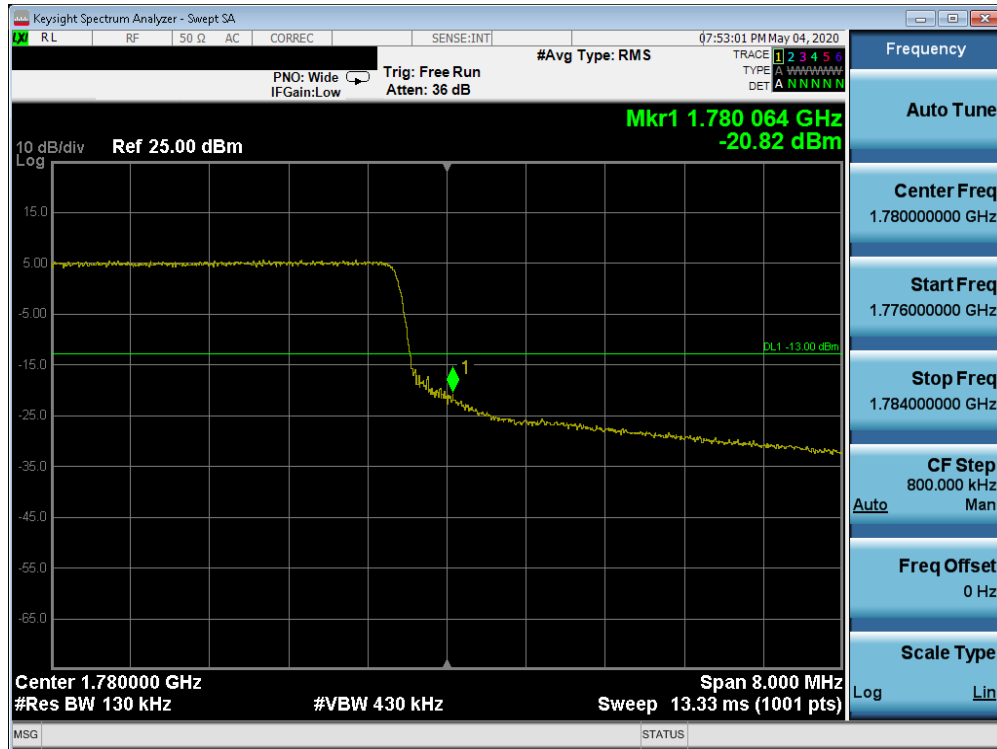
Plot 7-174. Upper Band Edge Plot (Band 66 - 10.0MHz QPSK - Full RB Configuration)
