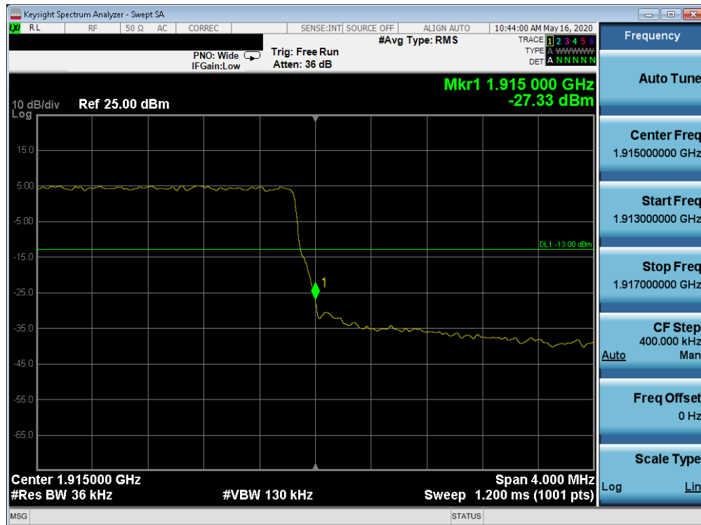
Plot 7-214. Upper Band Edge Plot (Band 25 - 3.0MHz QPSK - Full RB Configuration)
