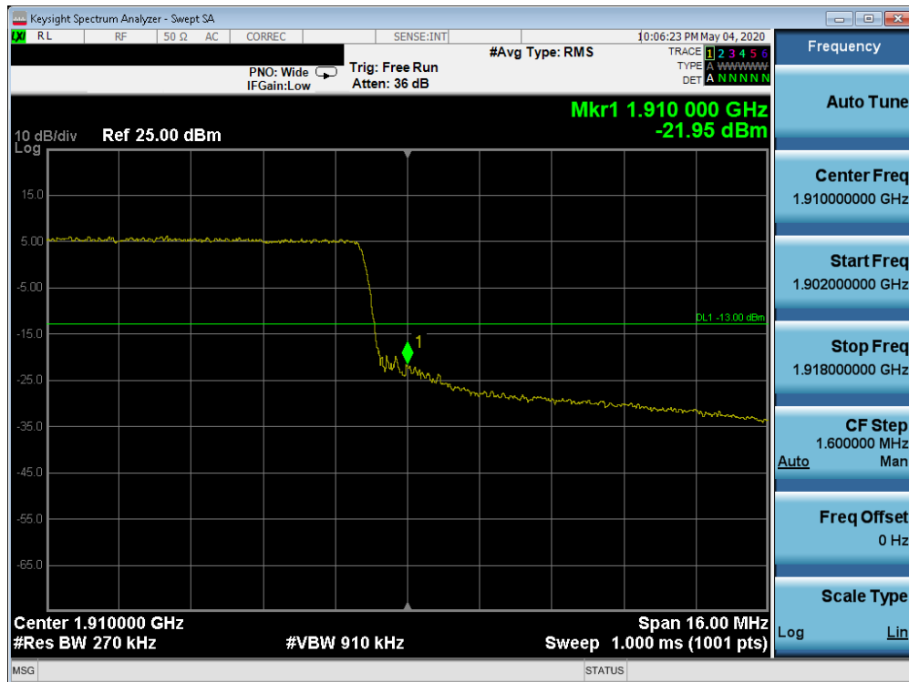
Plot 7-254. Upper Band Edge Plot (Band 2 - 20.0MHz QPSK - Full RB Configuration)
