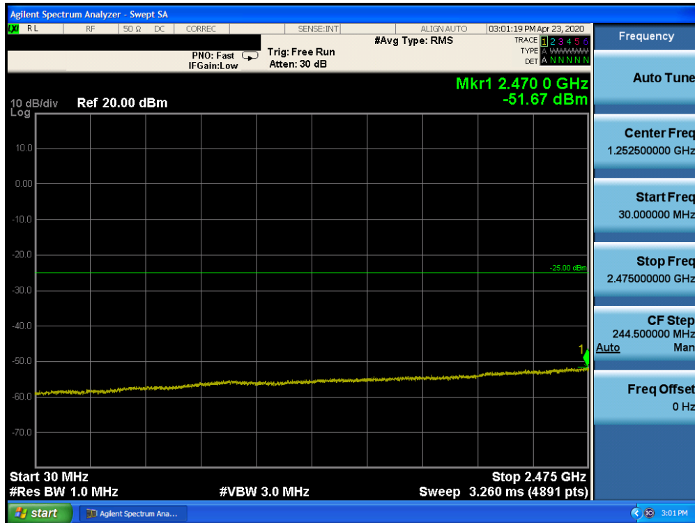
Plot 7-106. Conducted Spurious Plot (Band 7 - 20.0MHz QPSK - RB Size 1, RB Offset 0 - Low Channel)
