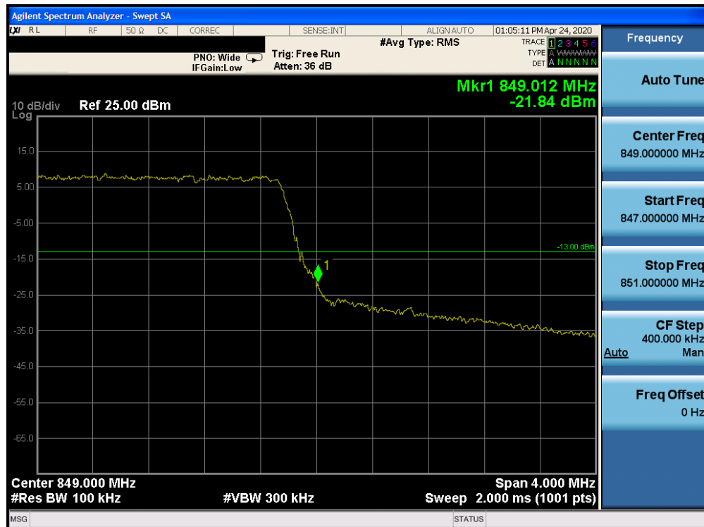
Plot 7-157. Upper Band Edge Plot (Band 5 - 5.0MHz QPSK - Full RB Configuration)
