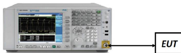
Figure 7-5. Test Instrument & Measurement Setup
