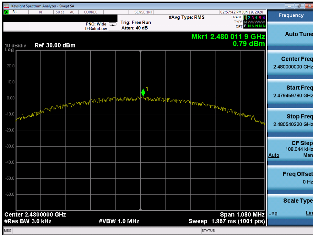
Plot 7-9. Power Spectral Density Plot (Bluetooth (LE), 1Mbps, ePA – Ch. 39)
