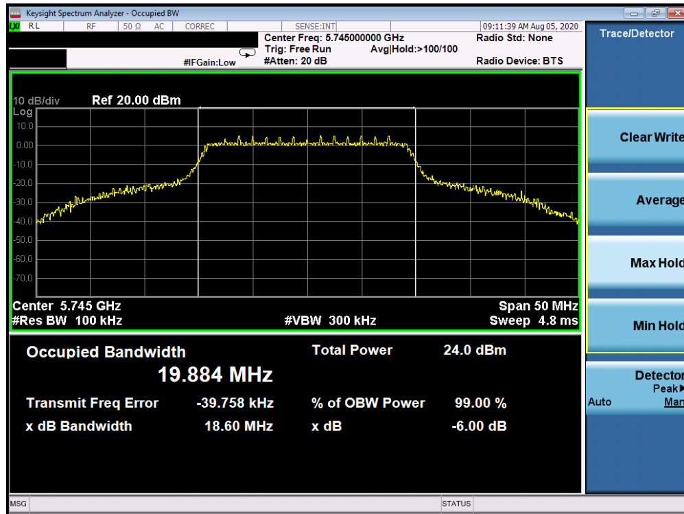
Plot 7-10. 6dB Bandwidth Plot (20MHz BW 802.11n (UNII Band 3) – Ch. 149)
