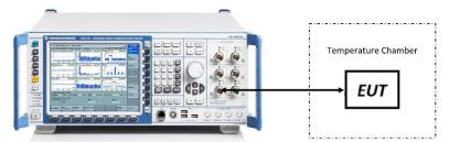
Figure 7-8. Test Instrument & Measurement Setup
