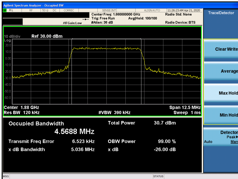
Plot 7-38. Occupied Bandwidth Plot (Band 25/2 - 5.0MHz 16-QAM - Full RB Configuration)
