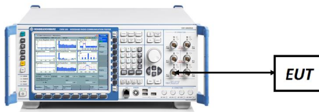
Figure 7-5. ERP/EIRP Measurement Setup
