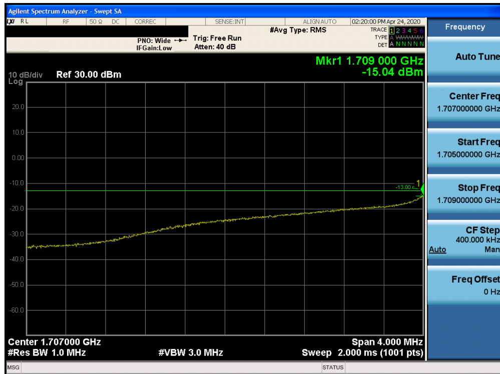
Plot 7-34. 4MHz Span Plot (AWS WCDMA Mode - Low Channel)
