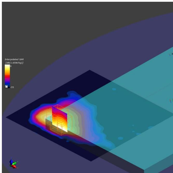
**11. LTE Band 41, QPSK - 20MHz, CH39750, Main Antenna – Back face**
