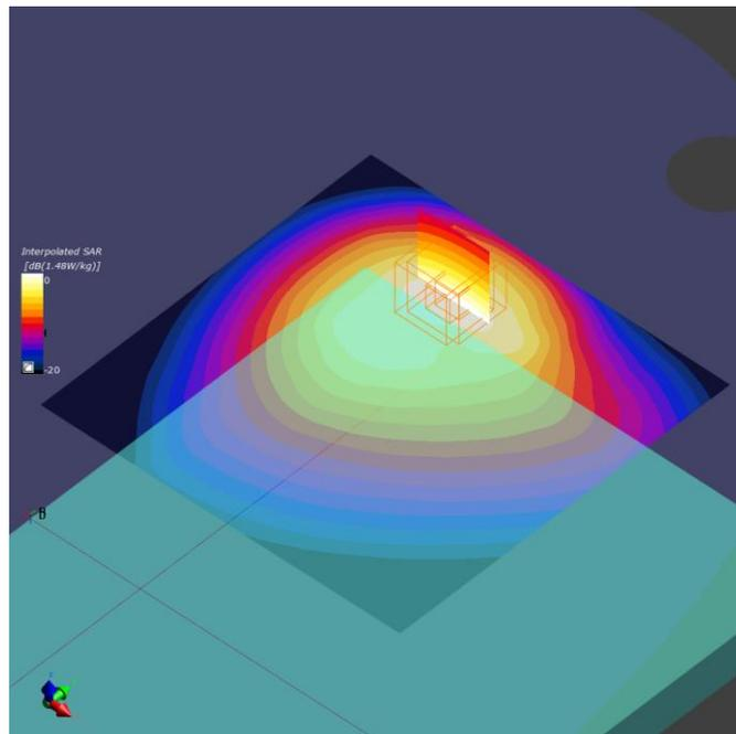
**8. LTE Band 26, QPSK - 15MHz, CH26775, Main Antenna – Laptop**
