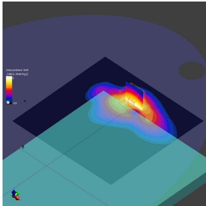
**10. LTE Band 38, QPSK - 20MHz, CH38000, Main Antenna – Back Face**
