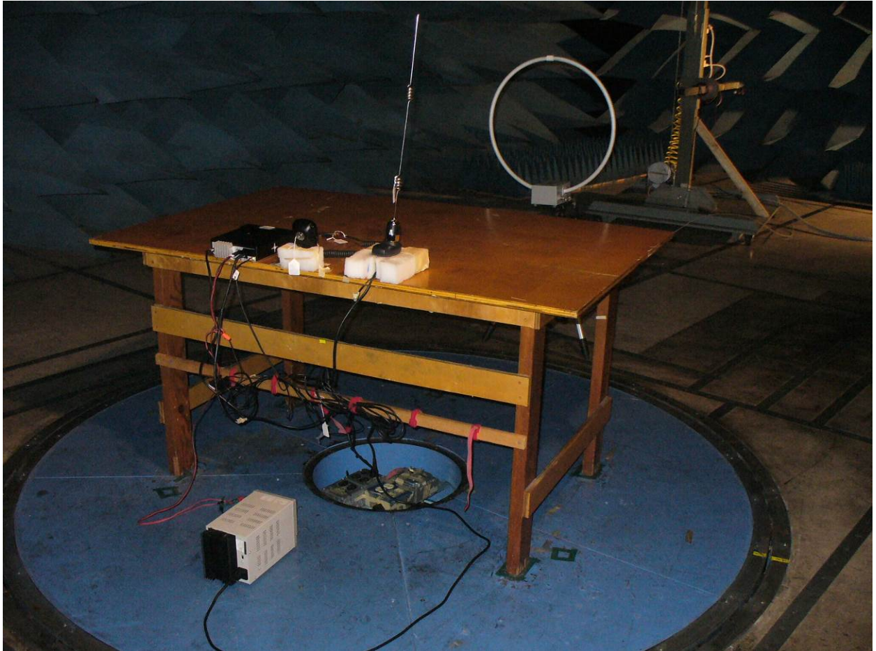
Figure 2: Radiated Emissions – Back View (Below 30 MHz)
