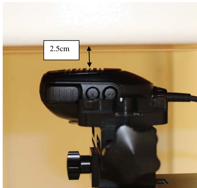
Test Position - Speaker Microphone 2.5cm from phantom
