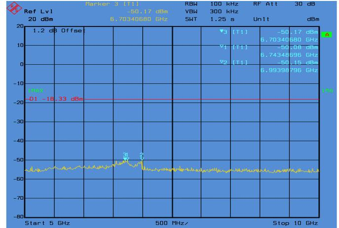
Conducted Emissions. 802.11g, Frequency 2412 MHz Emission Level, 5 GHz -> 10 GHz
