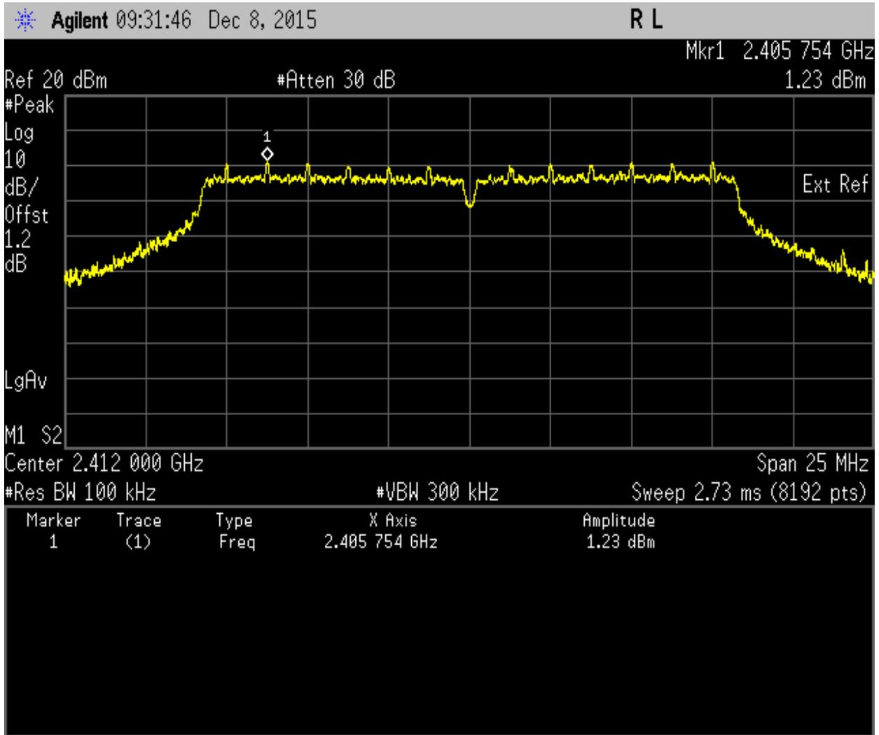
**Maximum Peak Power Spectral Density. 802.11g Frequency 2412 MHz**
