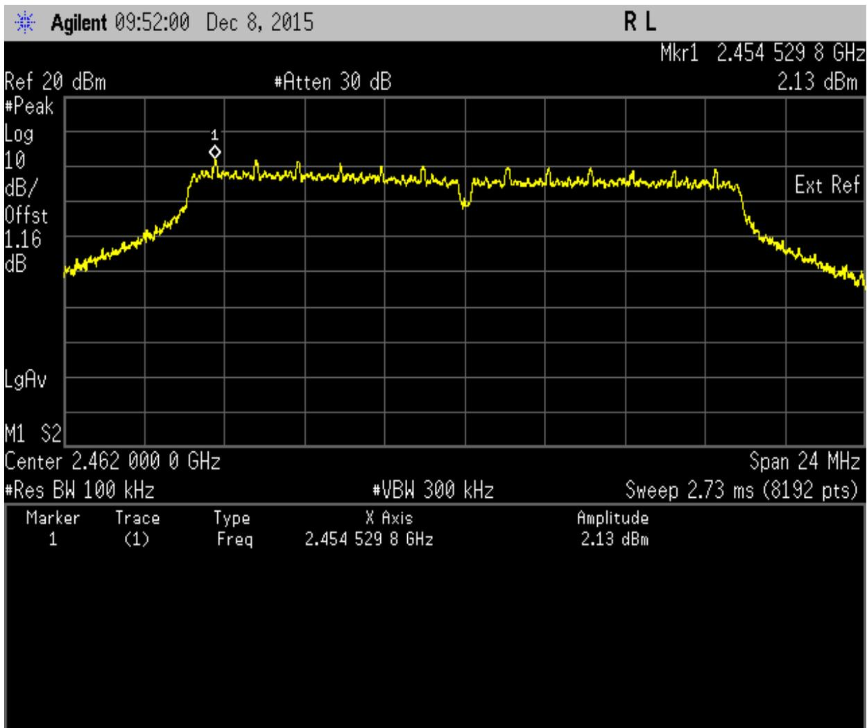
**Maximum Peak Power Spectral Density. 802.11g Frequency 2462 MHz**
