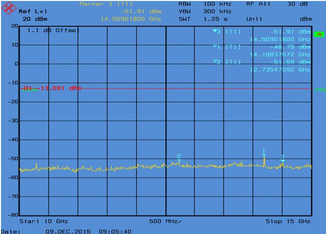
Conducted Emissions. 802.11b, Frequency 2437 MHz Emission Level, 10 GHz -> 15 GHz
