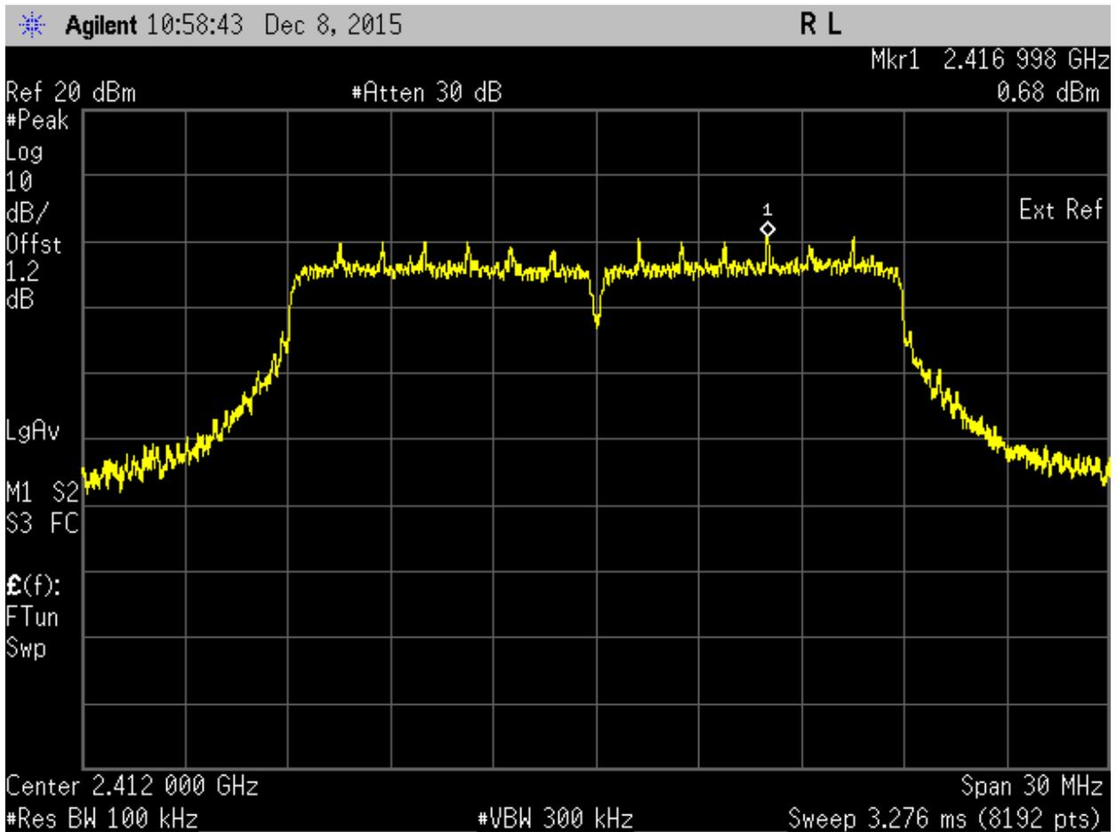
Band Edge (100 kHz). 802.11n\_20 Frequency 2412 MHz Reference Level
