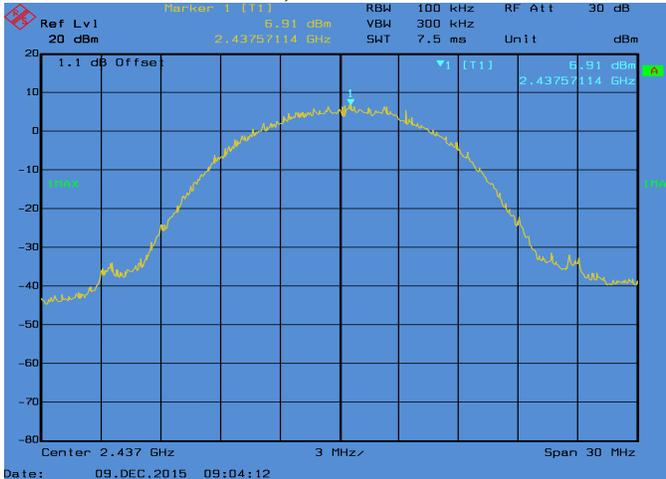
**Conducted Emissions. 802.11b, Frequency 2437 MHz Reference Level**
