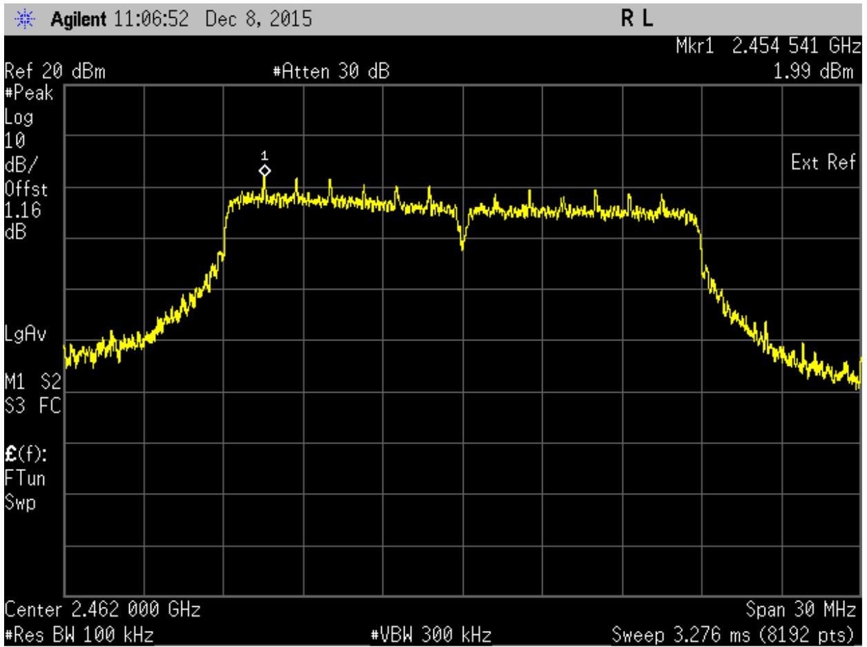
Band Edge (100 kHz). 802.11n\_20 Frequency 2462 MHz Reference Level
