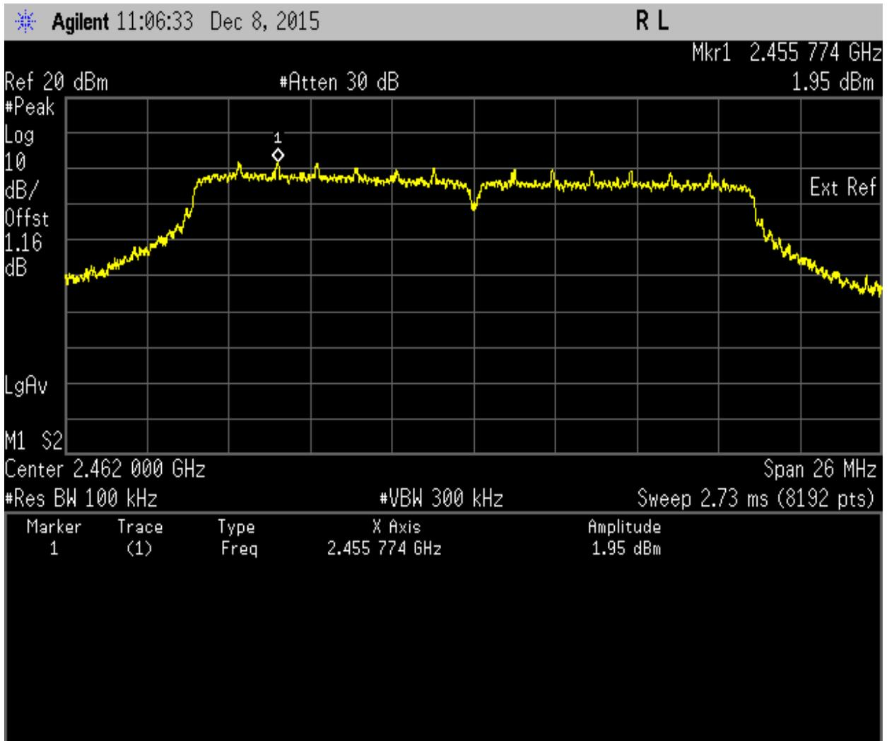
Maximum Peak Power Spectral Density. 802.11n\_20 Frequency 2462 MHz
