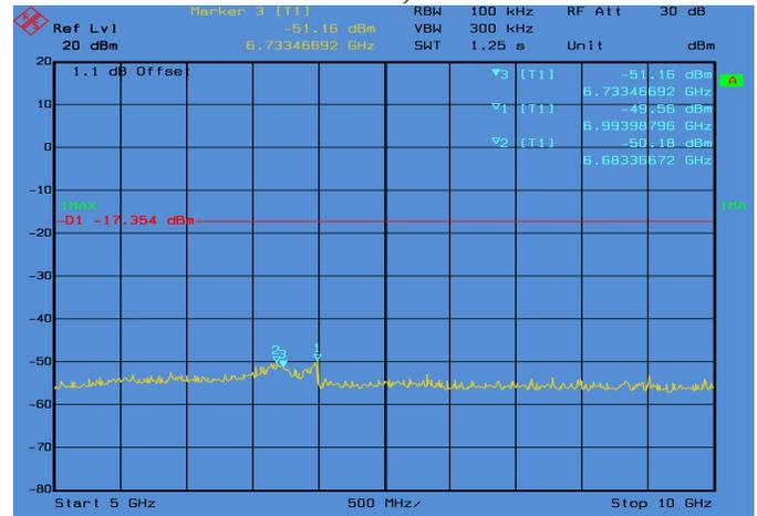
Conducted Emissions. 802.11n\_20, Frequency 2437 MHz Emission Level, 5 GHz -> 10 GHz
