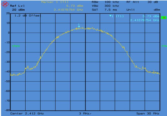
**Conducted Emissions. 802.11b, Frequency 2412 MHz Reference Level**
