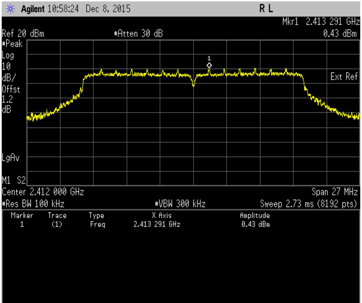
Maximum Peak Power Spectral Density. 802.11n\_20 Frequency 2412 MHz
