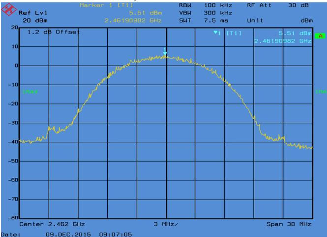
Conducted Emissions. 802.11b, Frequency 2462 MHz Reference Level
