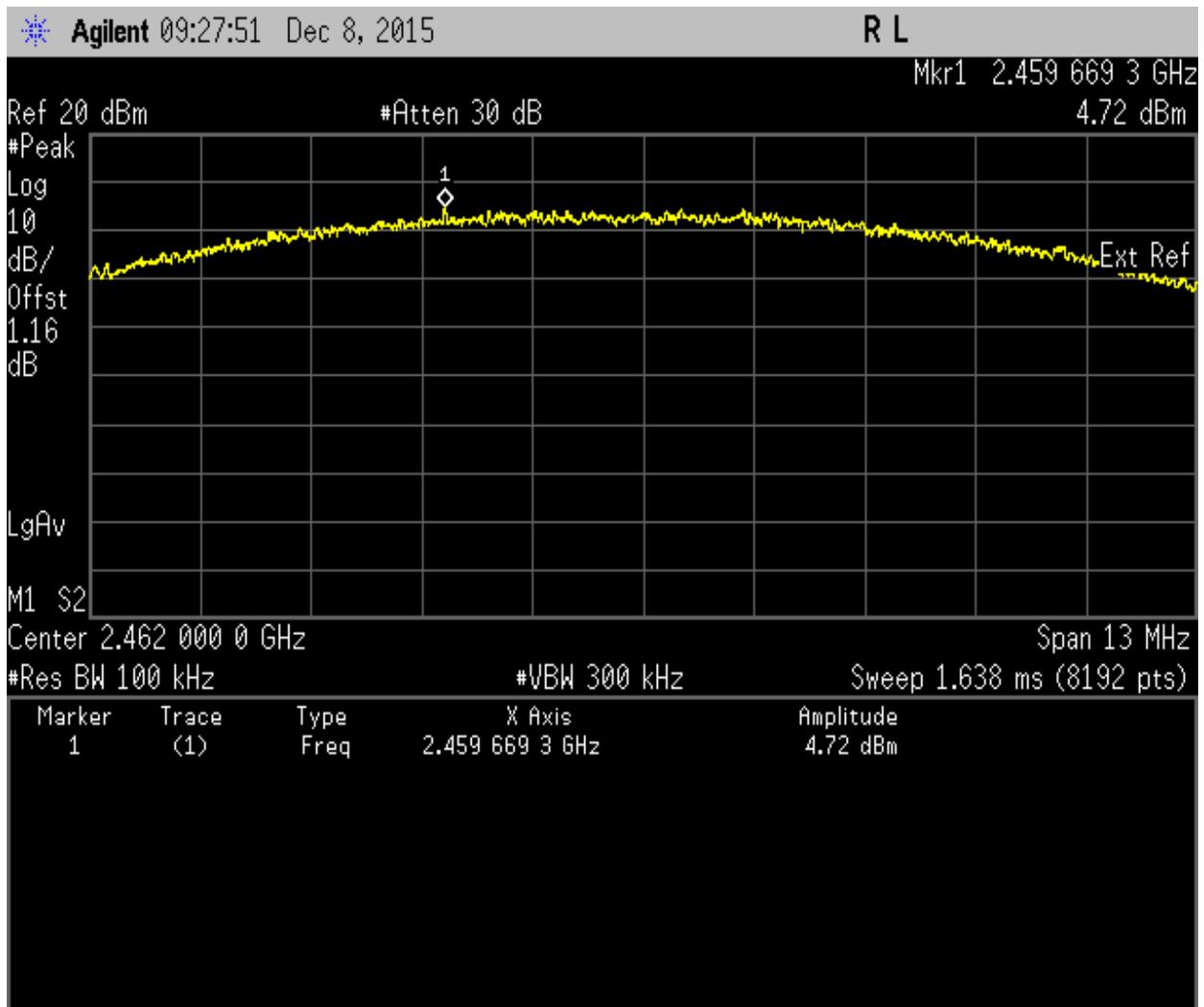
**Maximum Peak Power Spectral Density. 802.11b Frequency 2462 MHz**
