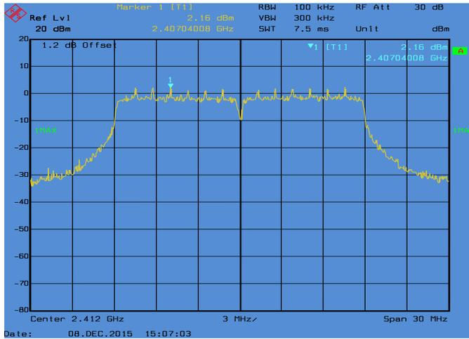
**Conducted Emissions. 802.11n\_20, Frequency 2412 MHz Reference Level**
