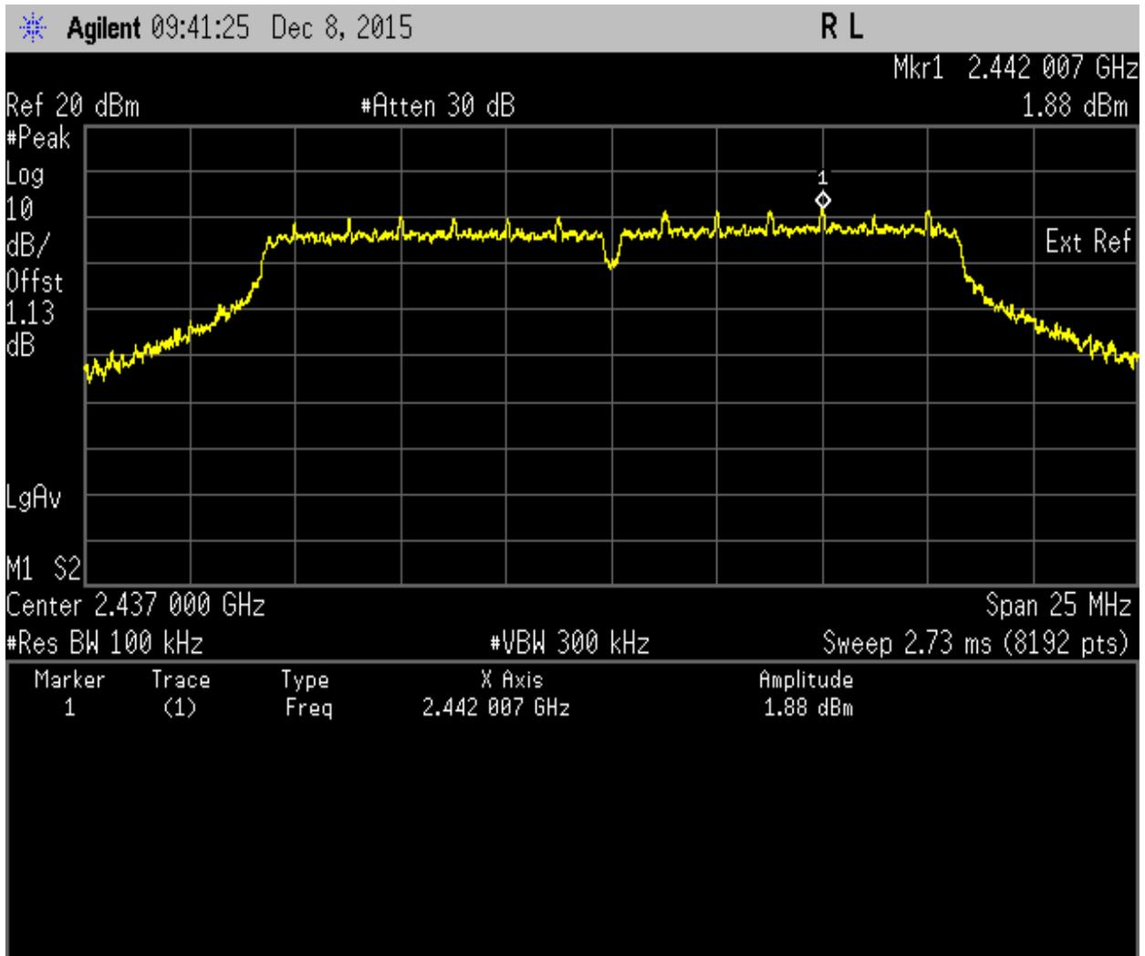
Maximum Peak Power Spectral Density. 802.11g Frequency 2437 MHz
