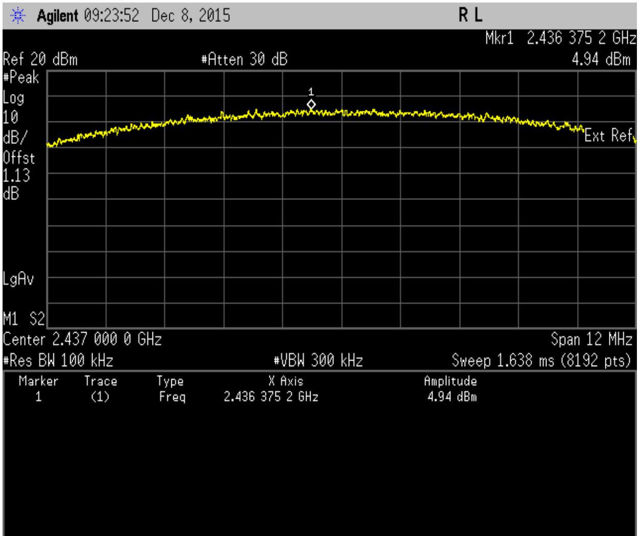
Maximum Peak Power Spectral Density. 802.11b Frequency 2437 MHz
