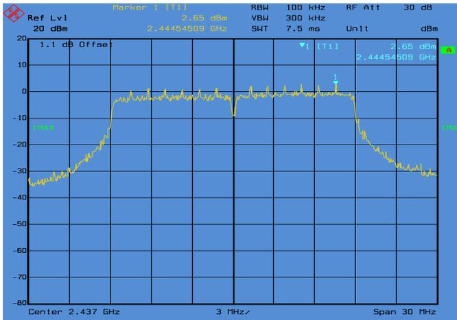
Conducted Emissions. 802.11n\_20, Frequency 2437 MHz Reference Level
