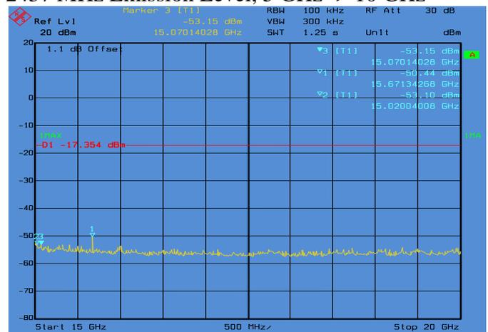
Conducted Emissions. 802.11n\_20, Frequency 2437 MHz Emission Level, 15 GHz -> 20 GHz
