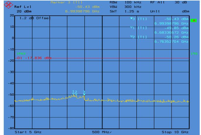
**Conducted Emissions. 802.11n\_20, Frequency 2412 MHz Emission Level, 5 GHz -> 10 GHz**
