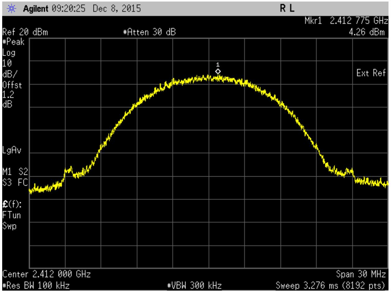
Band Edge (100 kHz). 802.11b Frequency 2412 MHz Reference Level
