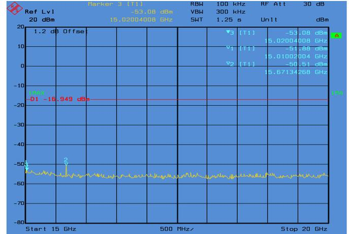
**Conducted Emissions. 802.11g, Frequency 2462 MHz Emission Level, 15 GHz -> 20 GHz**
