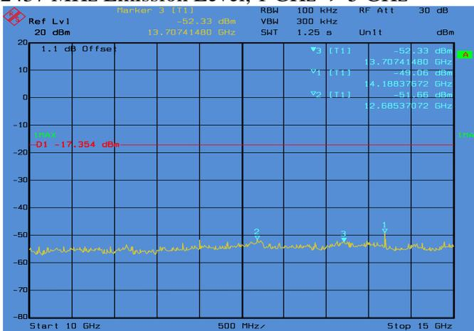
Conducted Emissions. 802.11n\_20, Frequency 2437 MHz Emission Level, 10 GHz -> 15 GHz
