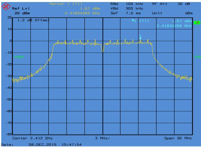
**Conducted Emissions. 802.11g, Frequency 2412 MHz Reference Level**
