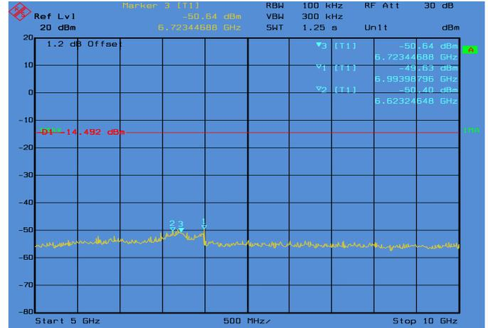
**Conducted Emissions. 802.11b, Frequency 2462 MHz Emission Level, 5 GHz -> 10 GHz**
