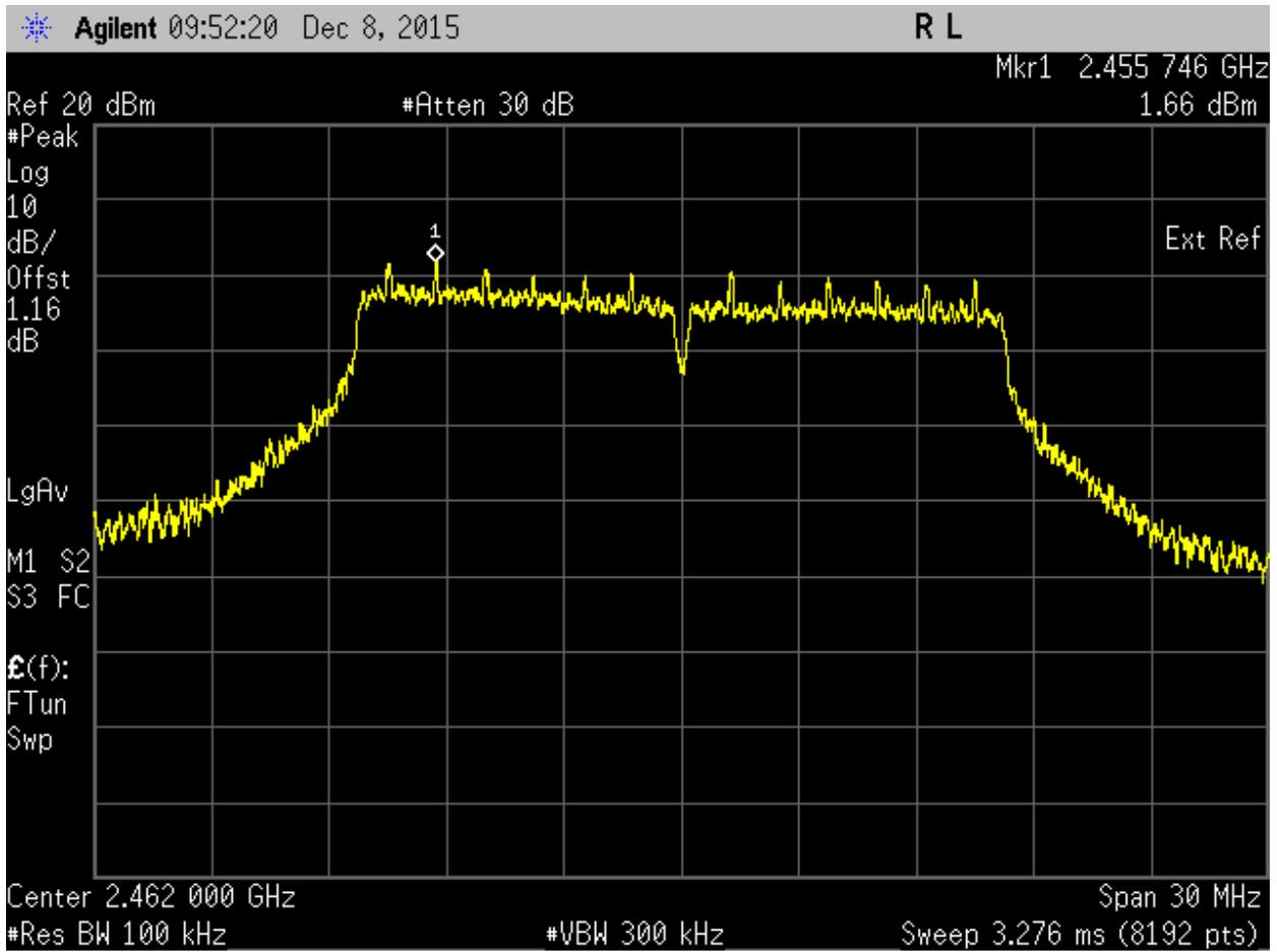
Band Edge (100 kHz). 802.11g Frequency 2462 MHz Reference Level
