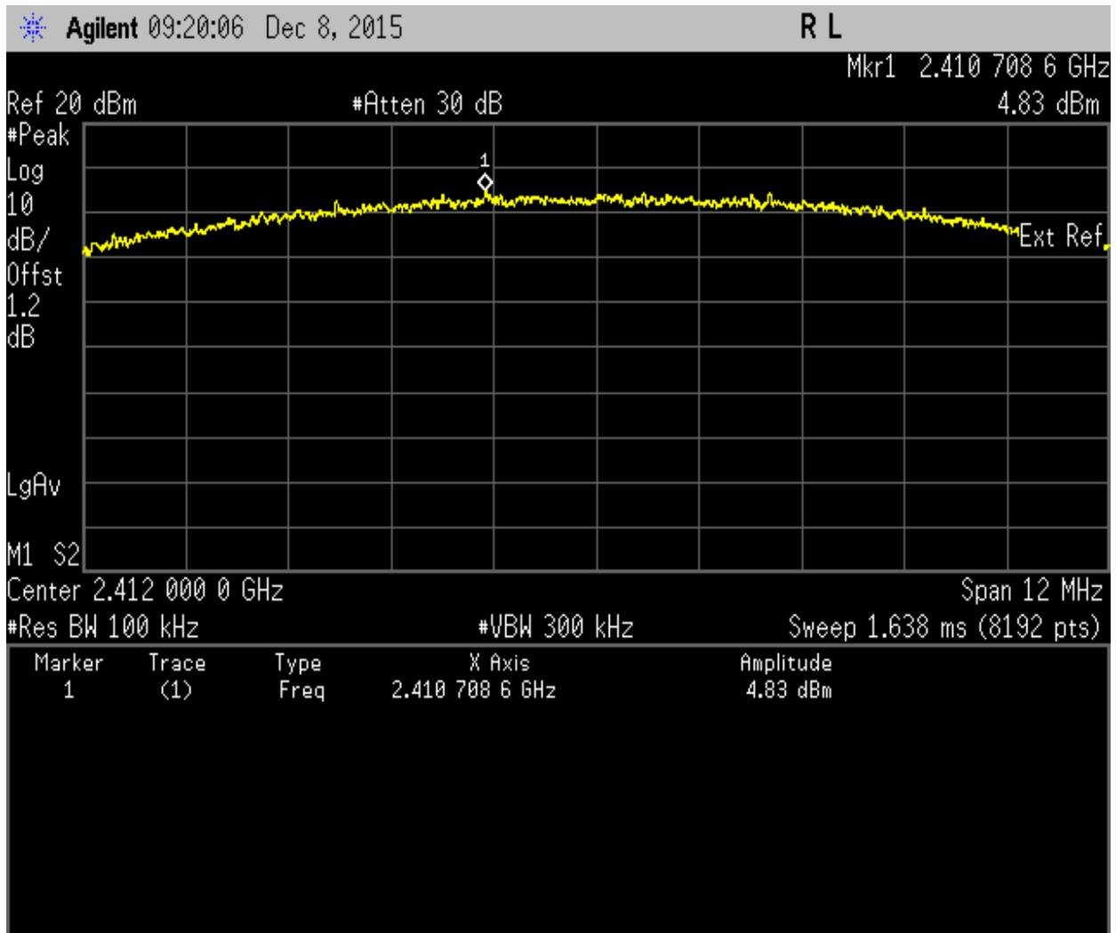
**Maximum Peak Power Spectral Density. 802.11b Frequency 2412 MHz**
