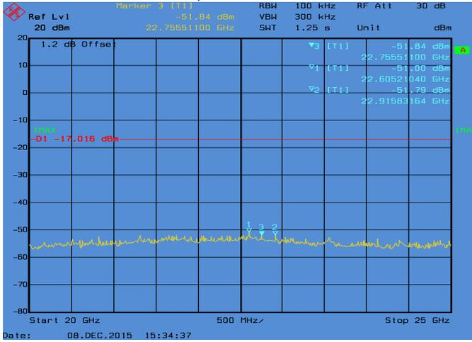
**Conducted Emissions. 802.11n\_20, Frequency 2462 MHz Emission Level, 20 GHz -> 25 GHz**
