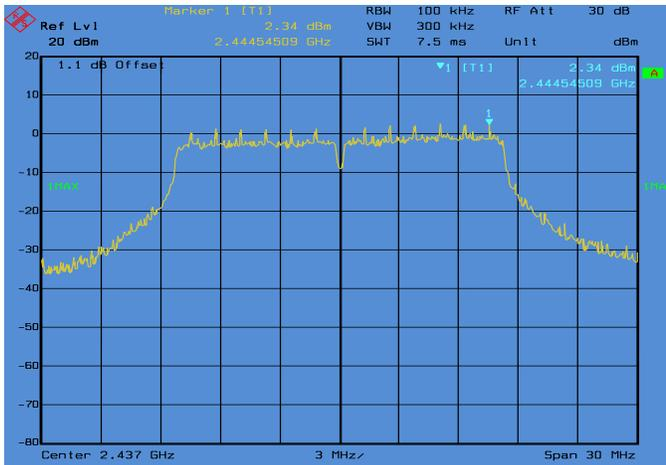
Conducted Emissions. 802.11g, Frequency 2437 MHz Reference Level
