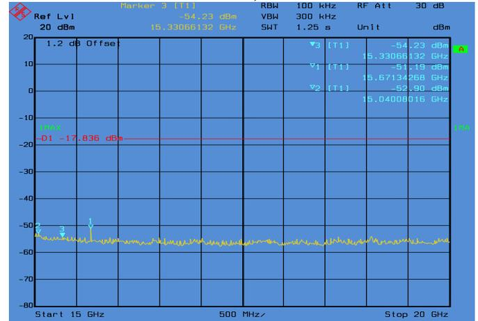
**Conducted Emissions. 802.11n\_20, Frequency 2412 MHz Emission Level, 15 GHz -> 20 GHz**
