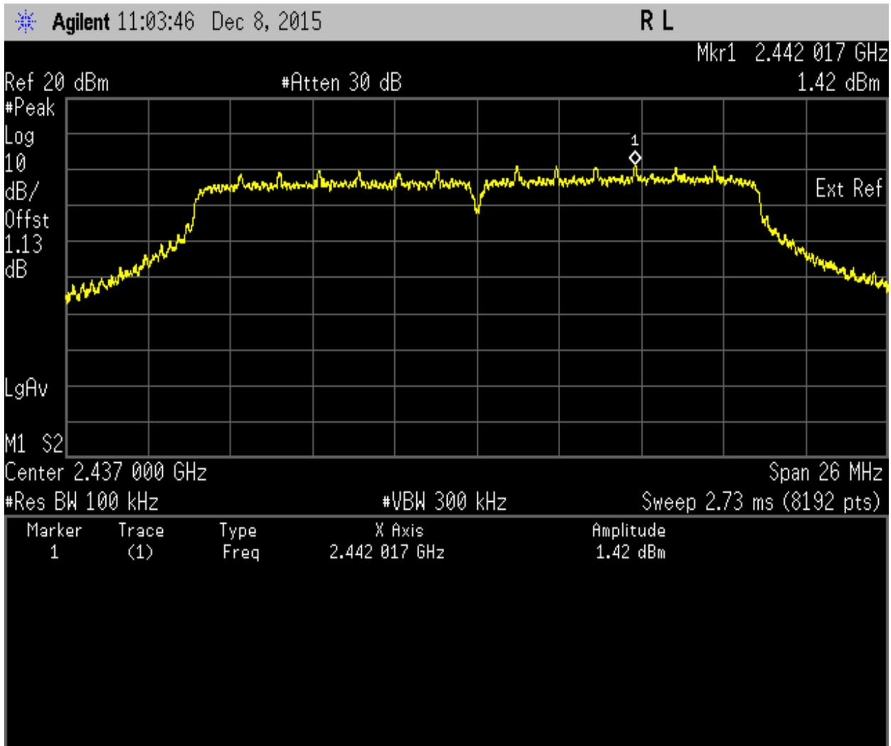
Maximum Peak Power Spectral Density. 802.11n\_20 Frequency 2437 MHz
