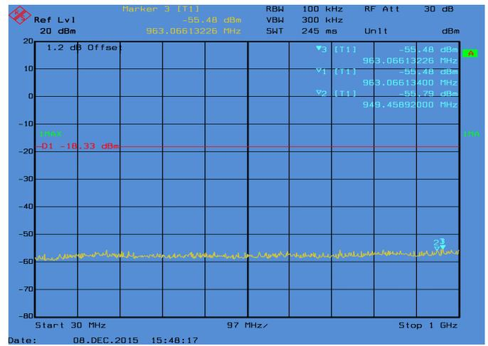
**Conducted Emissions. 802.11g, Frequency 2412 MHz Emission Level, 30 MHz -> 1 GHz**
