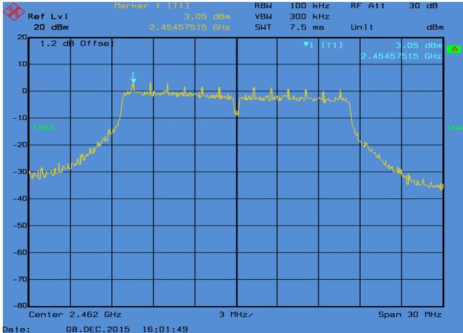
Conducted Emissions. 802.11g, Frequency 2462 MHz Reference Level
