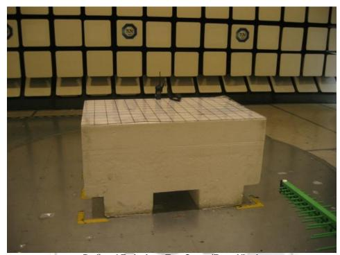
Radiated Emissions Test Setup (Front View)
