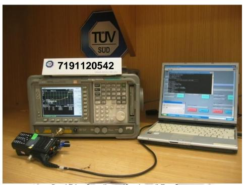
Band Edge Compliance (Conducted) Test Setup
