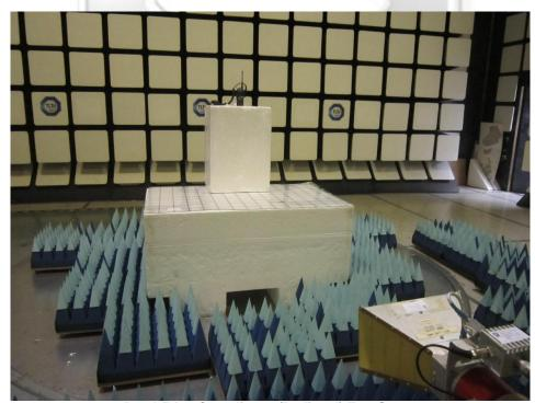
Band Edge Compliance (Radiated) Test Setup
