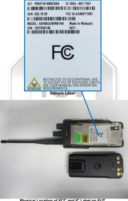
Physical Location of FCC and IC Label on EUT
