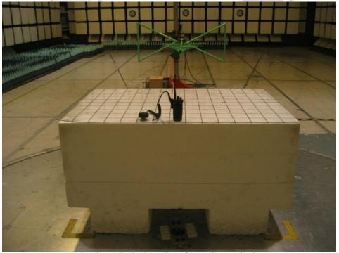
Radiated Emissions Test Setup (Rear View)
