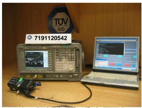
Peak Power Spectral Density Test Setup
