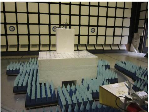
Radiated Emissions Test Setup (Front View)
