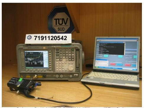
Spectrum Bandwidth (6dB Bandwidth Measurement) Test Setup
